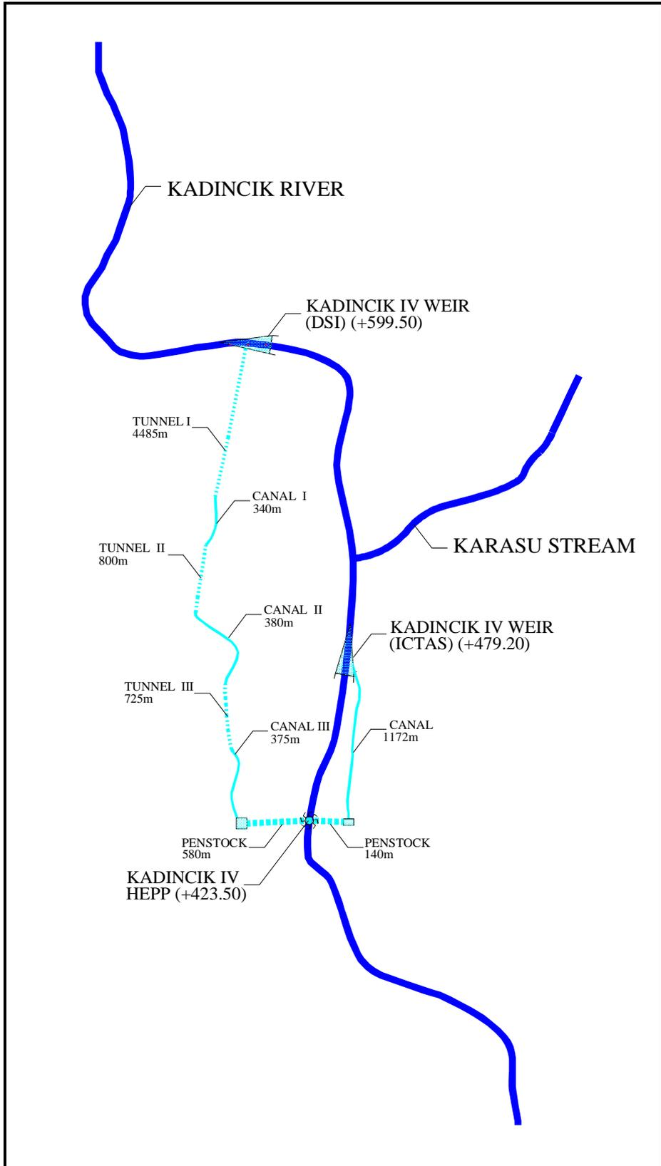
Figure 5.2. Illustration of the Two Alternatives
