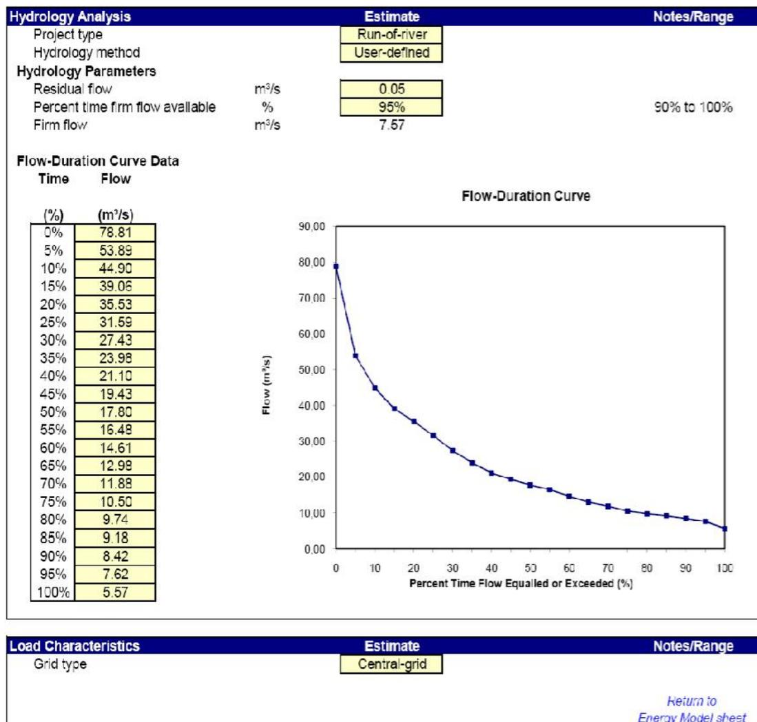
Figure 5.18. Kadıncık-4 HEPP Alternative II, Hydrology Analysis
