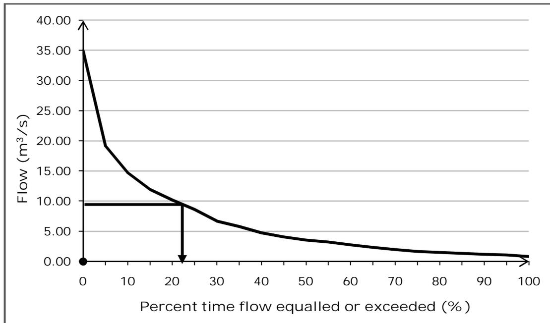
Figure 5.3. Flow-Duration Curve of Kadıncık-4 HEPP, Alternative I
