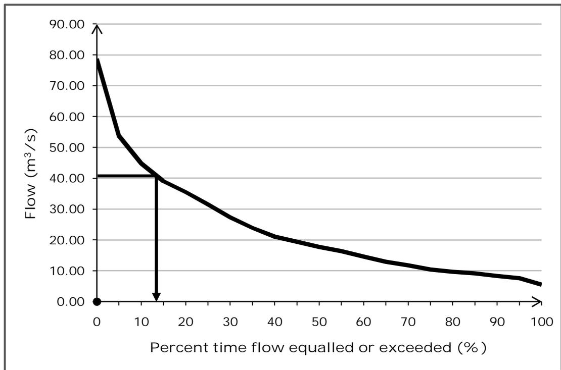
Figure 5.15. Flow-Duration Curve of Kadıncık-4 HEPP, Alternative II
