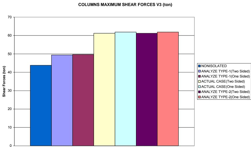
**Figure 3.24** Maximum Column Bottom Shear Forces V3 (ton) For Different Isolator Conditions.
