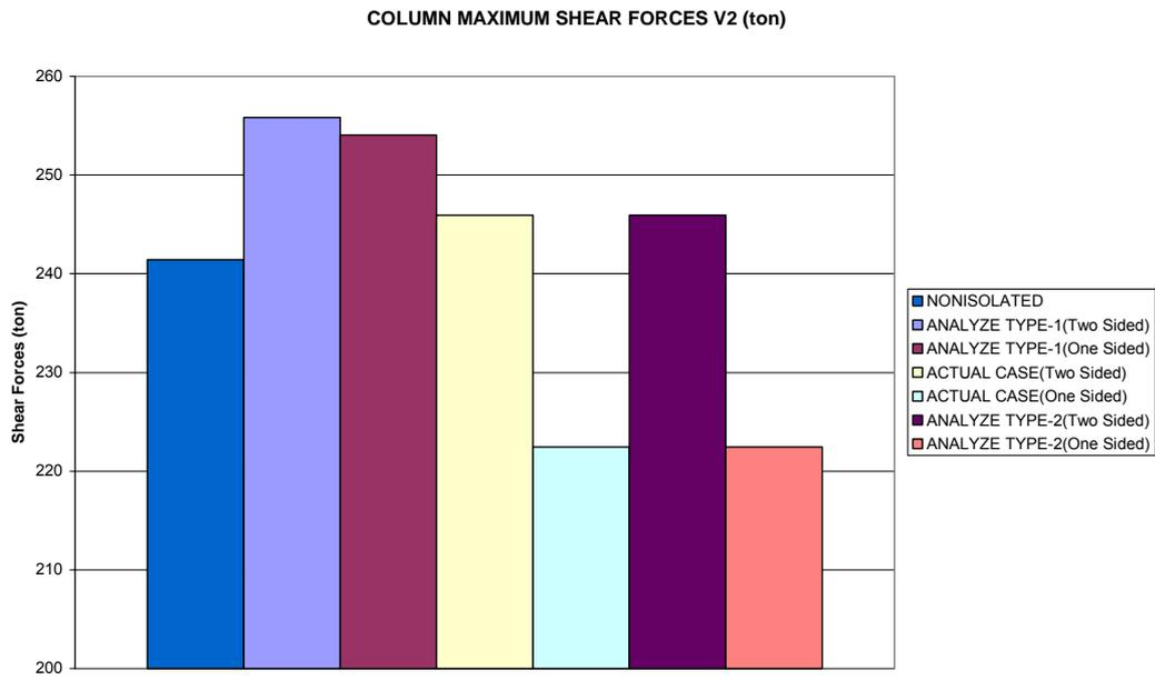
**Figure 3.23** Maximum Column Bottom Shear Forces V2 (ton) For Different Isolator Conditions.
