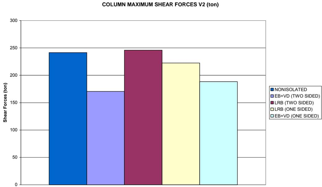
**Figure 3.6** Maximum Column Bottom Shear Forces V2 (ton) For Different Isolator Conditions.
