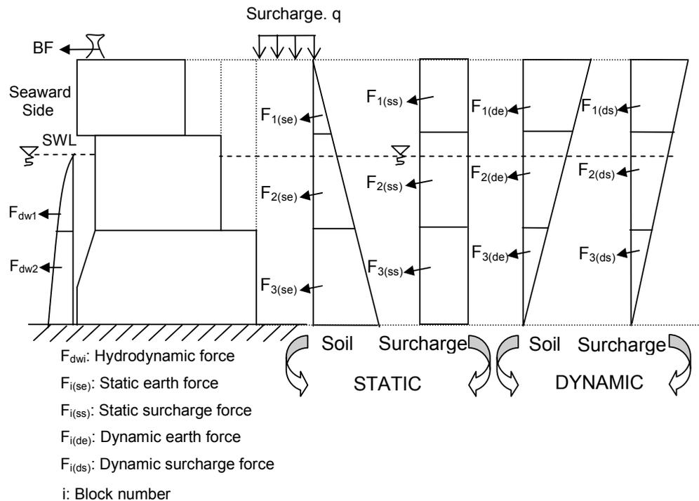
**Figure 4.13:** For dynamic case combined horizontal forces (surcharge + earth and water) and the vertical forces acting on block type quay wall
