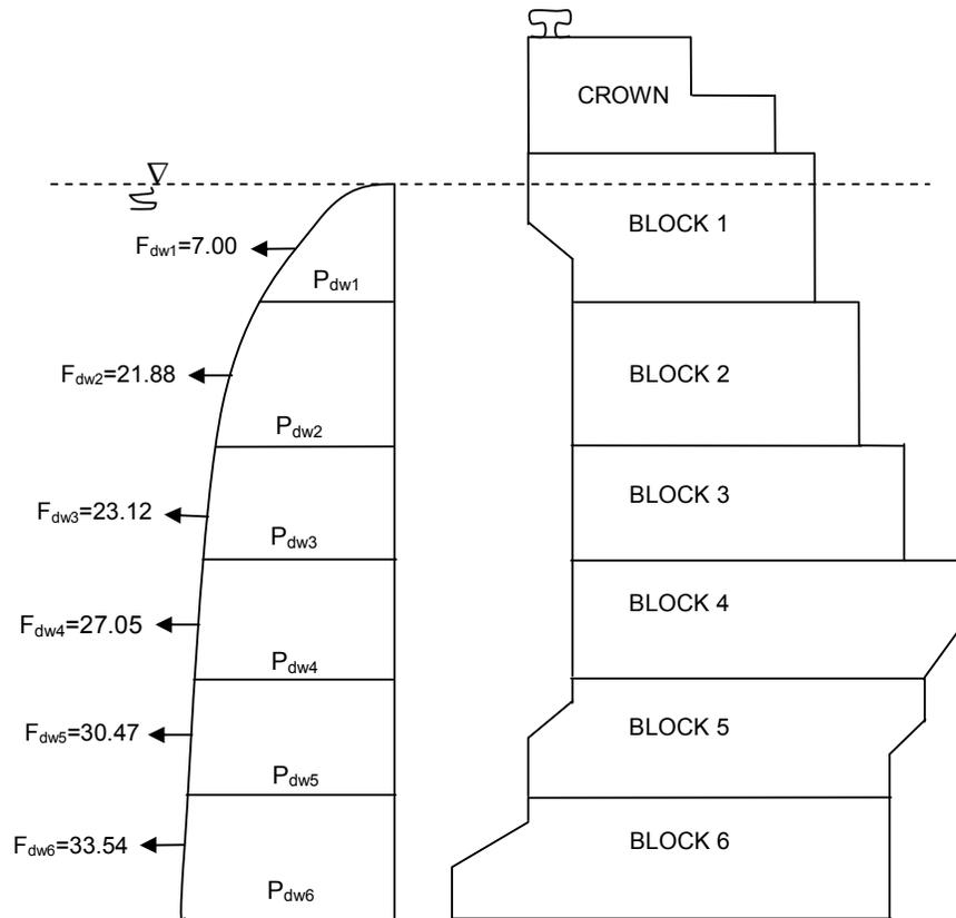
**Figure 5.7:** The hydrodynamic forces on the block type quay wall
