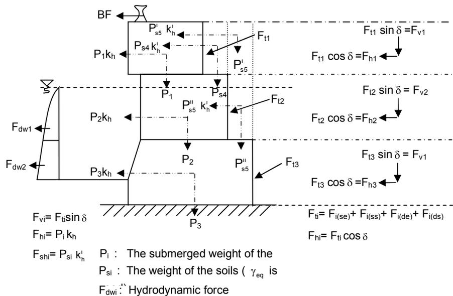
**Figure 5.8:** Forces acting on block type quay wall for Approach 1
