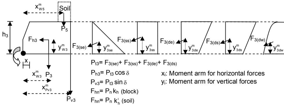
Figure 4.18: The vertical and horizontal forces on the Block 2
