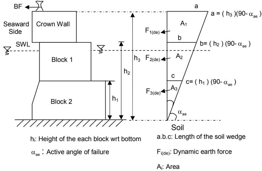
**Figure 4.10:** For dynamic case effect of soil on block type quay wall
