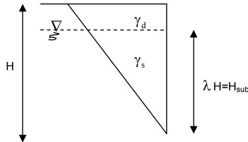
**Figure 4.9:** Calculation method of equivalent unit weight (Kramer, 1996)
