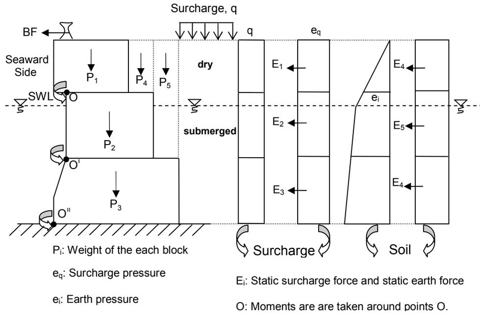
**Figure 4.4:** The static forces affecting on the block type quay walls (TSS, 1997)
