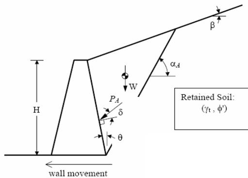
**Figure 4.7:** The parameters used to calculate active earth pressure ( $P_A$ )
