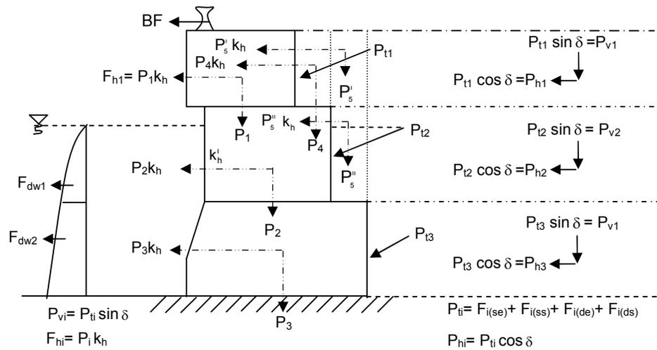
**Figure 4.15:** The vertical and horizontal forces on block type quay wall
