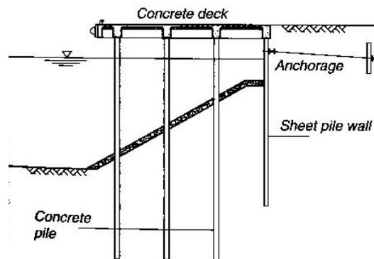
**Figure 2.11:** Typical section of open berth quay wall with retaining wall
