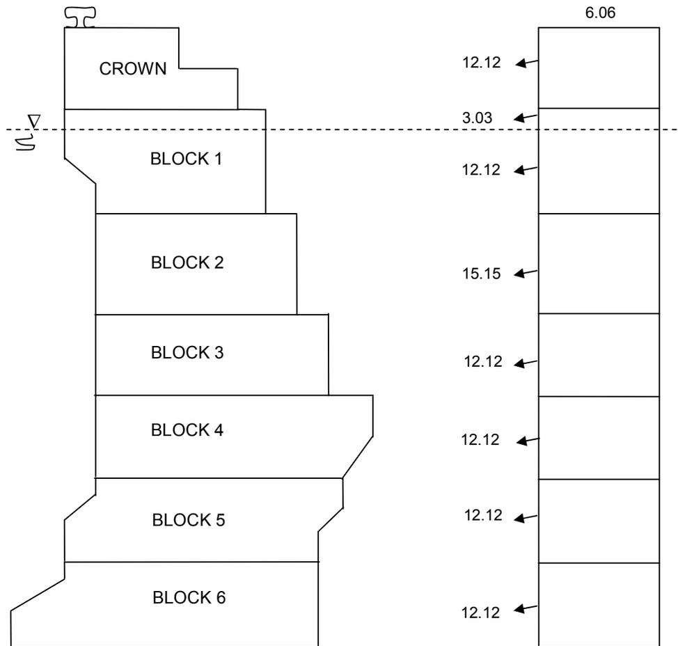
**Figure 5.13:** The surcharge effect on the block type quay wall for static case
