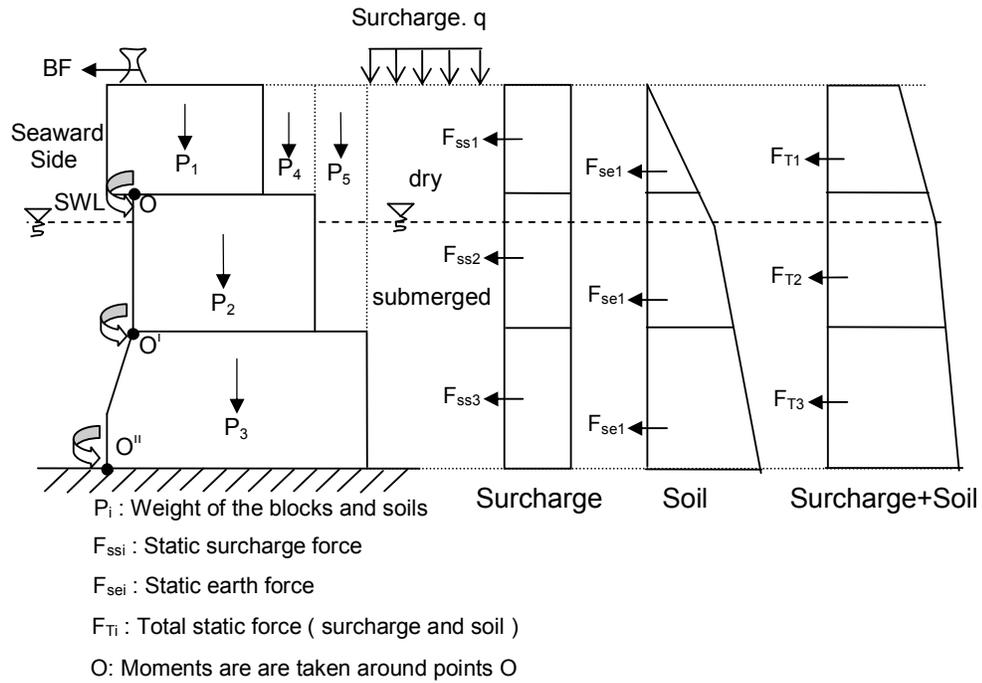
**Figure 5.18:** Static forces acting on block type quay wall (TSDC-CRA. 2007)
