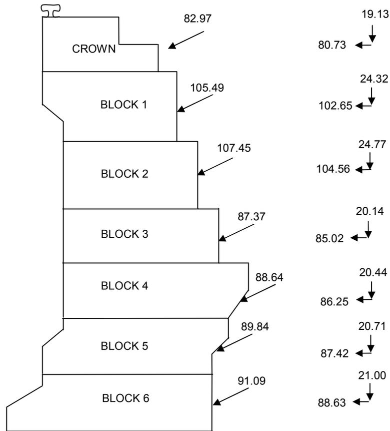
**Figure 5.6:** The total force ( static + dynamic (soil&surcharge)) on block type quay wall.
