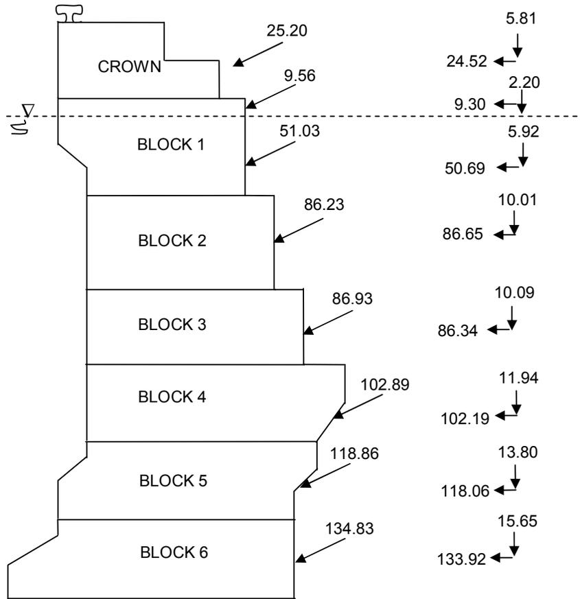
**Figure 5.16:** The total force on the block type quay wall.
