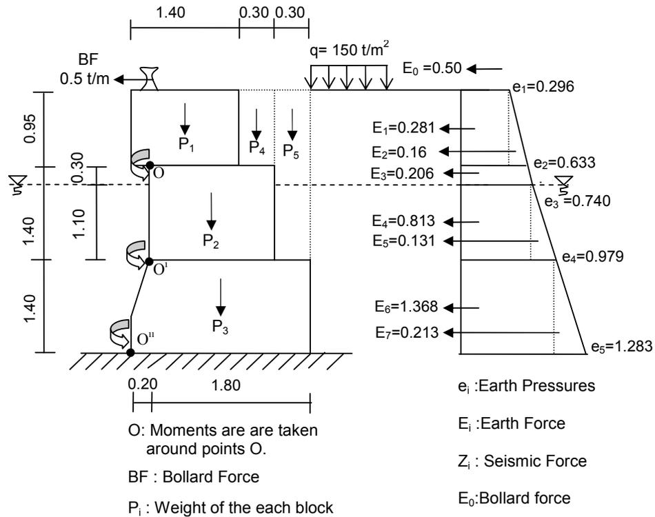
**Figure A.2:** Forces acting on block type quay wall, if earthquake is not considered (TSS, 1975)
