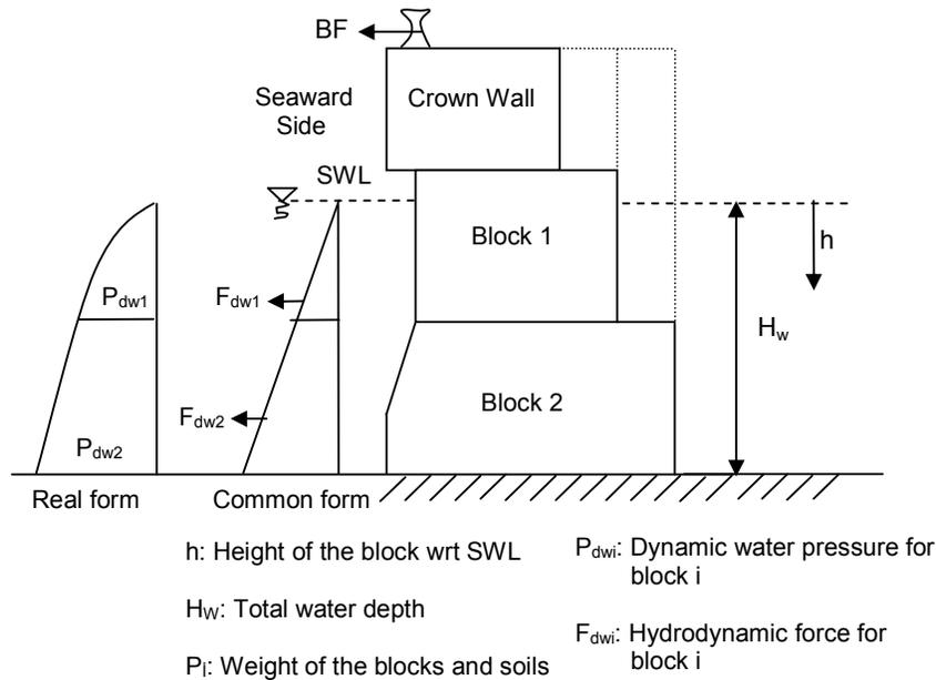
**Figure 4.12:** Earthquake-induced hydrodynamic force on coastal structure
