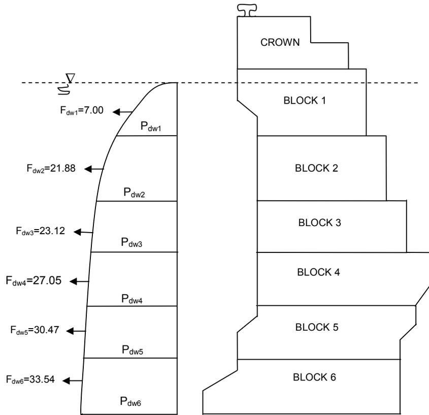
Figure 5.17: The hydrodynamic forces on the block type quay wall
