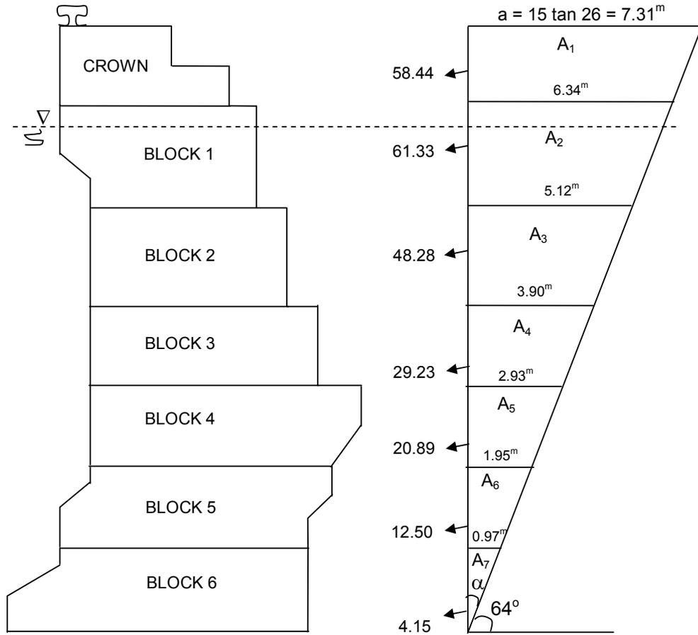
**Figure 5.4:** The soil effect on block type quay wall for dynamic case
