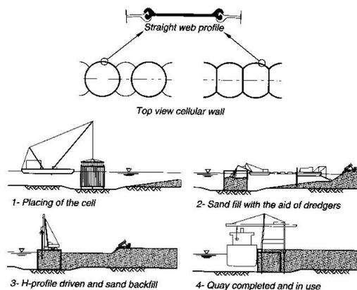
**Figure 2.6:** Typical section of cellular wall (Quay Wall Handbook, 2005)
