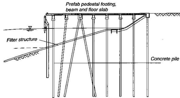
**Figure 2.12:** Typical section of open berth quay wall with embankment (Quay Wall Handbook, 2005)
