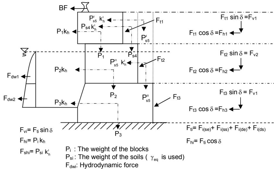
**Figure 5.9:** Forces acting on block type quay wall for Approach 2
