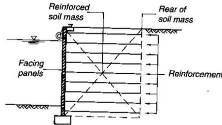
**Figure 2.7:** Typical section of reinforced earth wall (Quay Wall Handbook, 2005)
