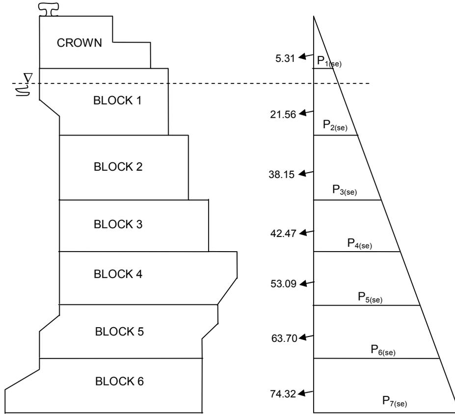
**Figure 5.2:** The soil effect on block type quay wall for static case
