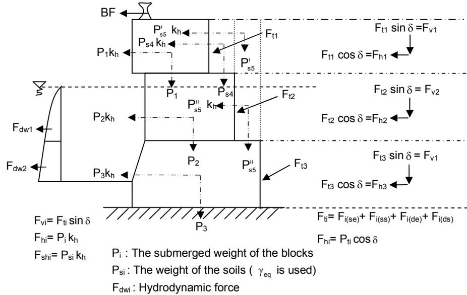
**Figure 5.10:** Forces acting on block type quay wall for Approach 3
