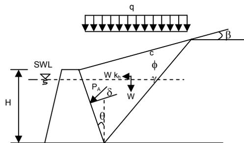
**Figure 4.6:** All the parameters used for calculating the forces
