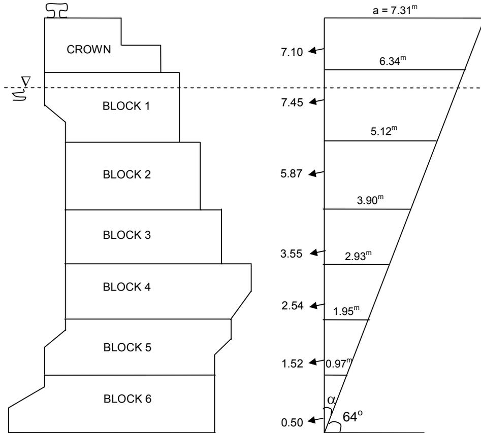
**Figure 5.5:** The surcharge effect on block type quay wall for dynamic case
