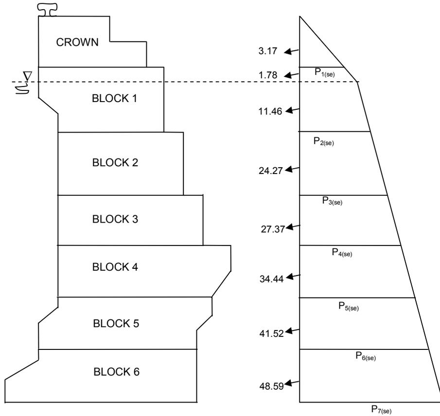
**Figure 5.14:** The soil effect on the block type quay wall for dynamic case
