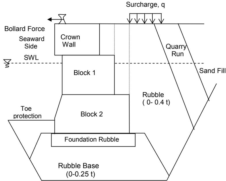
**Figure 4.1:** Typical section of block type quay wall
