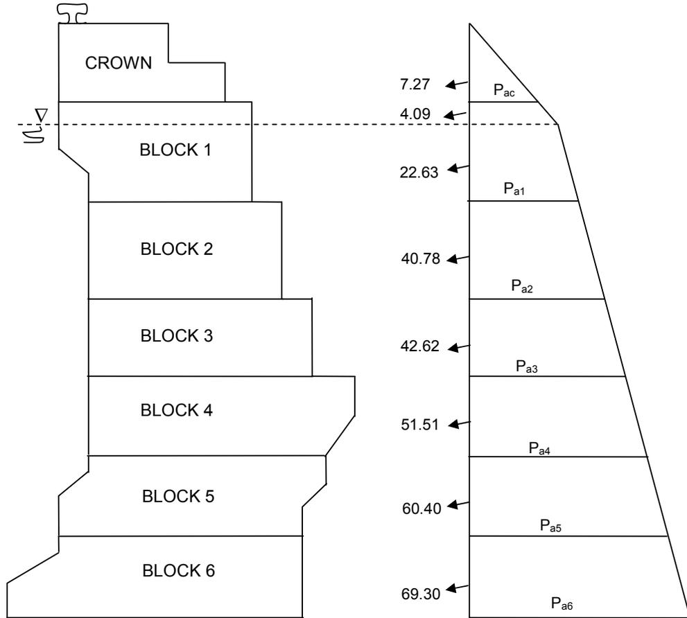
**Figure 5.12:** The soil effect on the block type quay wall for static case
