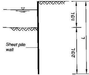
**Figure 2.8:** Typical section of cantilever wall (Quay Wall Handbook, 2005)
