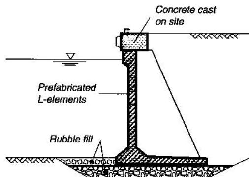
**Figure 2.4:** Typical section of L wall (Quay Wall Handbook, 2005)
