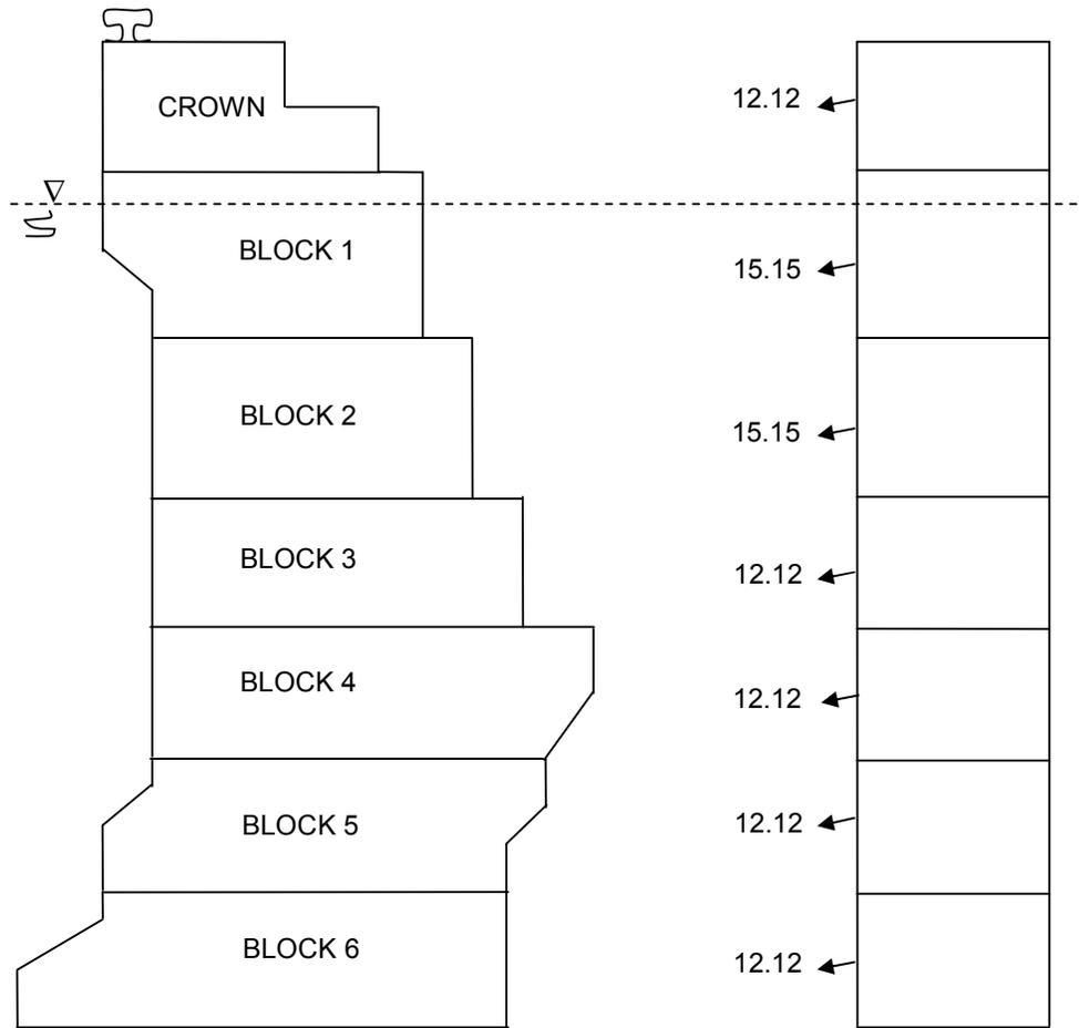
**Figure 5.3:** The surcharge effect on block type quay wall for static case
