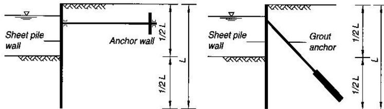
**Figure 2.9:** Typical section of anchored wall (Quay Wall Handbook, 2005)
