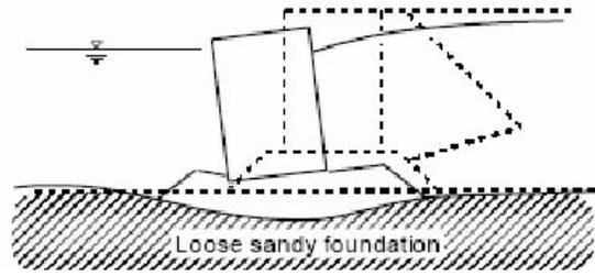
**Figure 2.14:** Deformation/failure modes of gravity quay wall on loose sandy formation (PIANC, 2001)
