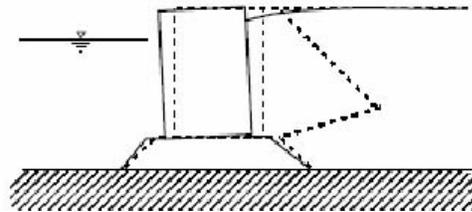
**Figure 2.13:** Deformation/failure modes of gravity quay wall on firm foundation (PIANC, 2001)
