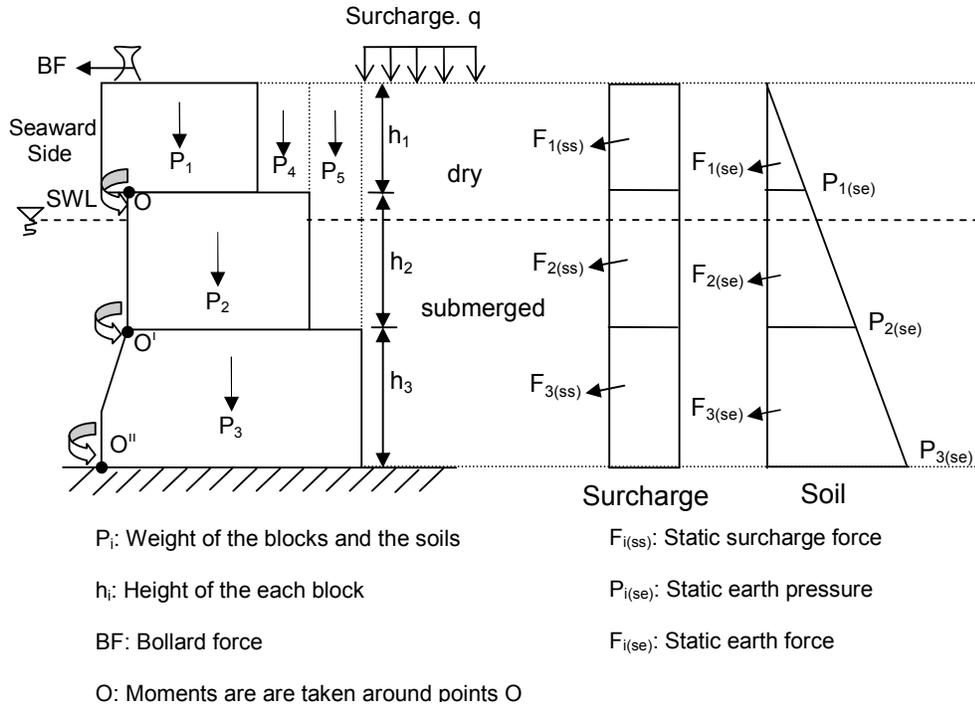
**Figure 4.8:** Forces acting on block type quay wall in static condition
