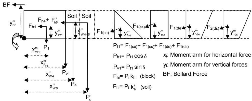
**Figure 4.16:** The vertical and horizontal forces on crown wall
