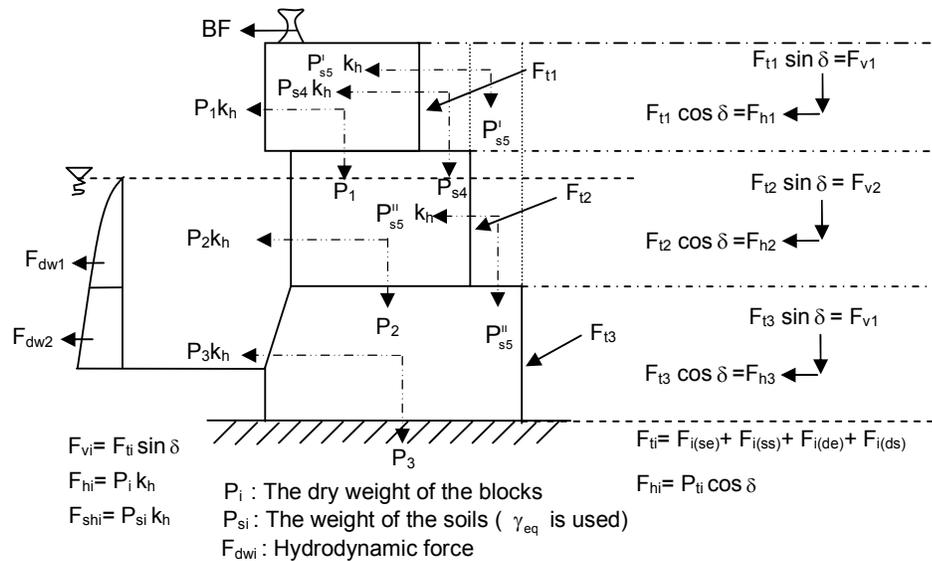
**Figure 5.11:** Forces acting on block type quay wall for Approach 4
