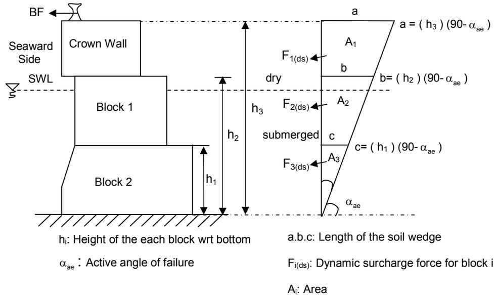
**Figure 4.11:** The dynamic effect of surcharge on block type quay wall
