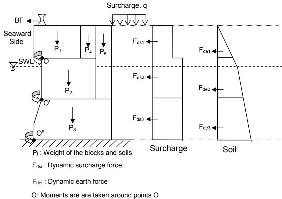
**Figure 5.19:** Dynamic forces acting on block type quay wall
