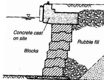
**Figure 2.3:** Typical section of block type wall (Quay Wall Handbook, 2005)
