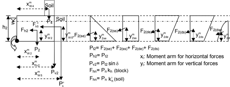
**Figure 4.17: The vertical and horizontal forces on the Block 1**
