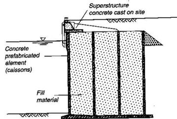
**Figure 2.5:** Typical section of caisson wall (Quay Wall Handbook, 2005)
