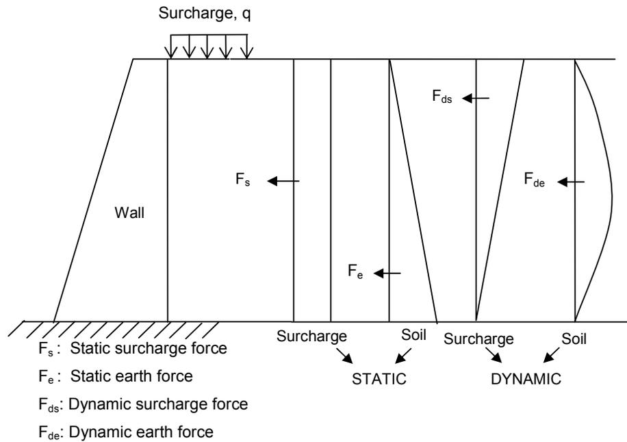
**Figure 4.3:** Forces both static and dynamic cases acting on a vertical wall
