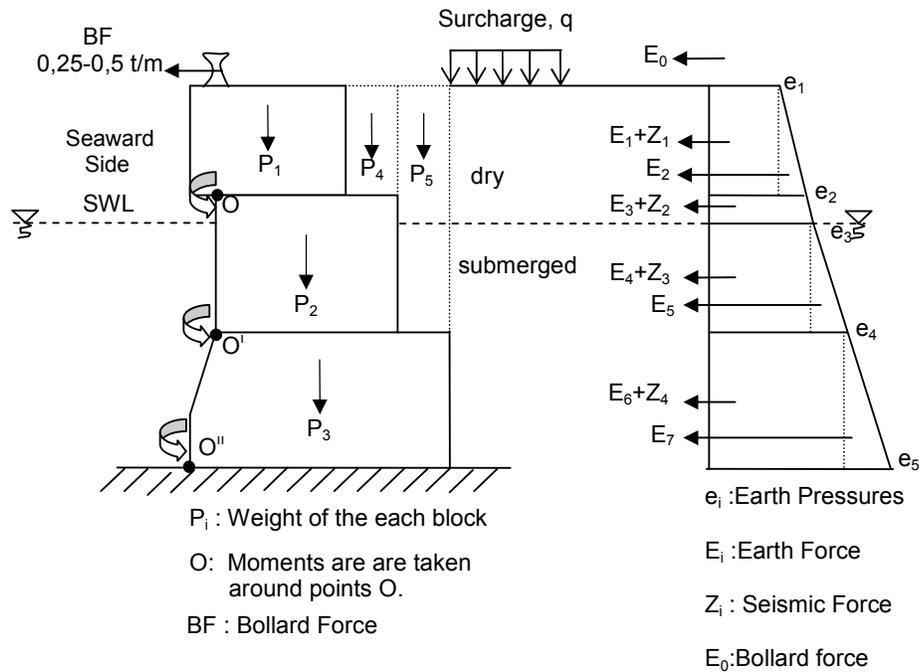
**Figure 4.2:** Loads both static and dynamic acting on block type quay walls according to TSS, 1975
