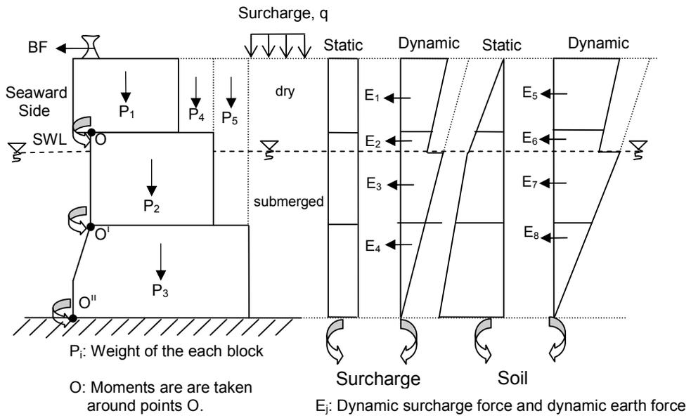
**Figure 4.5:** The dynamic forces affecting on the block type quay walls (TSS, 1997)
