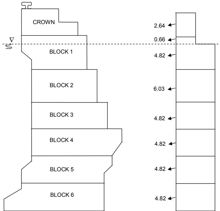
**Figure 5.15:** The surcharge effect on the block type quay wall for dynamic case
