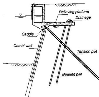
**Figure 2.10:** Typical section of embedded wall (Quay Wall Handbook, 2005)
