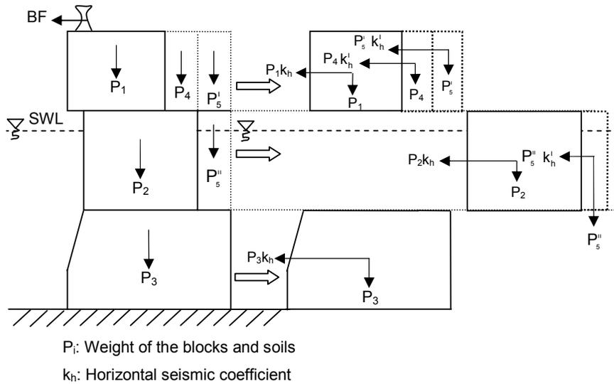
**Figure 4.14:** Inertia forces acting on block type quay wall
