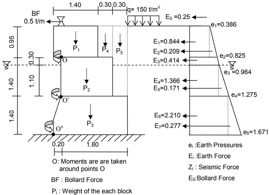
**Figure A.3:** Forces acting on block type quay wall. if earthquake is considered.
