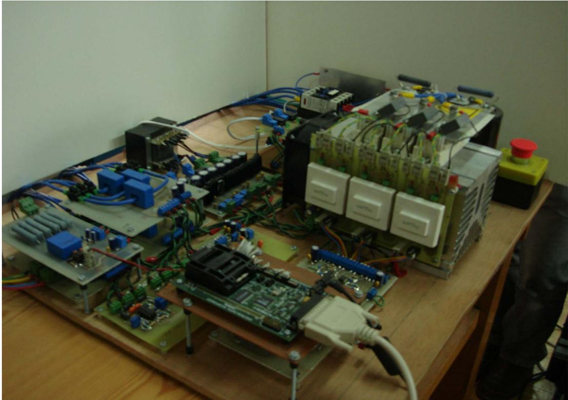
Figure 6.4 Laboratory prototype of the 3-phase 3-wire PAF (side view).
