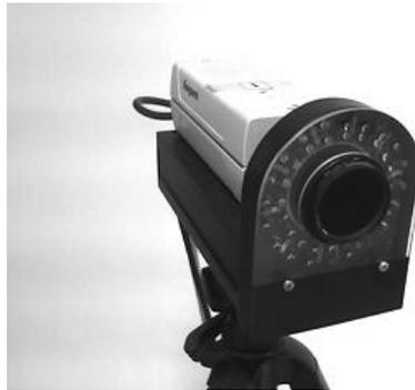
Figure 3.2 Camera with Infrared LED's and Filter
