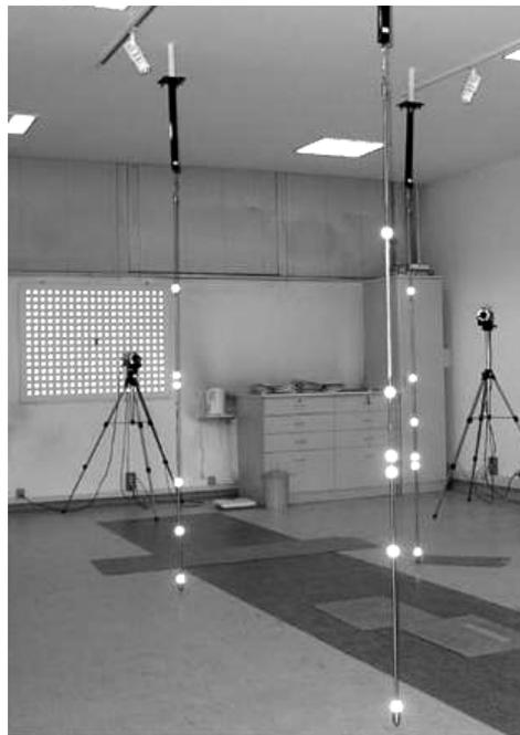
Figure 3.4 Calibration Rods (Front) and Linearization Grid (Back)
