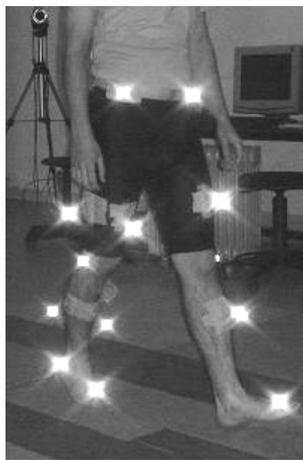
Figure 5.3 Dynamic Trial with Front and Side Markers
