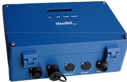
Figure 5.1: GSR-16 accelerometer with a dynamic range of 72/96 dB,  $SNR > 102\text{dB}$  (Geosig, 2007)
