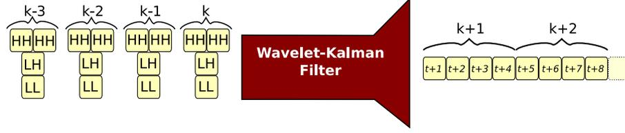
Figure 4.1: Wavelet-Kalman filter in action. The left hand side of the figure shows the block level filtered wavelet transform of the signal, the right hand side shows the continuous feeding of the filter by measurement blocks.
