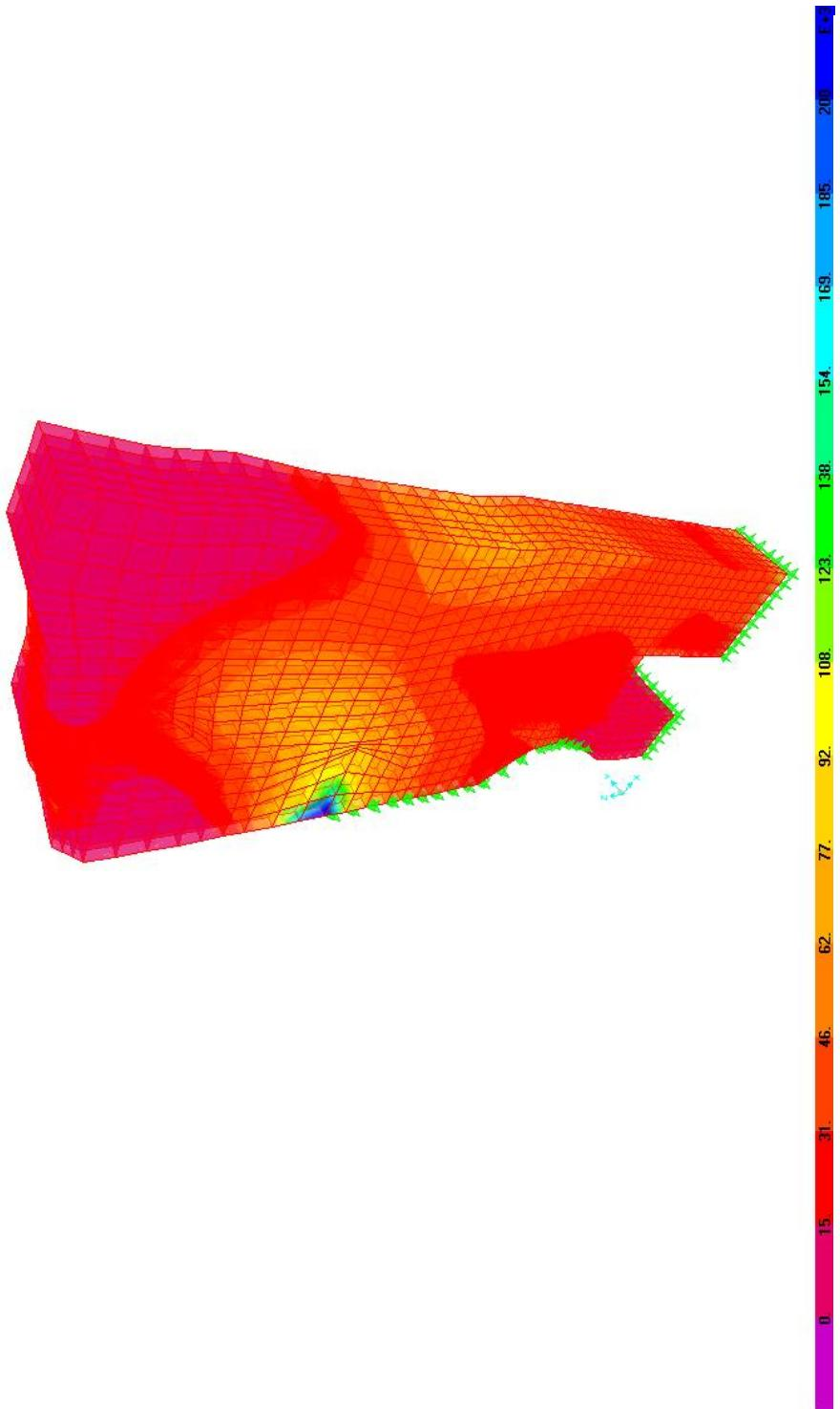
Figure 4.29 The diagram for the positive stress distribution for Load Case-2. The contours are scaled such that the blue contours show the locations where the stress is greater than 0.2 MPa.
