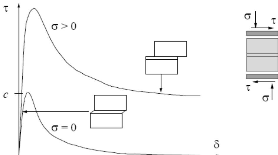
**Figure 2. 22 Behavior of masonry under shear direct shear [6].**
