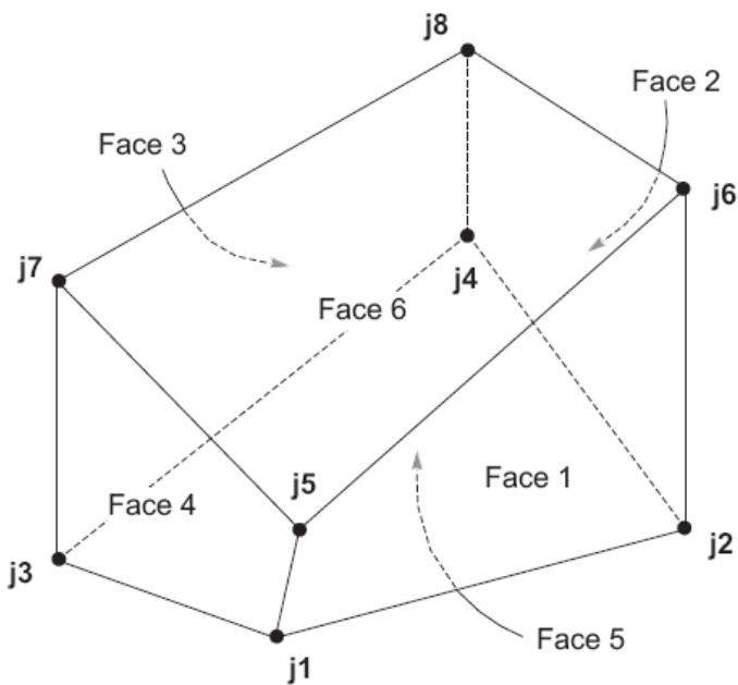
Figure 4.2 Solid element joint connectivity and face definitions of SAP2000.
