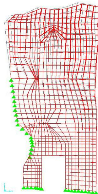
**Figure 4.28 X component of displacement at ultimate load for Load Case-2 (linear analysis).**
