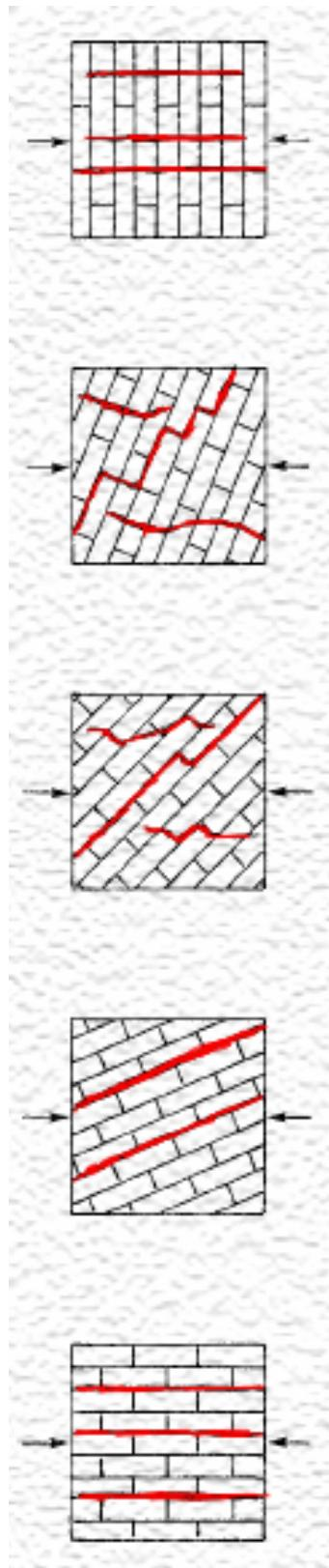
**Figure 3.9** Crack patterns of masonry under biaxial compression.
