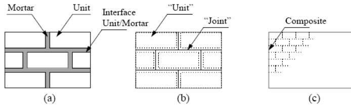
**Figure 3.19 Modeling strategies for masonry structures, a) detailed micro-modeling b) simplified micro-modeling c) macro-modeling [6].**
