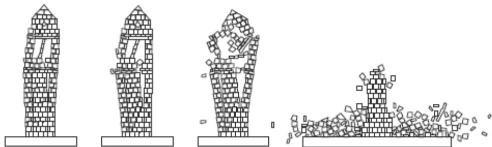
**Figure 3.18 Collapse sequence of a masonry tower [5].**
