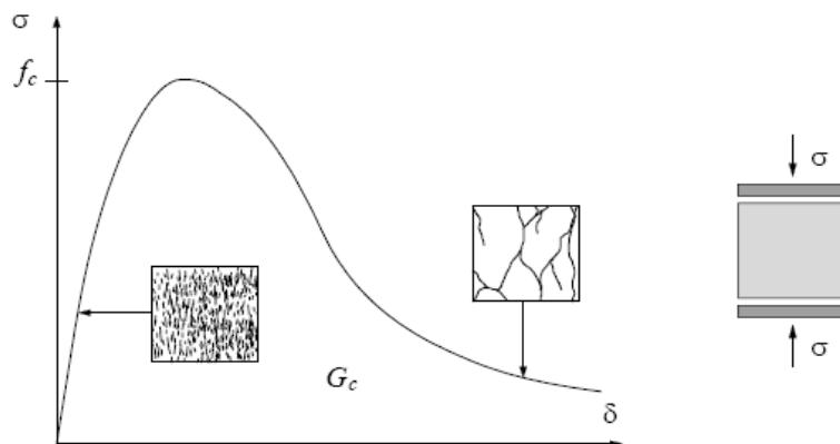
**Figure 2. 17 Typical behavior of quasi-brittle materials under uniaxial compression [6].**
