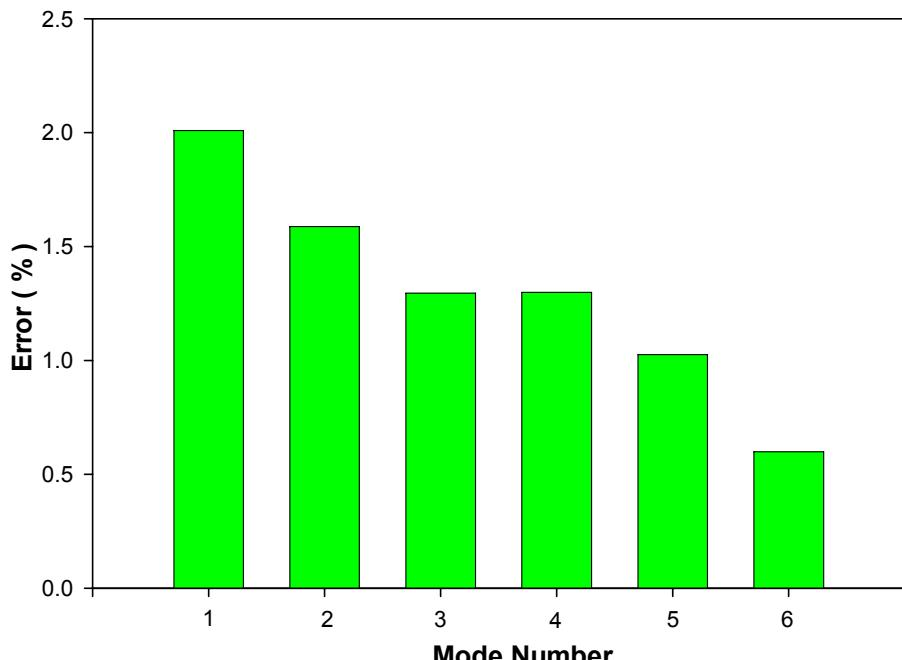
**Figure 4.11 Vertical bar chart of the percentage error for modal periods assuming ANSYS as the reference**
