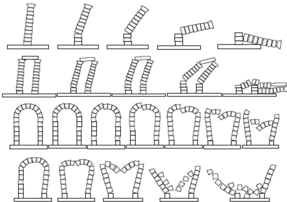
**Figure 3.15 Seismic behavior and collapse patterns for different structural elements [5].**
