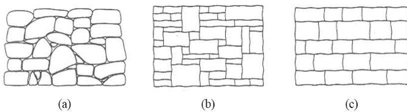
**Figure 2. 1 Different kinds of stone masonry; a) rubble masonry b) ashlar masonry c) coursing ashlar masonry [6]**
