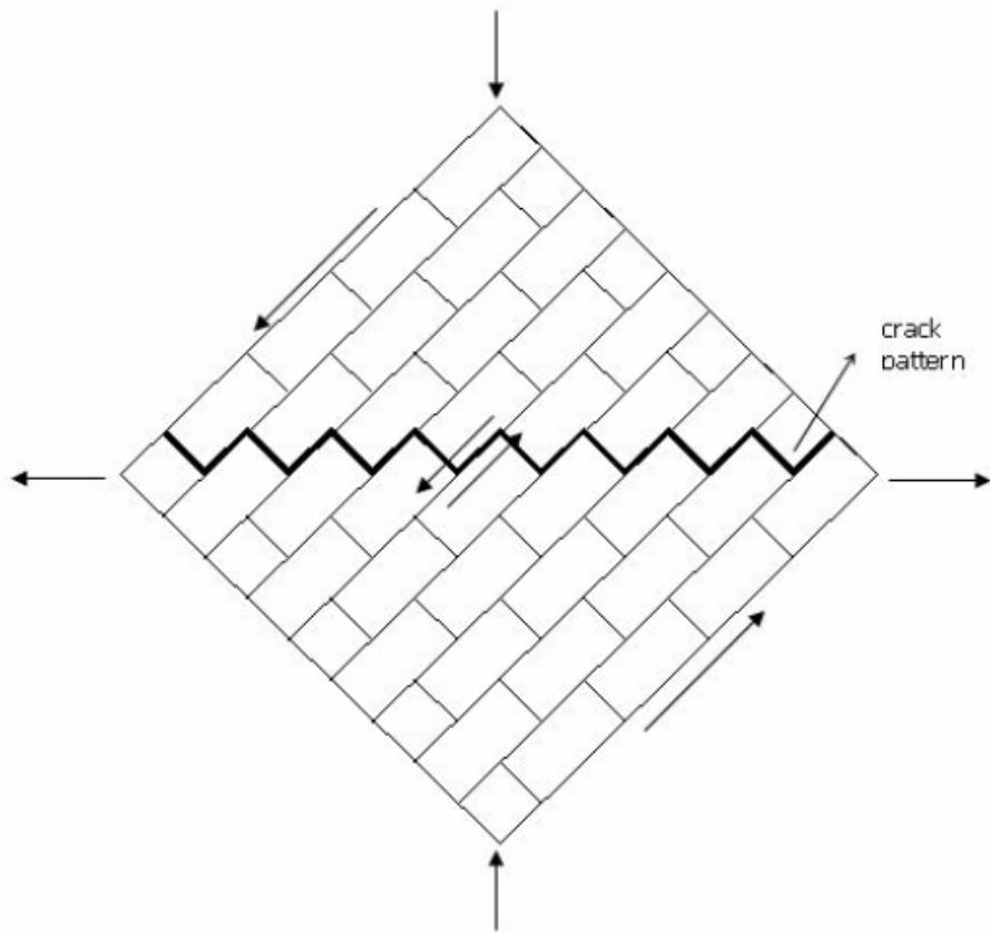
**Figure 3.8 Stepwise failure along diagonal [2].**
