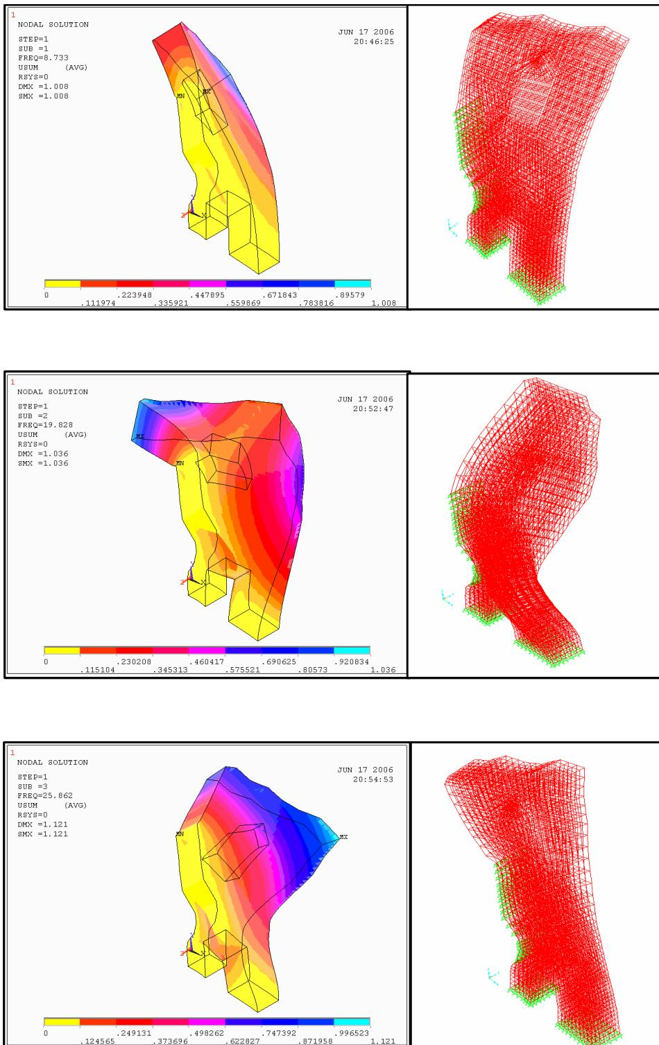
**Figure 4.8 Modal deformed shapes for Modes 1,2 and 3, respectively.**
