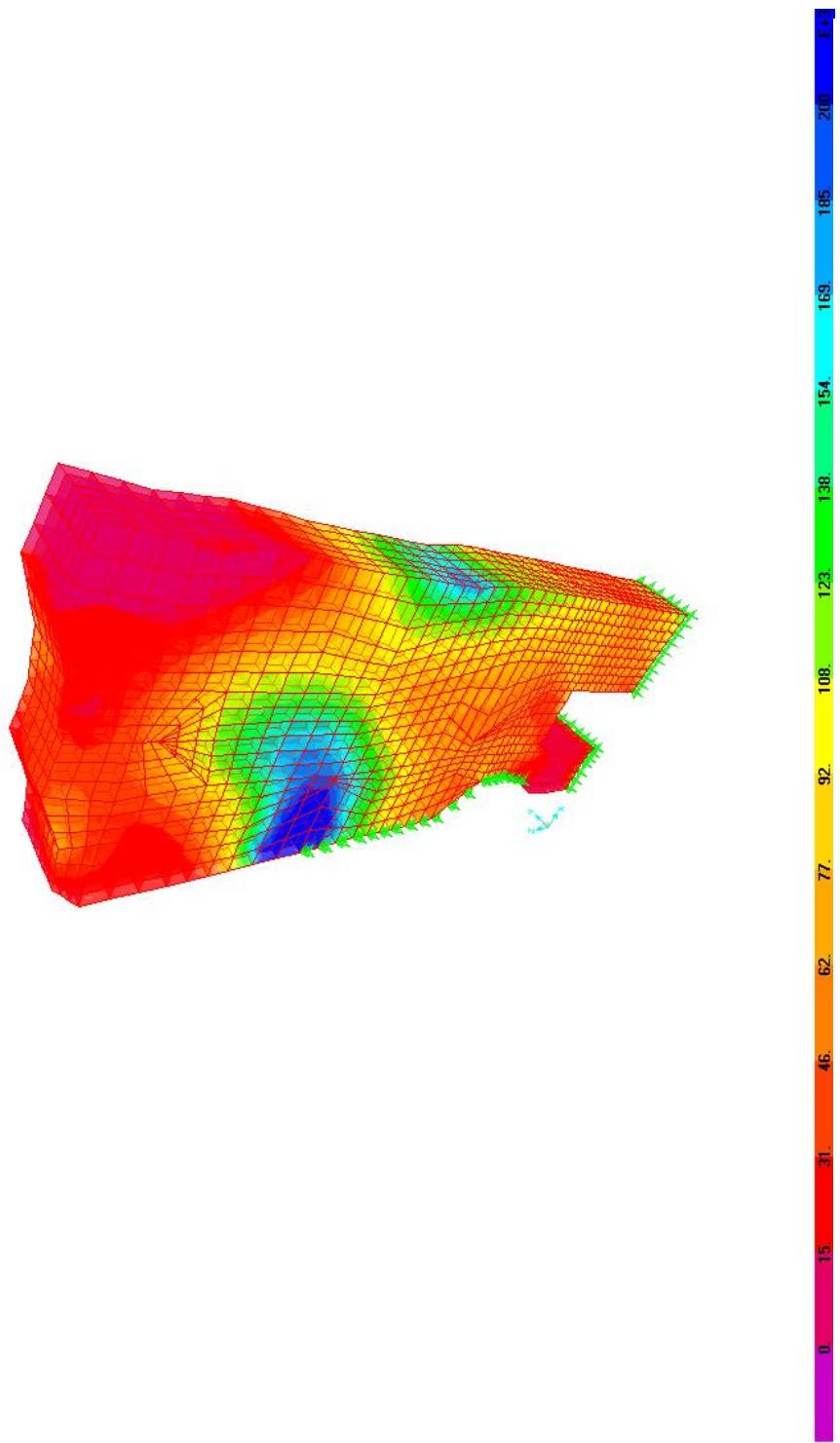
Figure 4.22 The diagram for the positive stress distribution for Load Case-1. The contours are scaled such that the blue contours show the locations where the stress is greater than 0.2 MPa.
