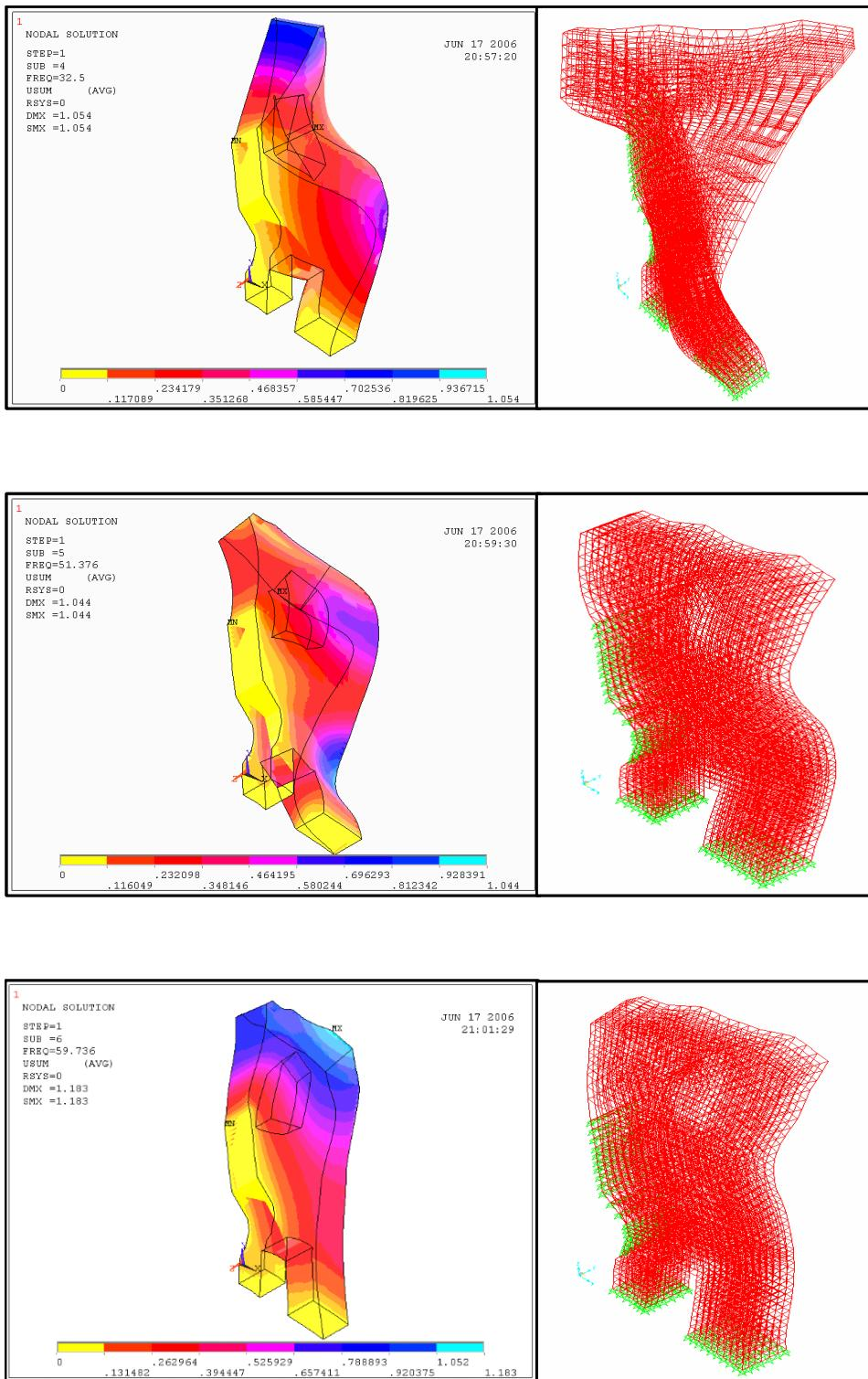
Figure 4.9 Modal deformed shapes for Modes 4,5 and 6, respectively.
