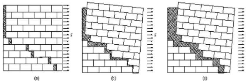
**Figure 3.16 Collapse mechanisms of a panel wall under horizontal loading, a) sliding b) overturning c) mixed mode [31].**
