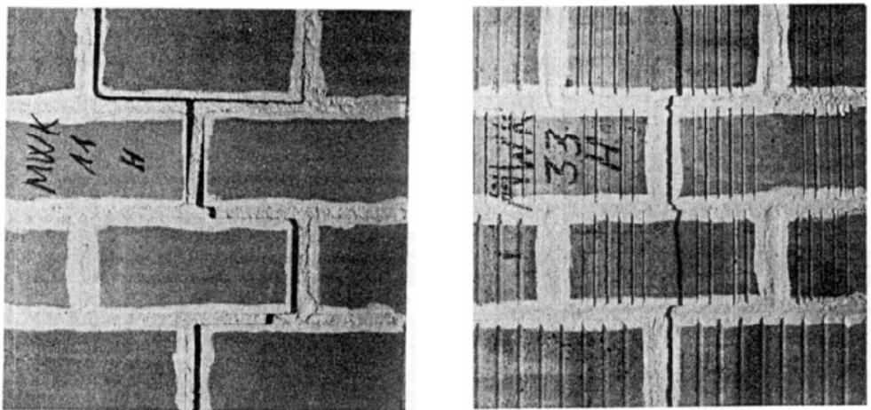
**Figure 3.6 Stepped crack and vertical crack photos of the specimens under tensional loading [6].**
