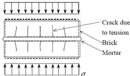
**Figure 3.3 Sketch of the splitting failure mechanism [20].**
