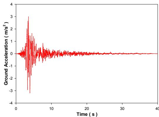
**Figure 4.12 Acceleration trace of one horizontal component of the 1989 Loma Prieta Earthquake recorded at Gilroy Gavilan College applied to the base of the structure ( PGA=3.19m/s<sup>2</sup> ).**
