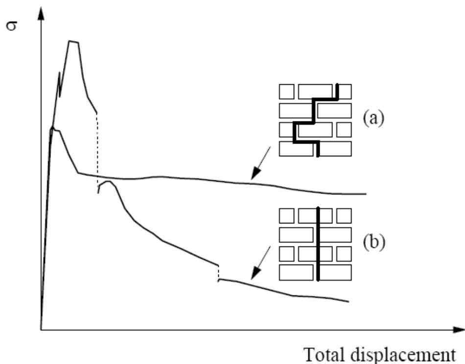
**Figure 3.5 Stress-displacement diagrams for tension in the direction parallel to bed joints, a) a stepped crack through head and bed joints b) vertical crack through head joints and units [6].**
