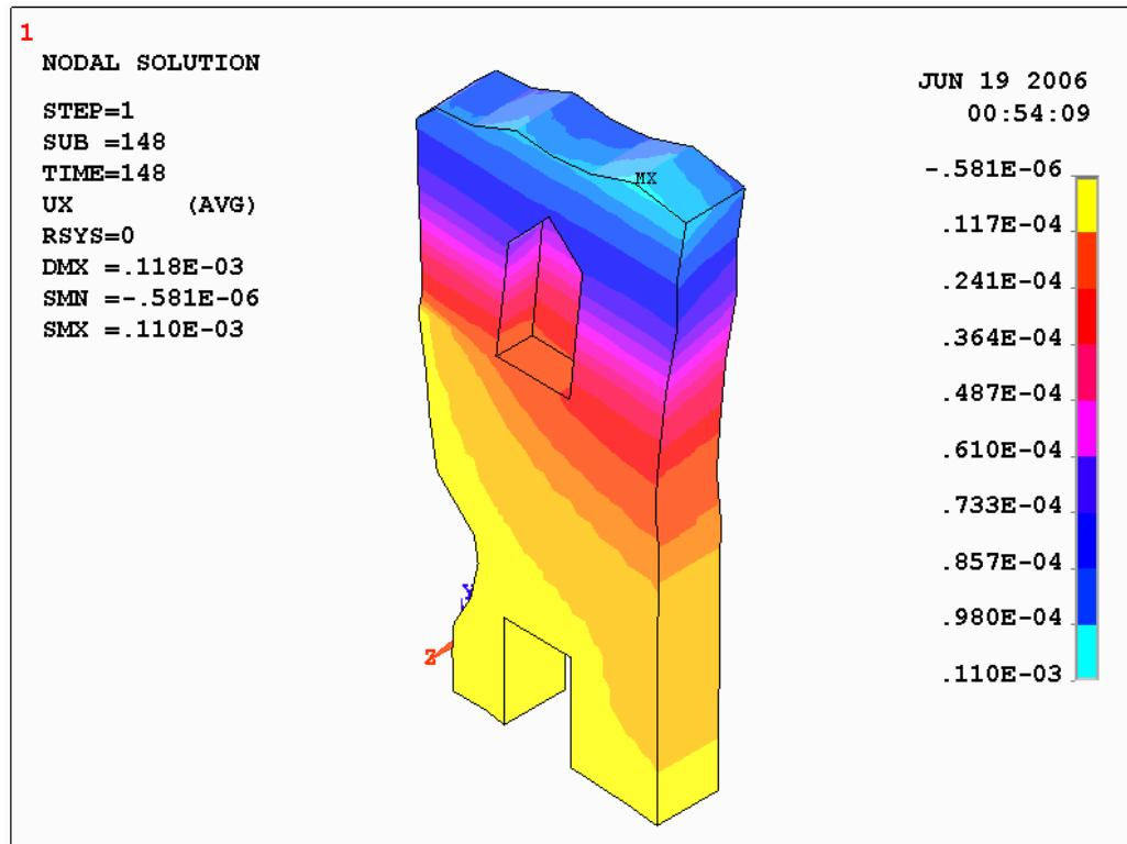
**Figure 4.27 X component of displacement at ultimate load for Load Case-2 (non-linear analysis).**
