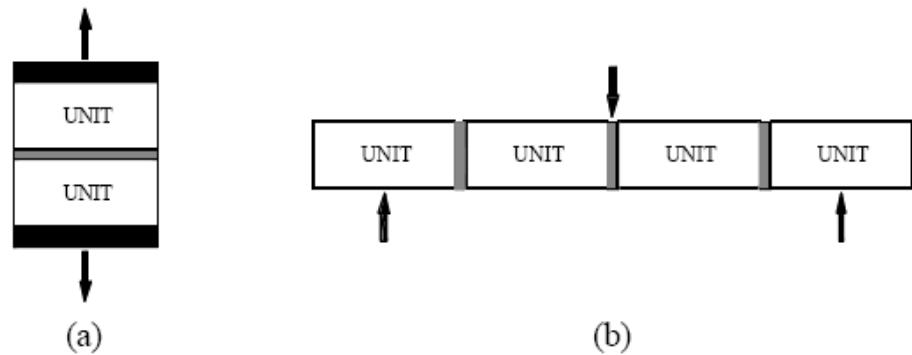
**Figure 2. 20 Direct tensile bind strength and flexural bind strength tests [7].**
