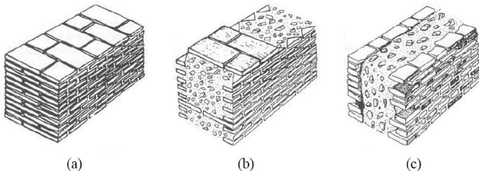
**Figure 2. 7 Roman masonry walls; a) bonded brick wall b) brick faced wall with header courses c) brick faced wall [7]**
