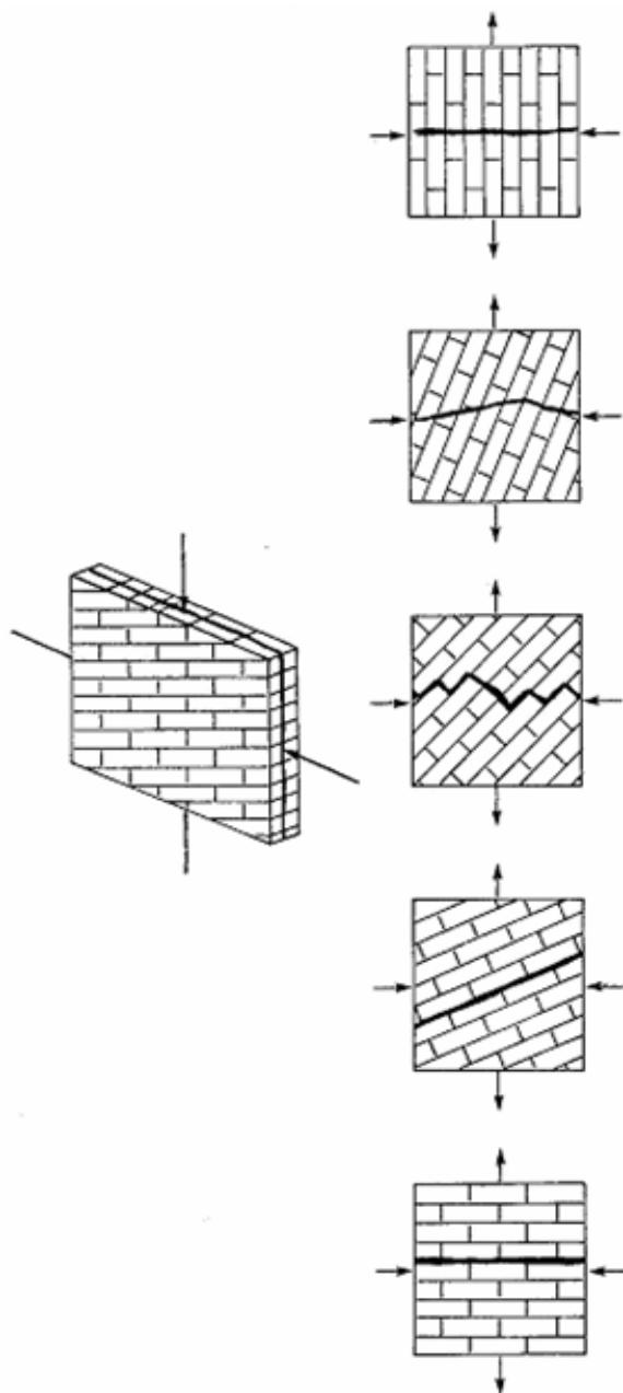
**Figure 3.11** Crack patterns in biaxial stress states for masonry.
