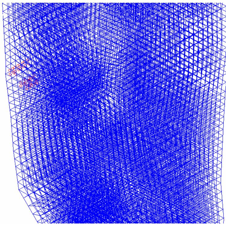
**Figure 4.32** Crack pattern at ultimate load for Load Case-3.
