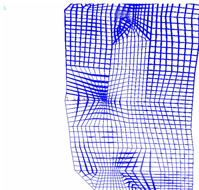
**Figure 4.25** Crack pattern at ultimate load for Load Case-2.
