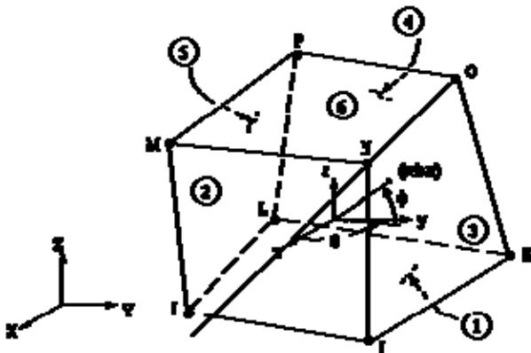
**Figure 4.3 The node locations, geometry and coordinate system of SOLID65 element.**
