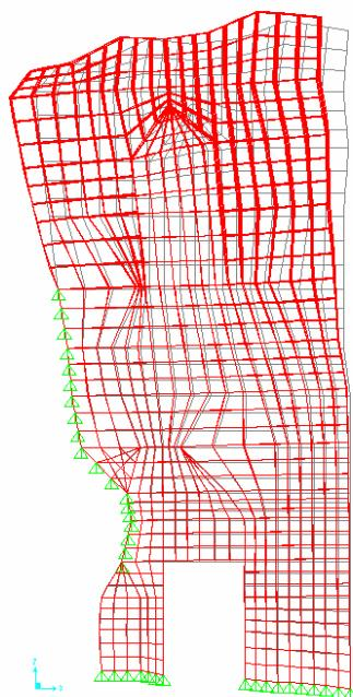
Figure 4.21 X component of displacement at ultimate load for Load Case-1 (linear analysis).
