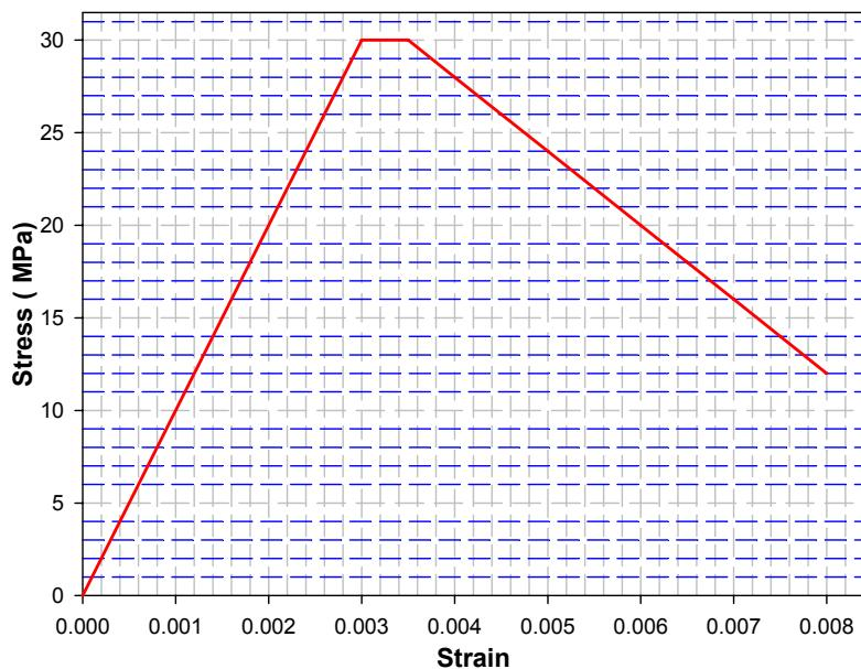
**Figure 4.4 Stress-strain relation for the macro element model**
