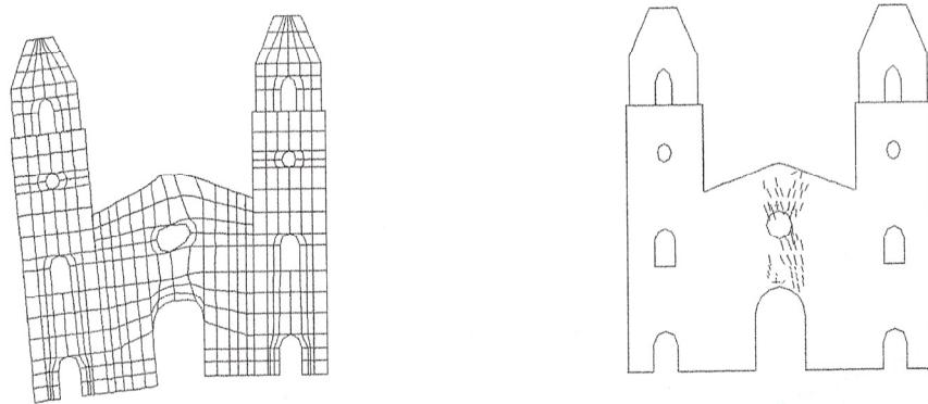
**Figure 3.12 Deformed shape and cracks of a masonry church due to support settlement [28].**
