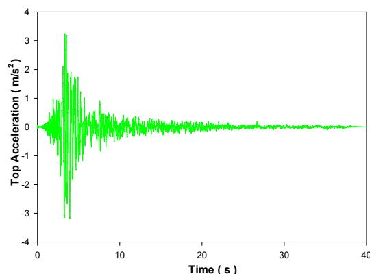
**Figure 4.13 Acceleration trace observed at the top of the structure ( Max Acc.=3.22m/s<sup>2</sup> ).**
