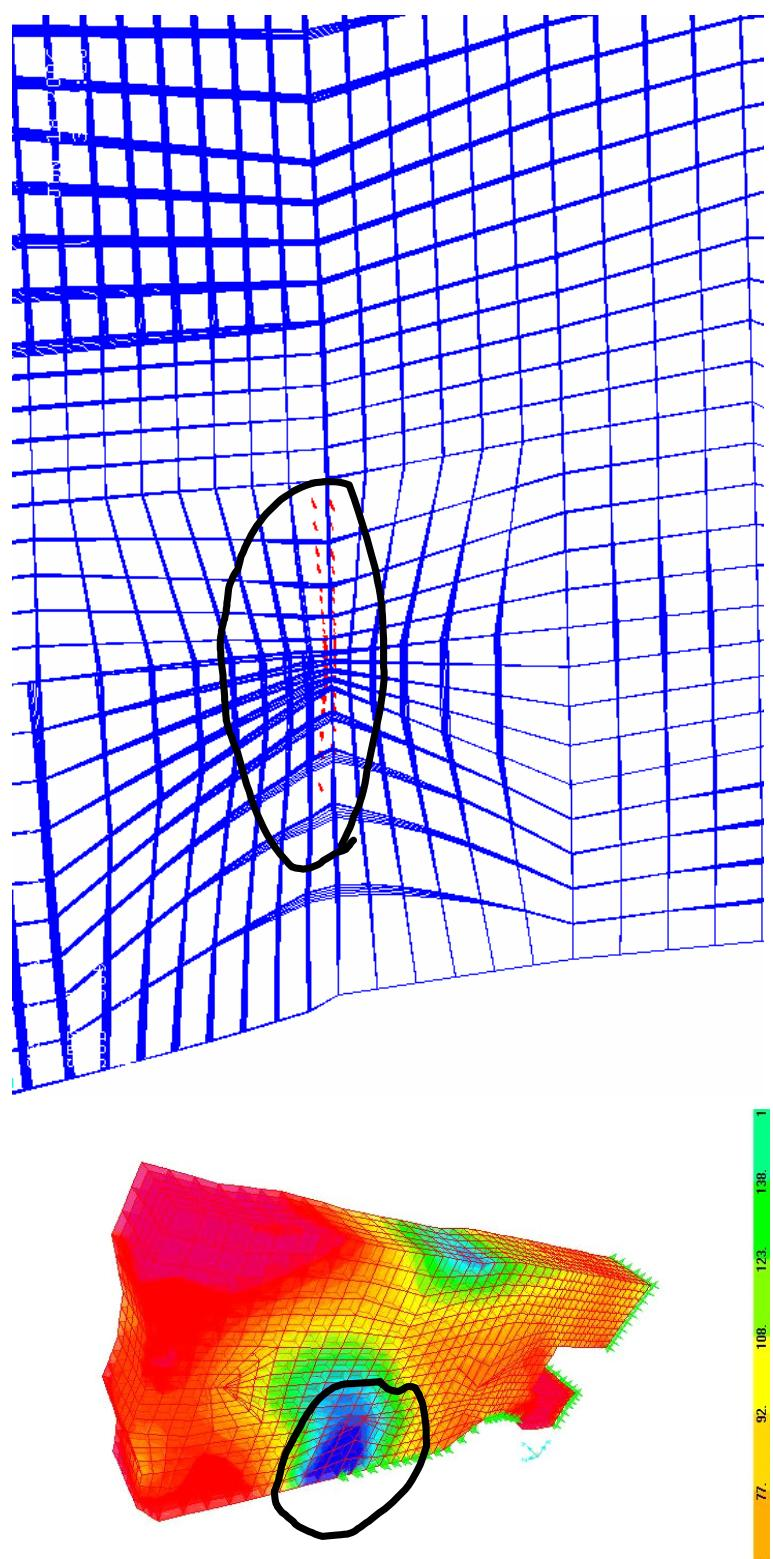
Figure 4.23 The comparison of the crack locations for linear and non-linear analysis for Load Case-1.
