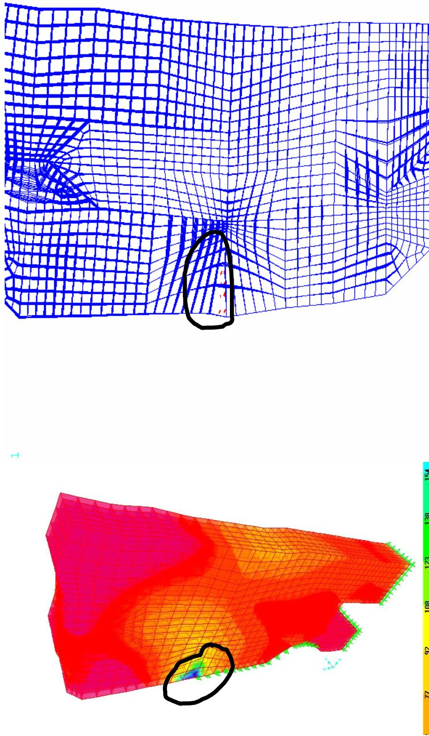
Figure 4.30 The comparison of the crack locations for linear and non-linear analysis for Load Case-2.
