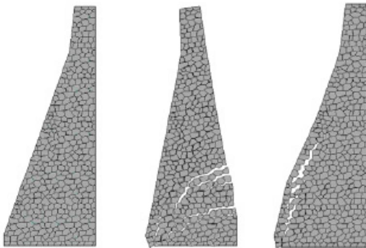
**Figure 3.14** The undeformed shape and expected failure mechanism of a load bearing wallof a Portuguese Castle [29].
