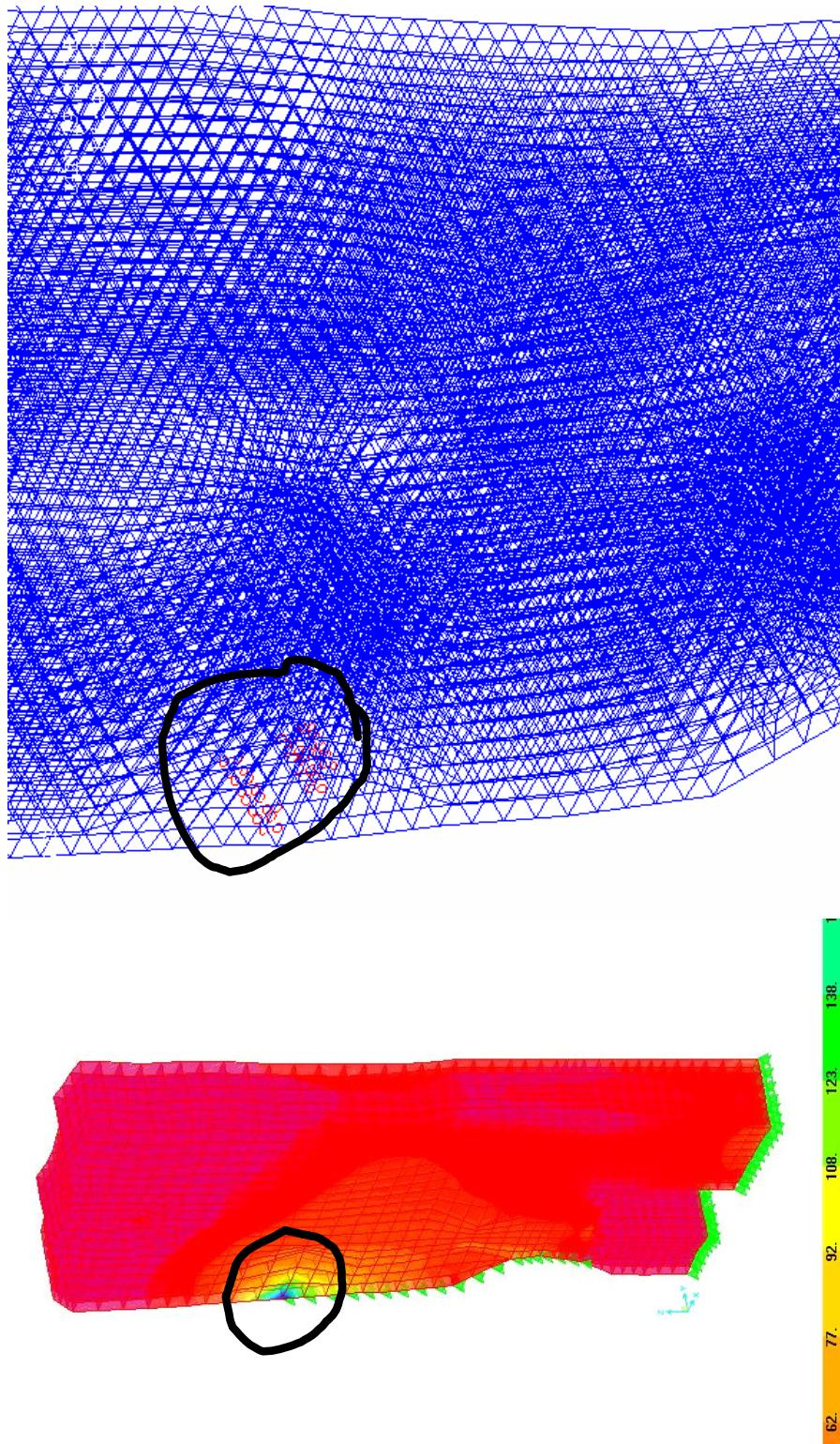
Figure 4.37 The comparison of the crack locations for linear and non-linear analysis for Load Case-3
