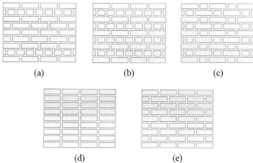
**Figure 2. 2 Different arrangements for brick masonry; a) American (common) bond b) English (cross) bond c) Flemish bond d) Stack bond e) stretcher bond [6]**
