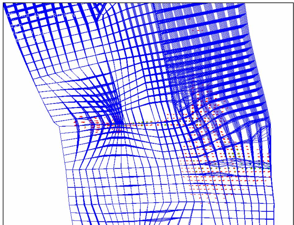
Figure 4.19 Crack pattern for un converged solution for Load Case-1.
