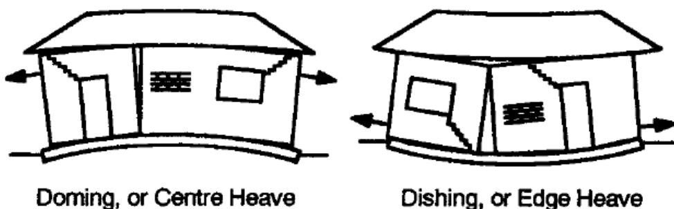
**Figure 3.2 Doming and dishing differential foundation profiles [27].**
