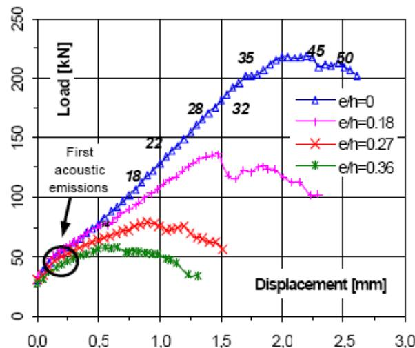
**Figure 2. 19** Load-displacement diagrams for different eccentricity rates [19].
