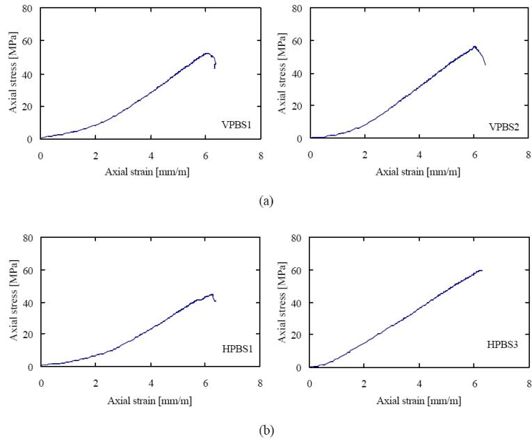
**Figure 2.16 Stress-strain graphics for four prismatic brick specimens tested under axial displacement control; a) vertical direction b) horizontal direction [7].**
