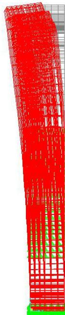
Figure 4.35 Z component of displacement at ultimate load for Load Case-3 (linear analysis).
