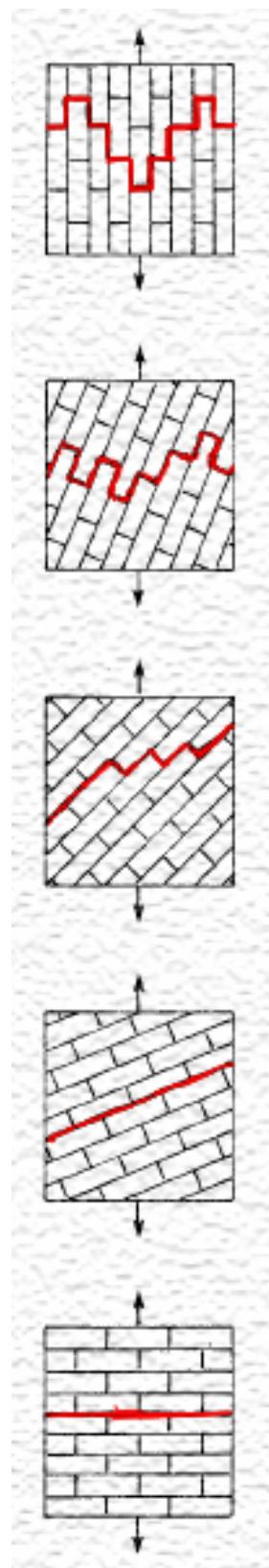
**Figure 3.10** Crack patterns of masonry under biaxial tension.
