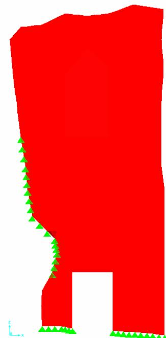
**Figure 4.7** Restraints of the finite element model
