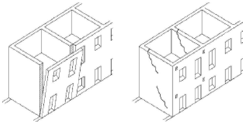
**Figure 3.17 Basic damage modes of a masonry building [32].**
