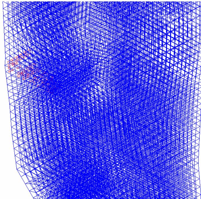
**Figure 4.33** Crack pattern for un converged solution for Load Case-3.
