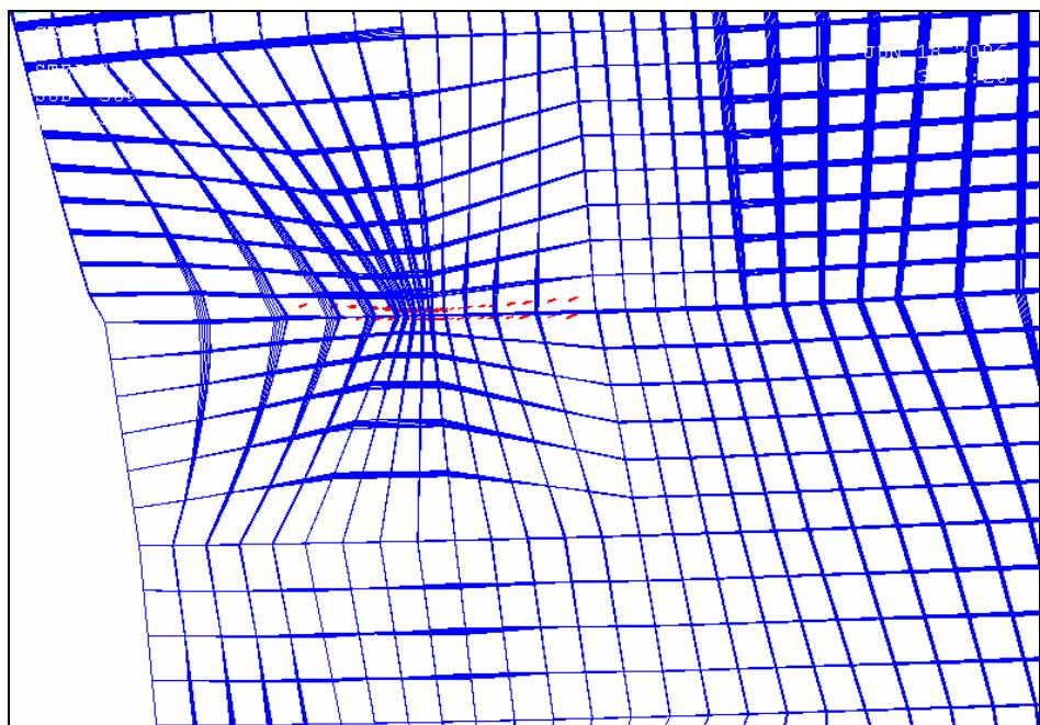
Figure 4.18 Crack pattern at ultimate load for Load Case-1.
