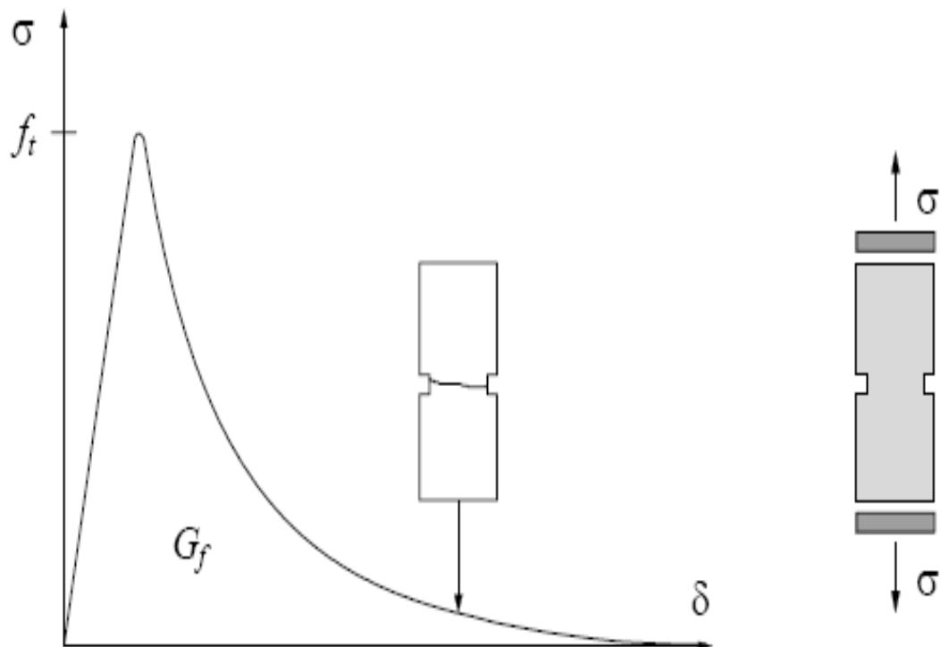
**Figure 2. 21 Typical behavior of quasi-brittle materials under uniaxial tension and definition of fracture energy [6].**
