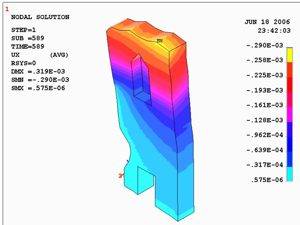
Figure 4.20 X component of displacement at ultimate load for Load Case-1 (non-linear analysis).
