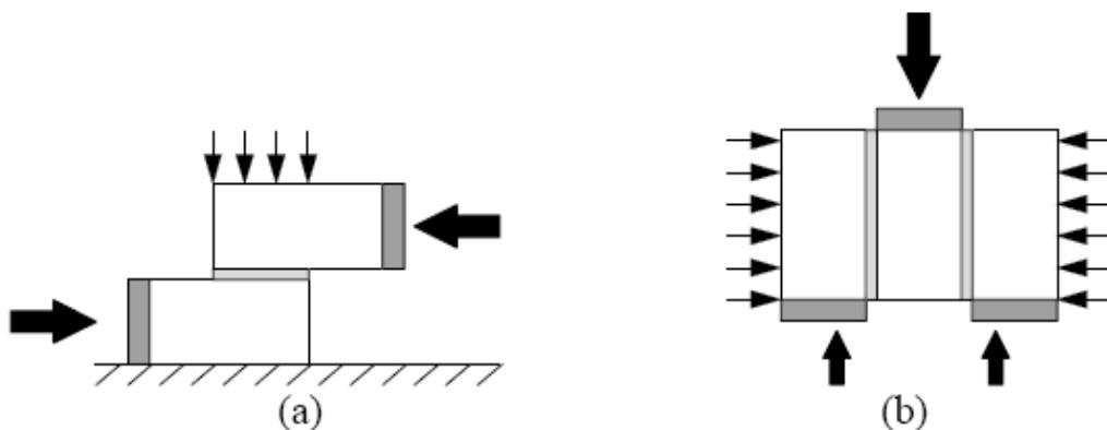
**Figure 2. 14 Possible test set-ups for determination of shear bind strength; a) couple test b) triplet test [6].**
