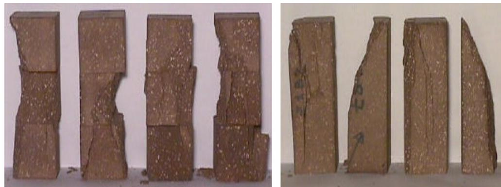
**Figure 3.4 Failure mechanisms of the prismatic brick specimens [11].**
