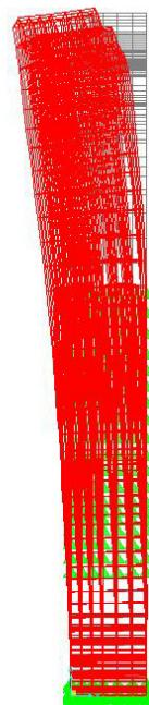
Figure 4.35 Z component of displacement at ultimate load for Load Case-3 (linear analysis).
