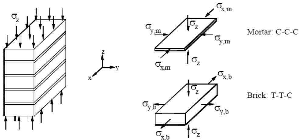
**Figure 2.18** Masonry prism under compressive loading normal to bed joints and stress states for brick and mortar elements (C: compression, T: tension) [11].
