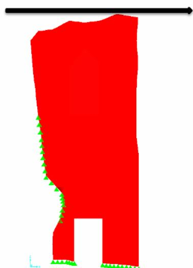
**Figure 4.14 Load Case-1, inertial force is to the right (in-plane).**
