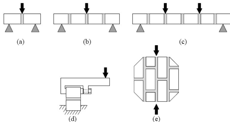
**Figure 2. 13 Possible test set-ups for determination of bind strength; a) three point bending with a single joint b) three point bending with a longer specimen c) four-point bending d) bind-wrench test e) splitting test [6]**
