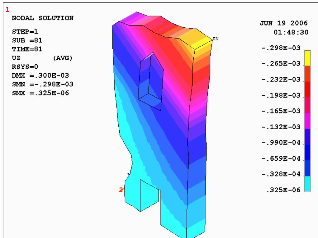
Figure 4.34 Z component of displacement at ultimate load for Load Case-3 (non-linear analysis).
