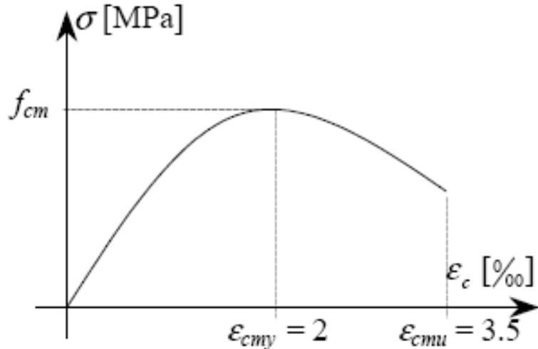
Figure 2.24 Parabolic stress-strain relationship for masonry [20].
