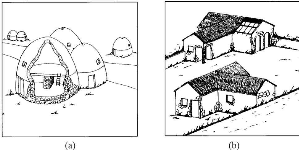
**Figure 2. 3 Examples of prehistoric architecture of masonry in the Ancient Near East; a) beehive houses from a village in Cyprus (c.5650 BC) b) rectangular dwellings from a village in Iraq [6].**
