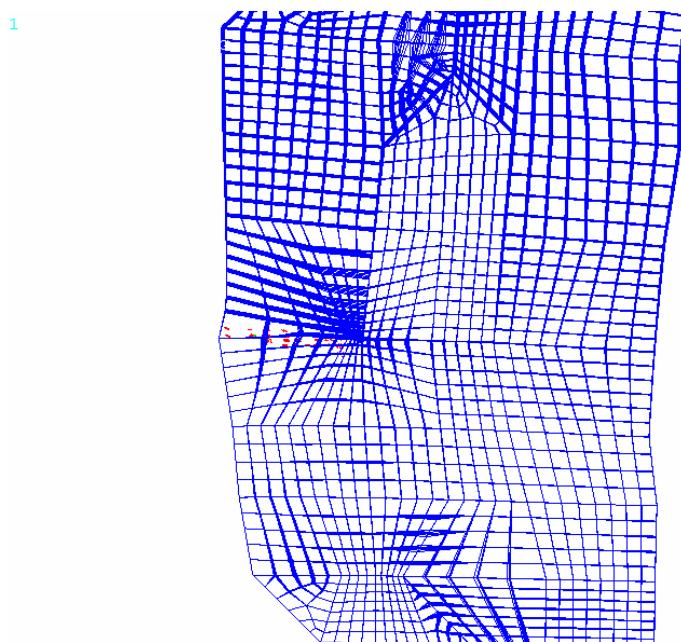
**Figure 4.26** Crack pattern for un converged solution for Load Case-2.
