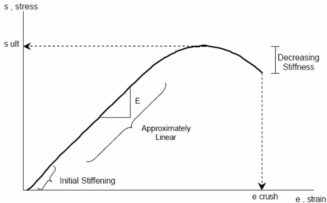
Figure 2. 23 Fundamental stress-strain diagram for masonry under compression
