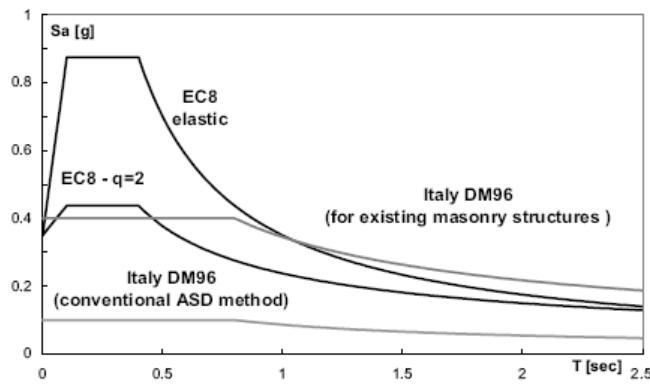
Figure 3. 1 EC8 elastic and reduced spectra and Italian Seismic Code spectra [26].
