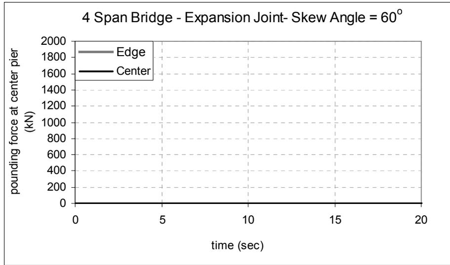
Figure 5.85: Pounding force at the center pier of the bridge without link slab
