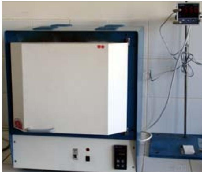
**Figure 3.2 Muffle furnace for solutionizing**
