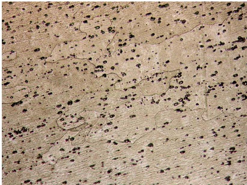
**Figure 4.1 Microstructure of as-received Al 6066 (200X)
