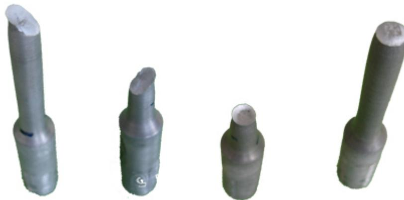
**Figure 4.8 Macroscopic fracture surfaces**
