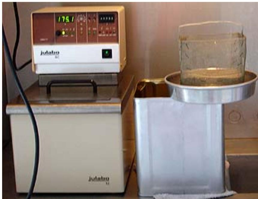
**Figure 3.4 Julabo heating circulator for aging**
