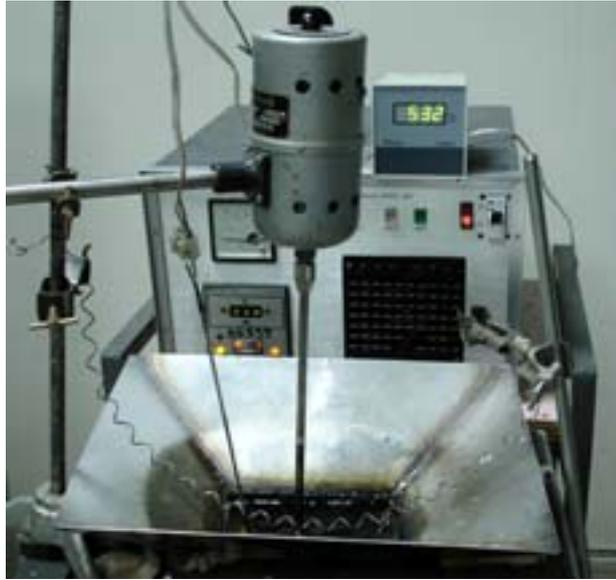
**Figure 3.3 Salt bath for solutionizing**
