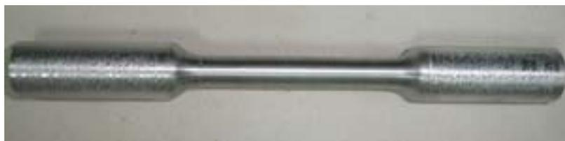
**Figure 3.10 Small-sized specimen proportional to standard tension specimen**
