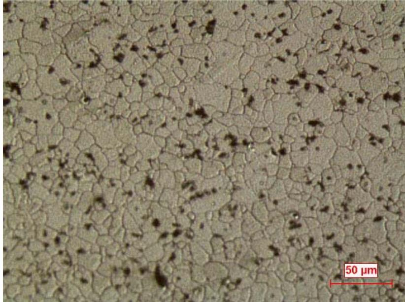
**Figure 4.2 Microstructure of Al 6066 – T6 (200X)**
