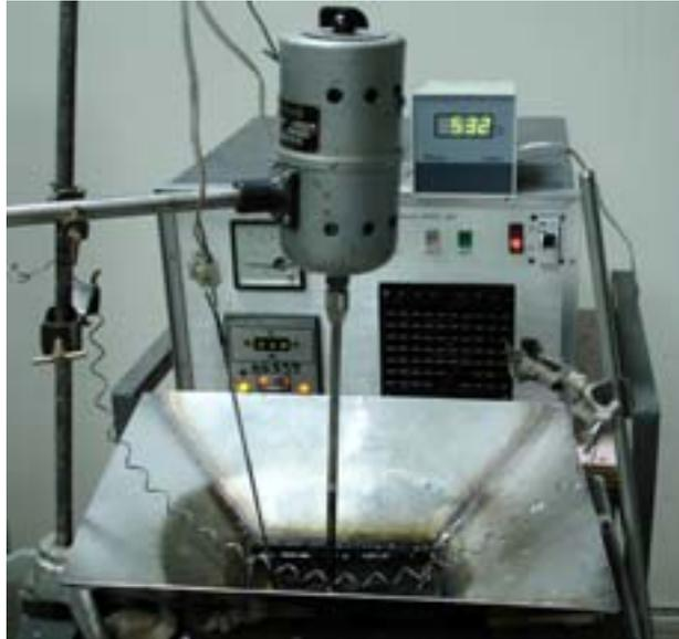
**Figure 3.3 Salt bath for solutionizing**
