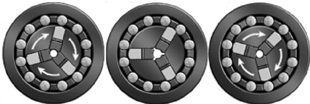
**Figure 3.5 Operation scheme of swager**
