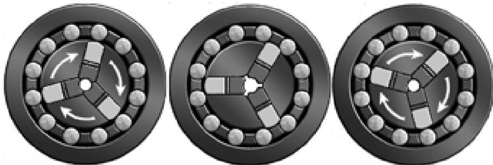
**Figure 3.5 Operation scheme of swager**
