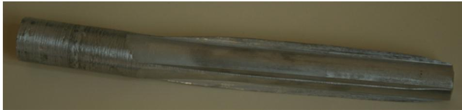
**Figure 3.7 Failure of 40% deformation at 200°C with single pass**
