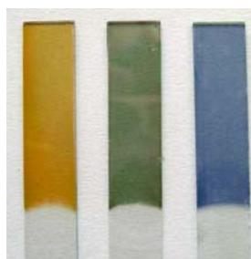
**Figure 3.35** Colors of the electrochromic electrodes of POTE at different potentials
