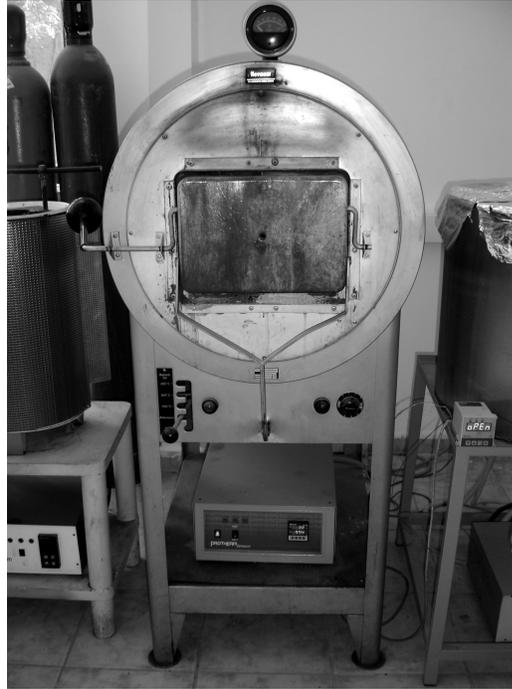
**Figure 3.1** Hereaus Annealing Furnace
