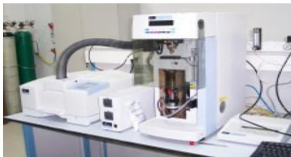
**Figure 3.1.** Photograph of the TG-FTIR instrument
