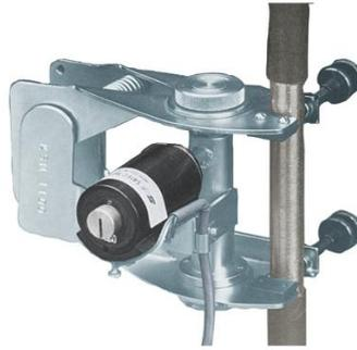
**Figure 2.9** Mechanical extensometer
