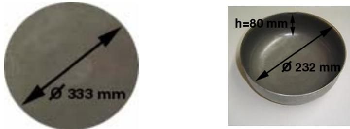
**Figure 1.1** Blank after trimming and the final part
