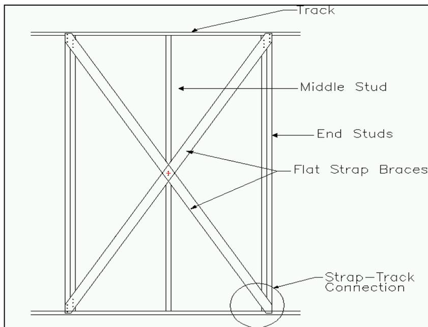
Figure 5.1 General Drawing of Frame with X-bracing.
