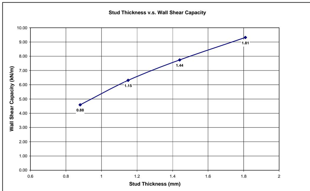
Figure 5.7 Stud Thickness vs. Wall Shear Capacity curve
