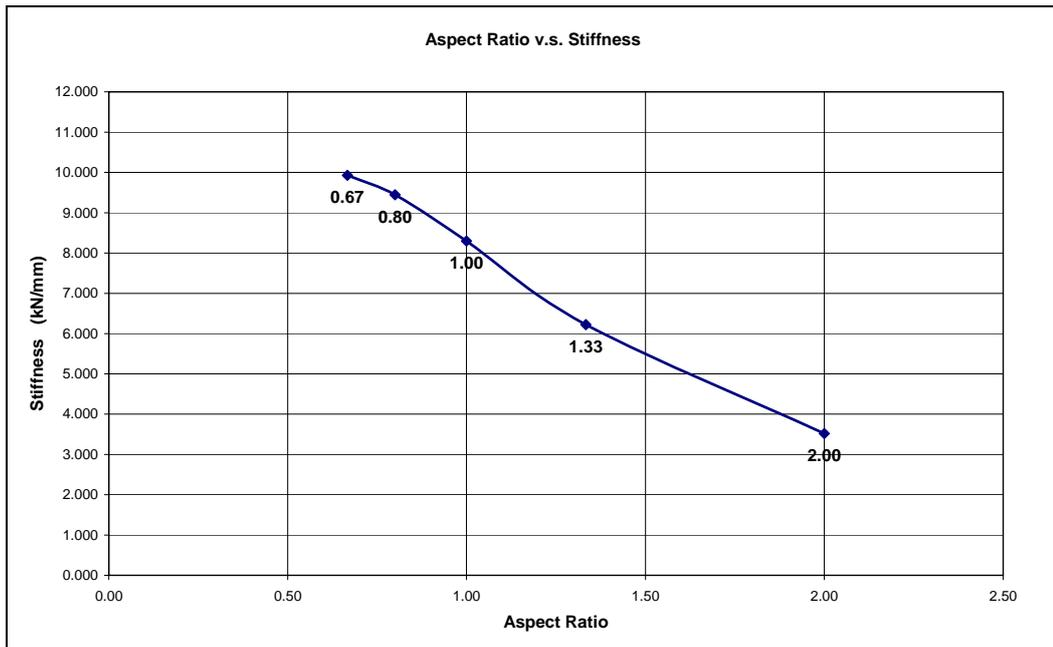
Figure 5.10 Change of Stiffness with Aspect Ratio curve
