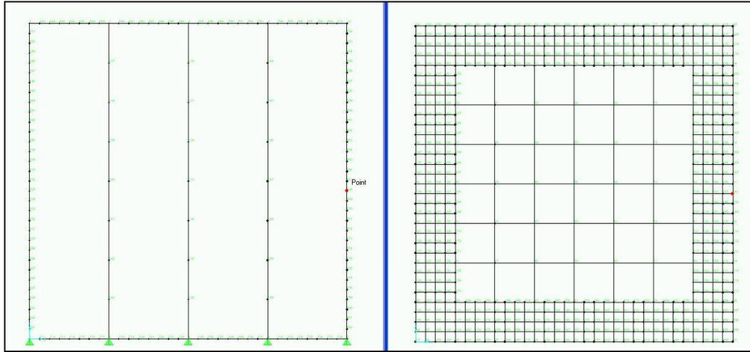
Figure 4.5 Steel Frame and Meshed Shell of Sap2000 model
