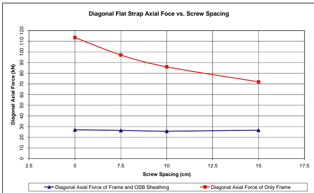
Figure 6.4 Diagonal Flat Strap Axial force vs. Screw Spacing with and without X-bracing
