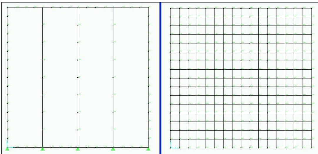
Figure 4.1 Steel Frame and Meshed Shell of Sap2000 model
