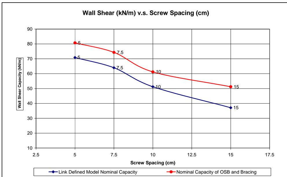
Figure 6.3 Nominal Capacities of Walls vs. Screw Spacing with and without X-bracing
