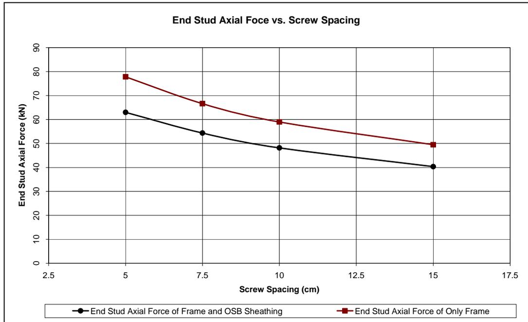
Figure 6.5 End Stud Axial Force vs. Screw Spacing with and without X-bracing
