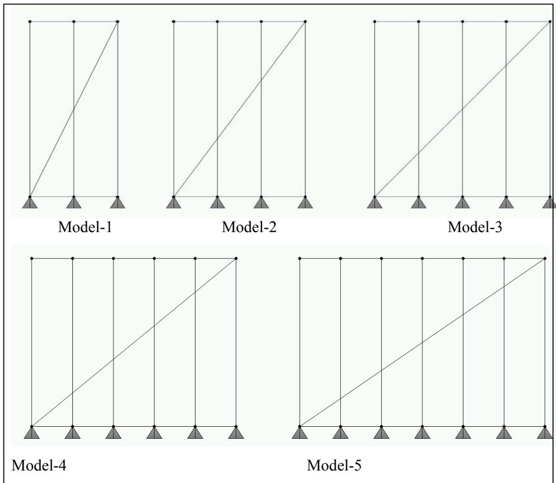
Figure 5.8 Analytical models of shear wall with X-bracing with different aspect ratios
