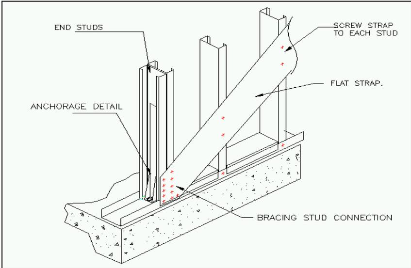
Figure 5.3 Bracing-frame connection detail
