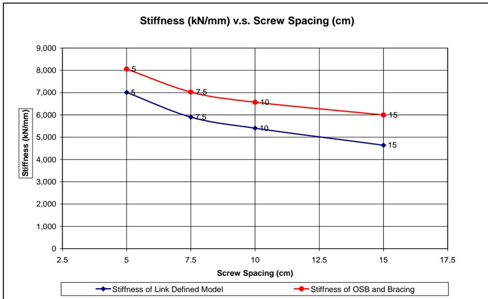
Figure 6.2 Stiffness of Walls vs. Screw Spacing with and without X-bracing
