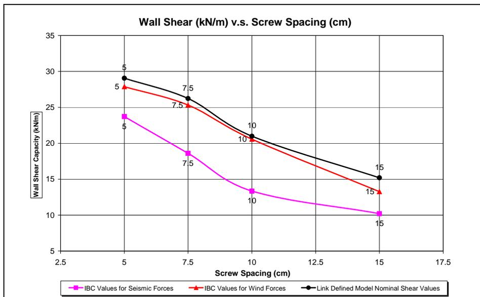
Figure 4.12 Comparison of Nonlinear Link defined Model Nominal Shear Capacity with IBC nominal shear values for wind and seismic forces
