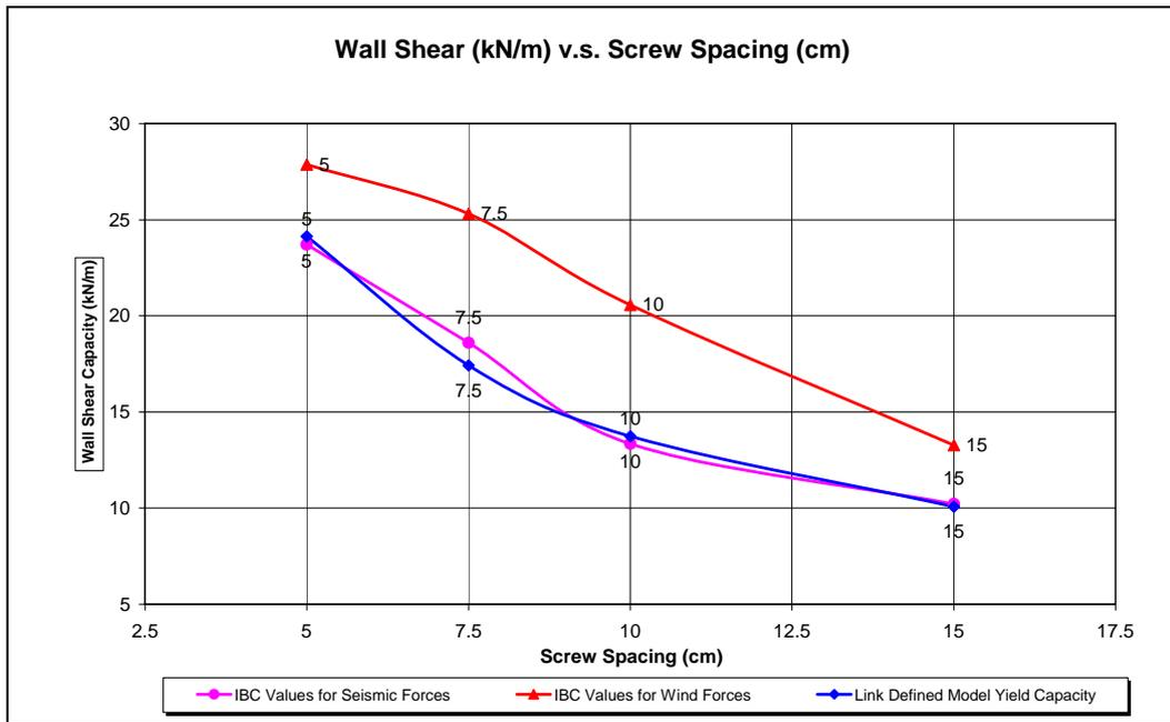
Figure 4.10 Comparison of Nonlinear Link defined Model yield Capacity with IBC nominal shear values for wind and seismic forces
