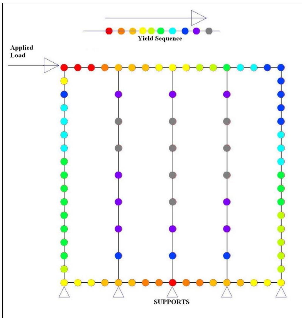
Figure 4.16 Yield pattern for the shear wall with 15 cm screw spacing on center at perimeter.
