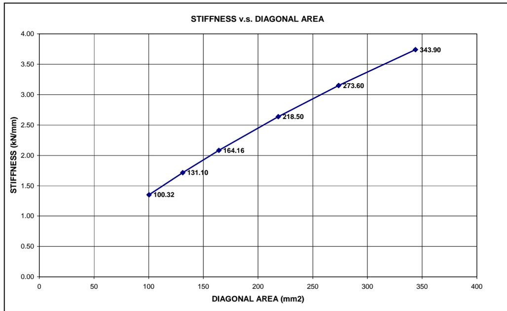
Figure 5.5 Stiffness vs. Diagonal Area curve
