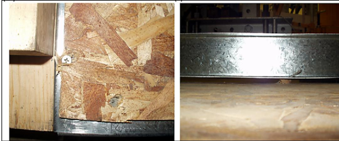
Figure 2.1 Deformation on OSB and screw pulling-out from OSB at tests done by Tian, Wang and Lu (2003)
