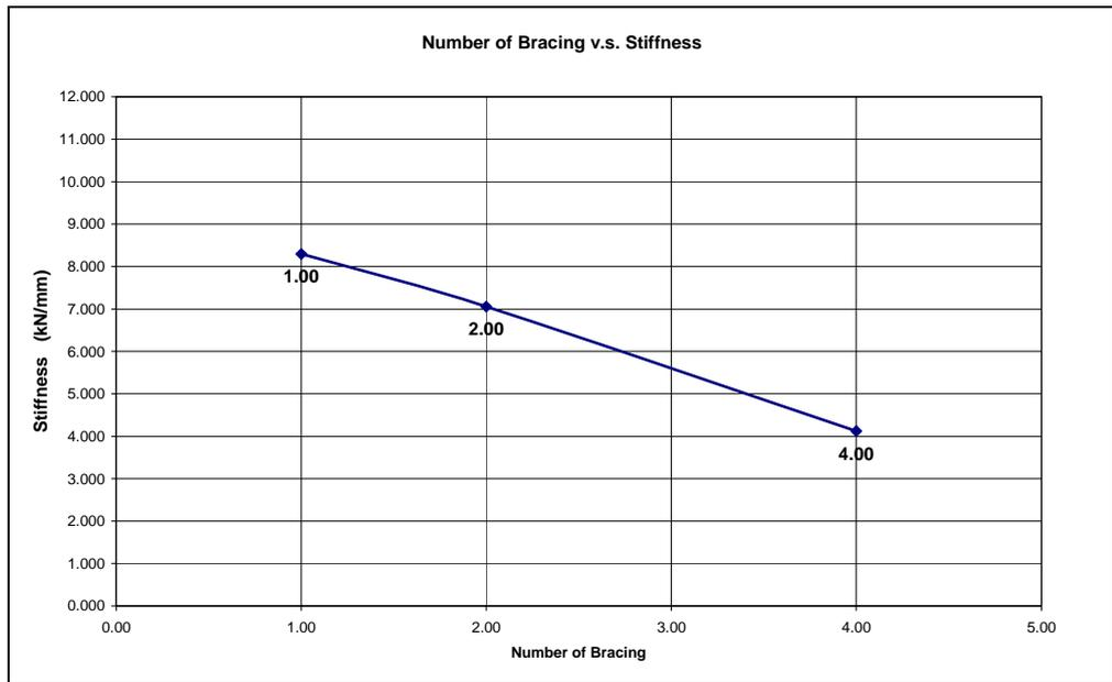
Figure 5.12 Change of Stiffness with Number of Bracing curve
