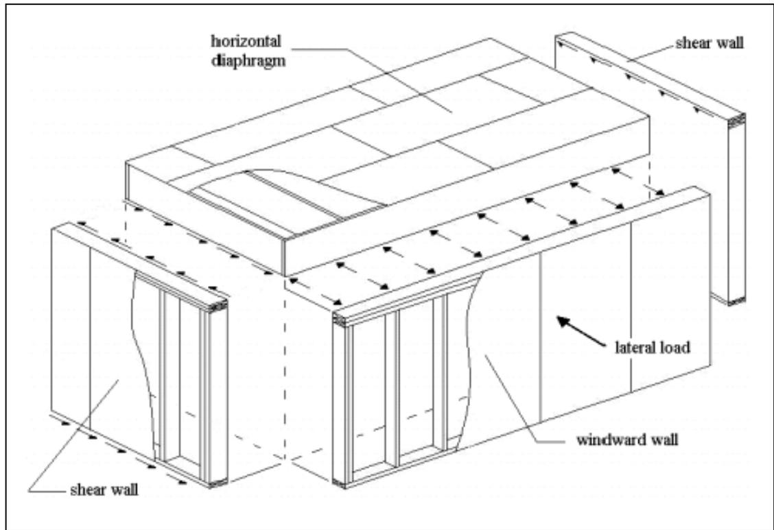
Figure 1.8 Lateral Load Carrying Mechanism of Light framed Building, Bredel (2003)
