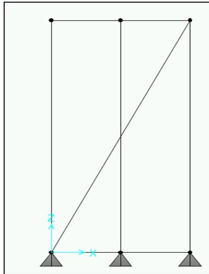
Figure 5.6 Sap2000 model of frame.
