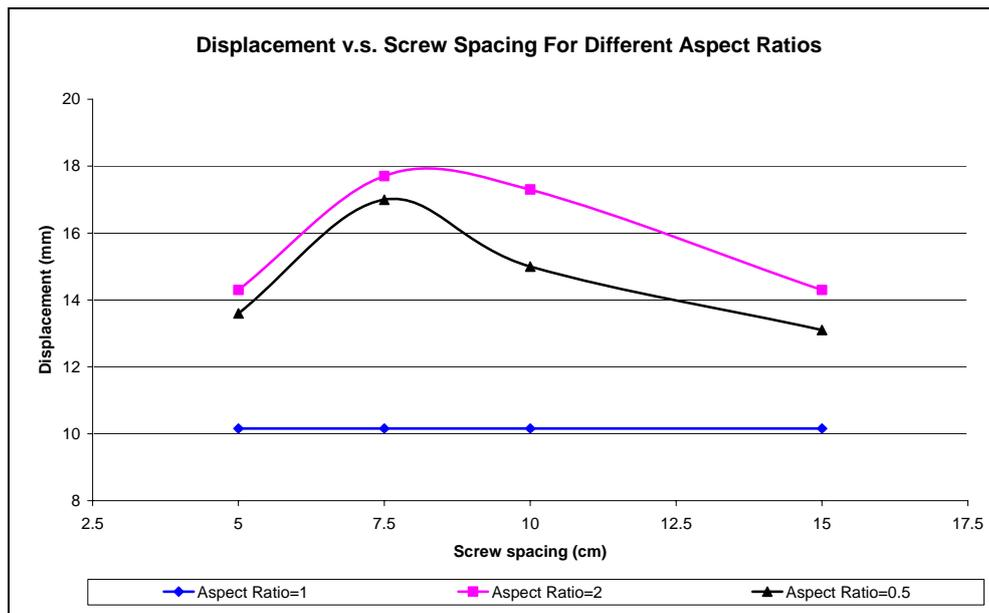
Figure 4.15 Displacement values of frames for different aspect ratios for four different screw spacing
