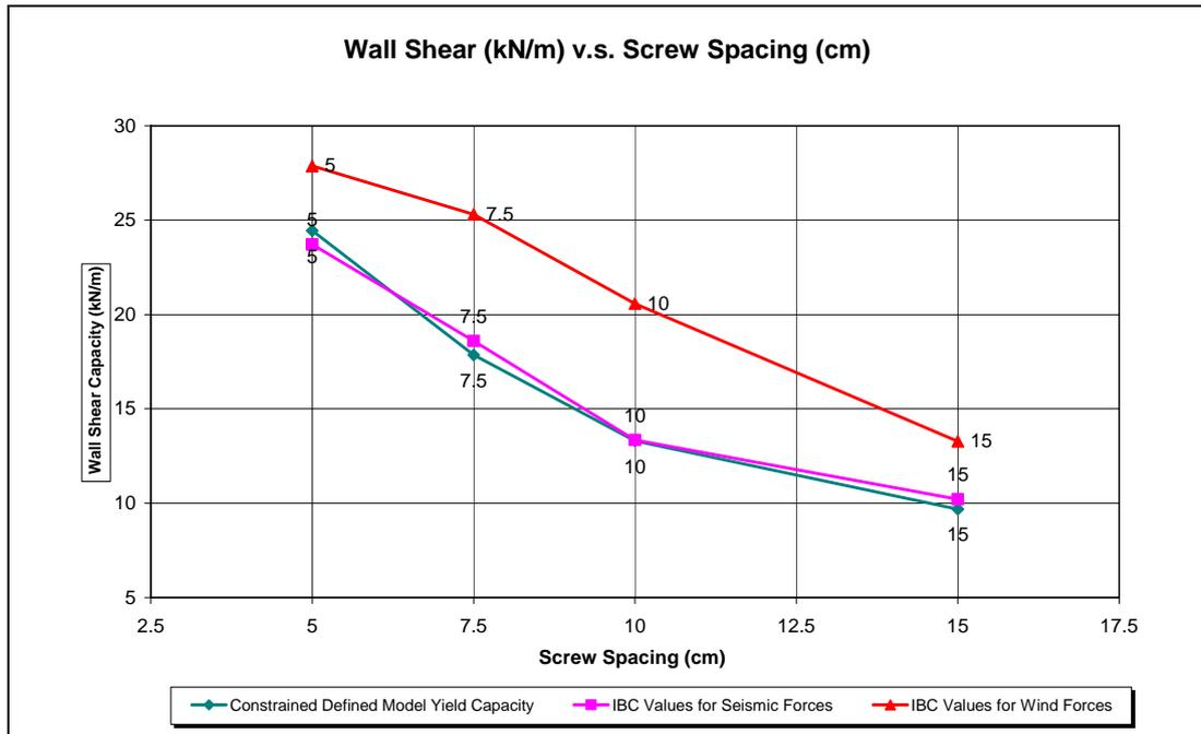
Figure 4.9 Comparison of Constraint defined Model yield Capacity with IBC nominal shear values for wind and seismic forces
