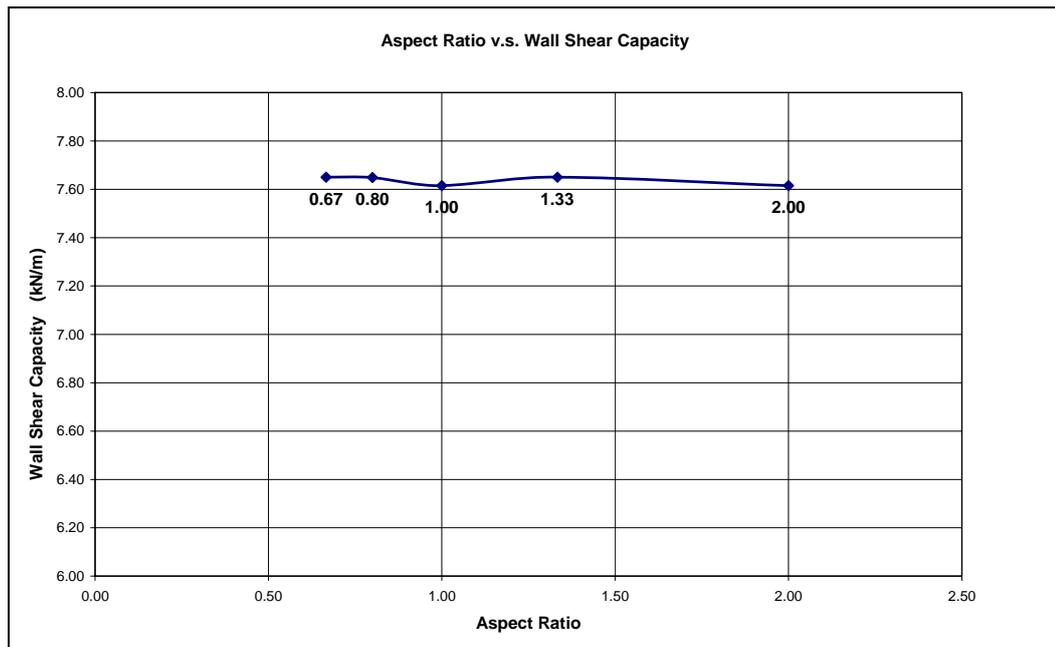
Figure 5.9 Change of Unit Wall Shear Capacity with Aspect Ratio curve
