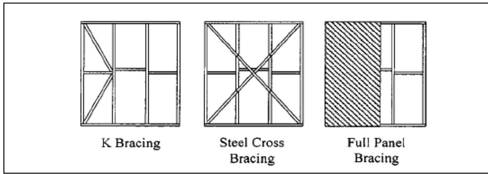
Figure 1.6 Bracing Types Used in Light Framed residential structures, Serrette (1997)
