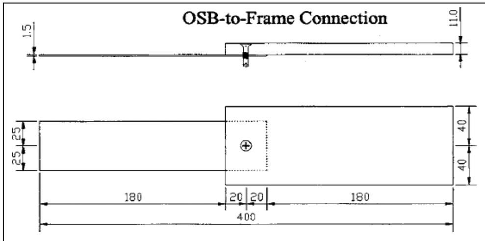
Figure 2.2. Drawing of tested OSB to Steel skeleton connections by Fülöp and Dubina (2006)
