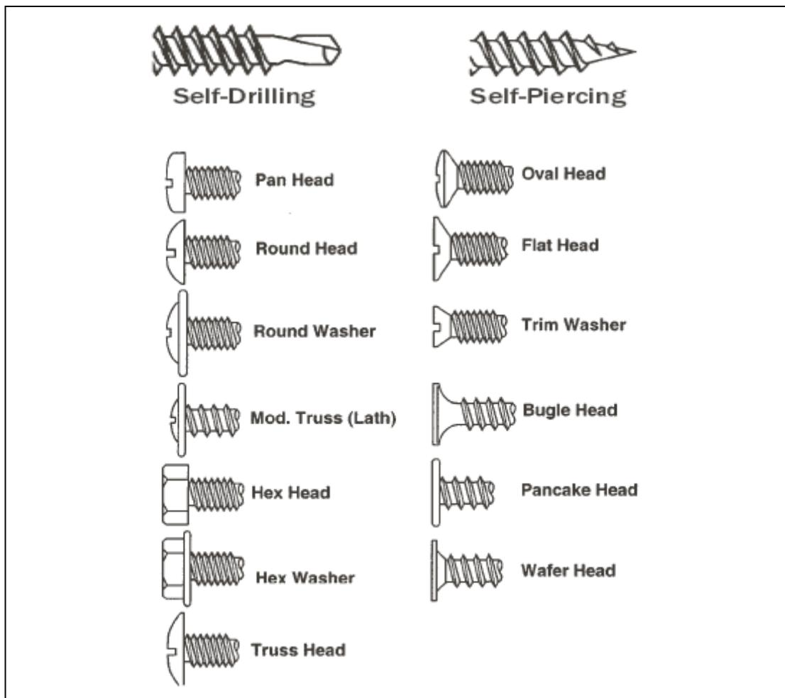
Figure 3.3 Head and Types of screws, Prescriptive Method (2000)
