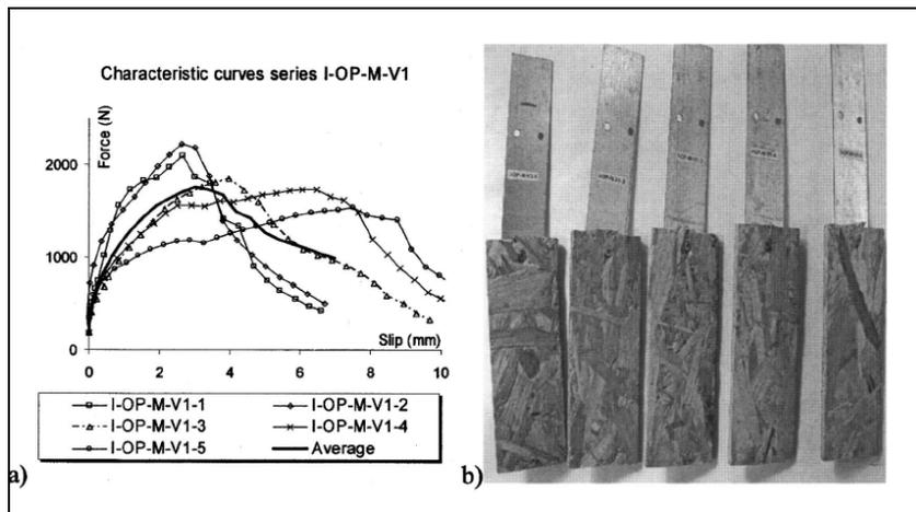
Figure 2.3 Experimental curves and failure modes of OSB to steel connections by Fülöp and Dubina (2006)
