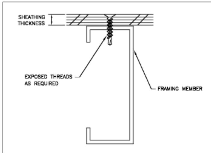
Figure 3.6 Oriented Strand Board and steel stud screw connection, NASFA Publication NT600.
