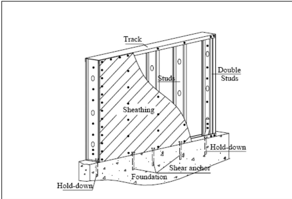
Figure 1.9 Typical Cold Formed Steel Shear Wall, Zhao and Rogers (2002)
