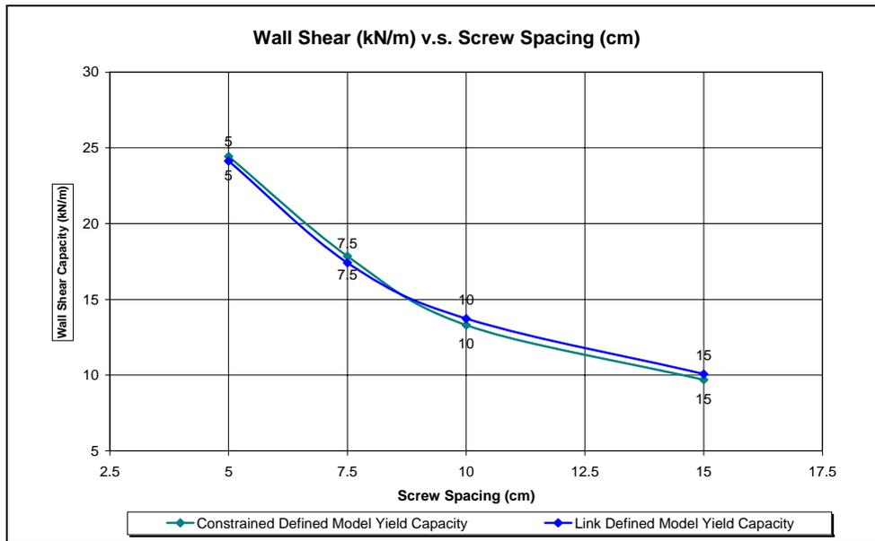
Figure 4.11 Comparison of Nonlinear Link defined Model yield Capacity with Constraint defined Model yield Capacity
