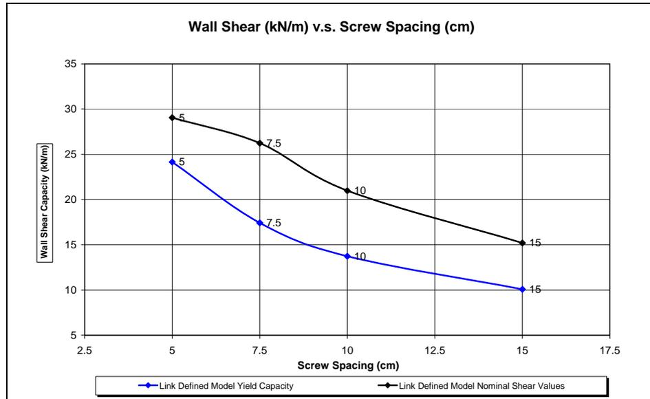
Figure 4.13 Yield and nominal shear values for nonlinear link defined models
