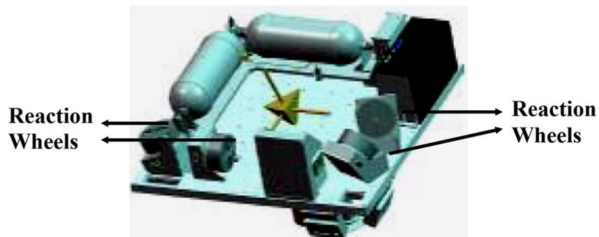
**Figure 1.3 :** Four Wheels in a Tetrahedral Configuration.
