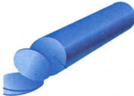
Figure 4.4: Illustration of a silicone ingot and cut wafers [37].
