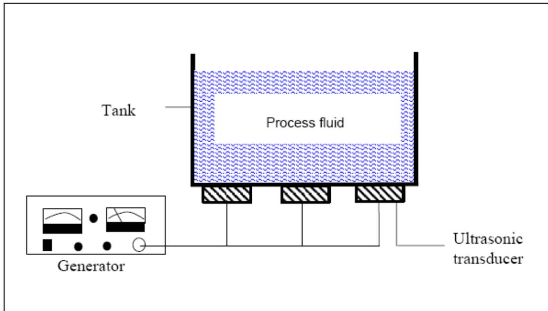
**Figure-14:** Schematic Ultrasonic Bath [Adapted from Fuchs (1999)]
