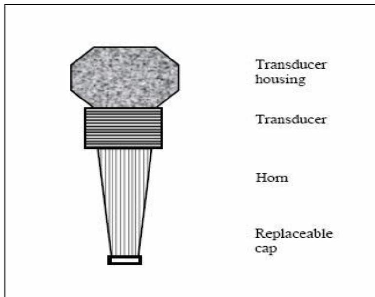
**Figure-17:** Schematic of Ultrasonic Probe [Adapted from Mason (1998)]
