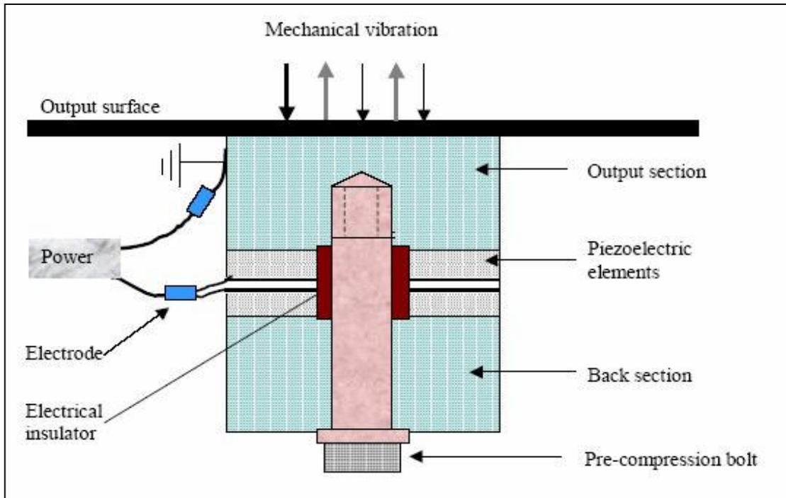
**Figure-16:** Piezoelectric Transducer [Adapted from Fuchs (1999)]
