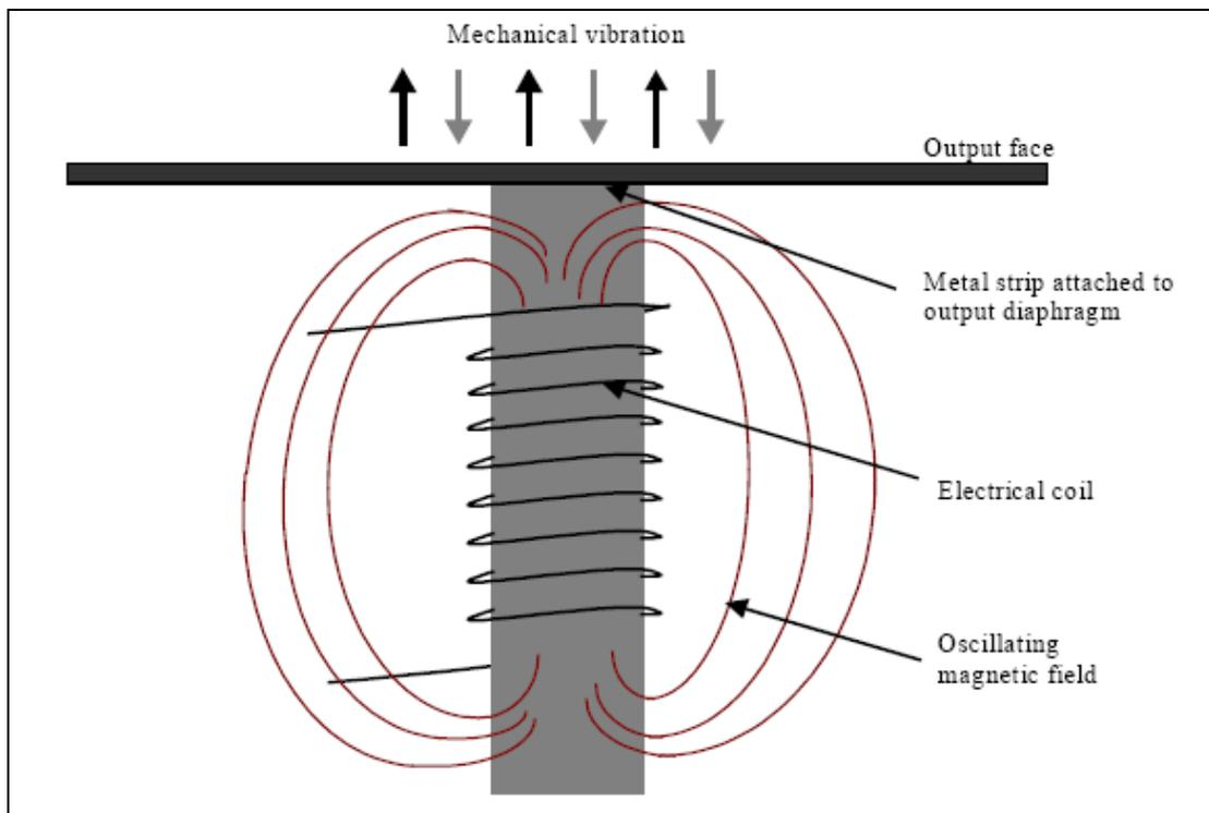
**Figure-15:** Magnetostrictive transducer [Adapted from Fuchs (1999)]
