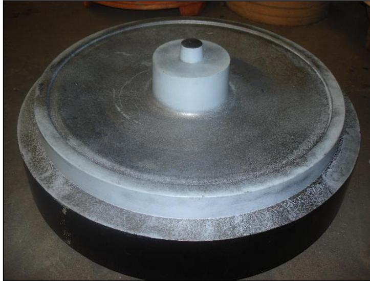
Figure A.1 – Photograph of impeller pattern
