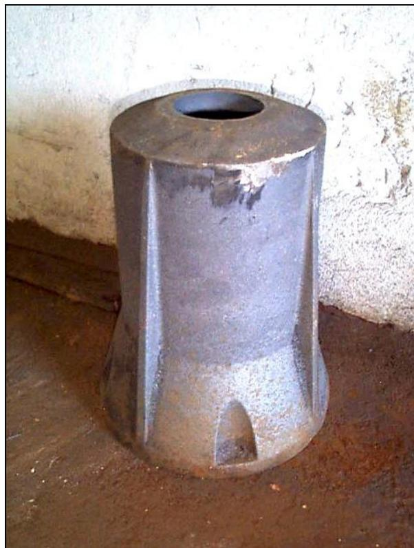
Figure A.12 – Photograph of motor case before machining
