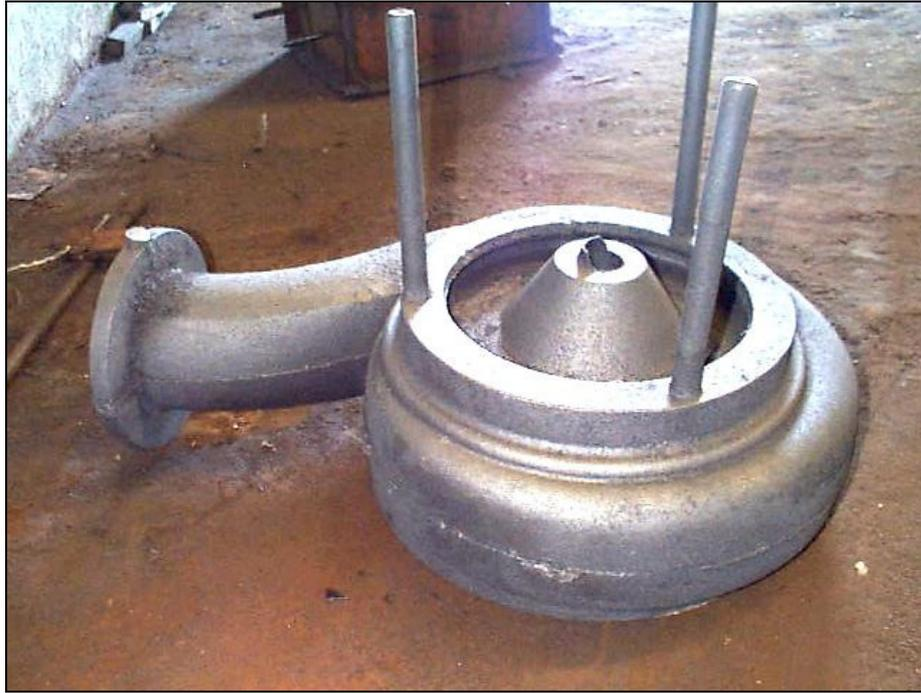
Figure A.11 – Photograph of volute before machining
