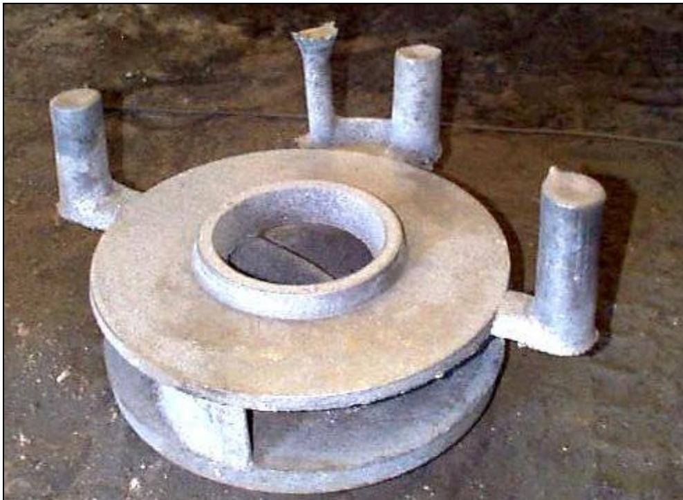
Figure A.10 – Photograph of impeller before machining
