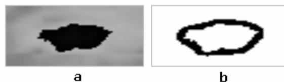
Figure 4.20 a) Gray-scale image, b) Adaptive thresholded image with a 15x15 window, C=-12
