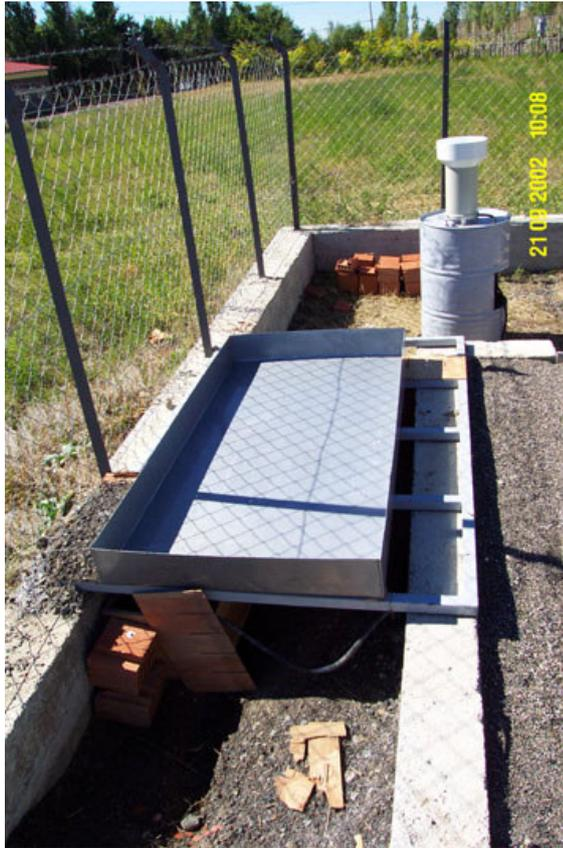
Figure 4.16 Snowmelt lysimeter at Güzelyayla station
