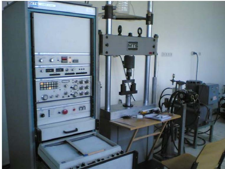
**Figure 5.13** MTS Testing machine in operation during pre-cracking the specimens
