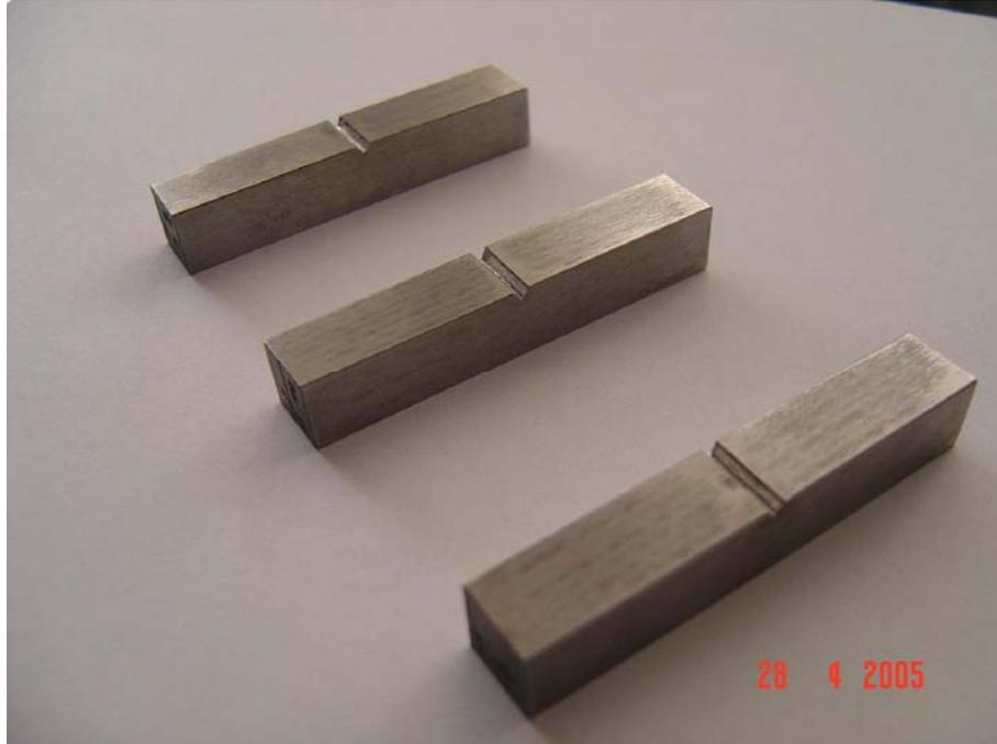
**Figure 5.9** Charpy impact bar samples prepared after heat treatment
