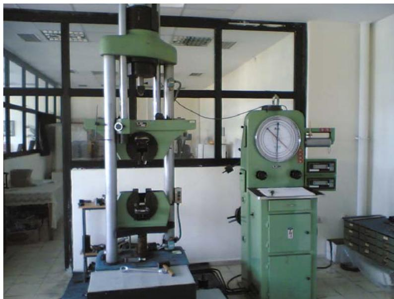
**Figure 5.14** Alsa Laboratory Machine used to fracture the specimens until failure
