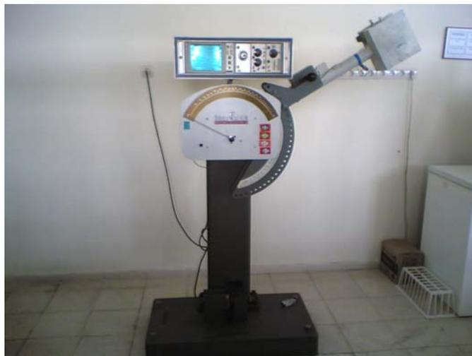
**Figure 5.10** Charpy impact test machine used.
