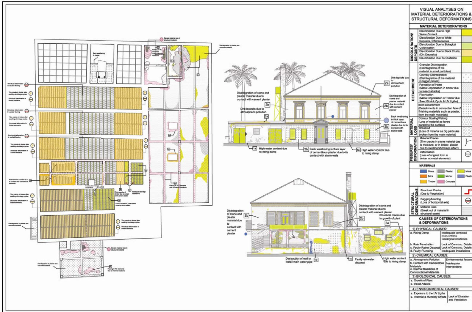
Drawing 2.34 Analysis on Material Deteriorations and Structural Deformations
