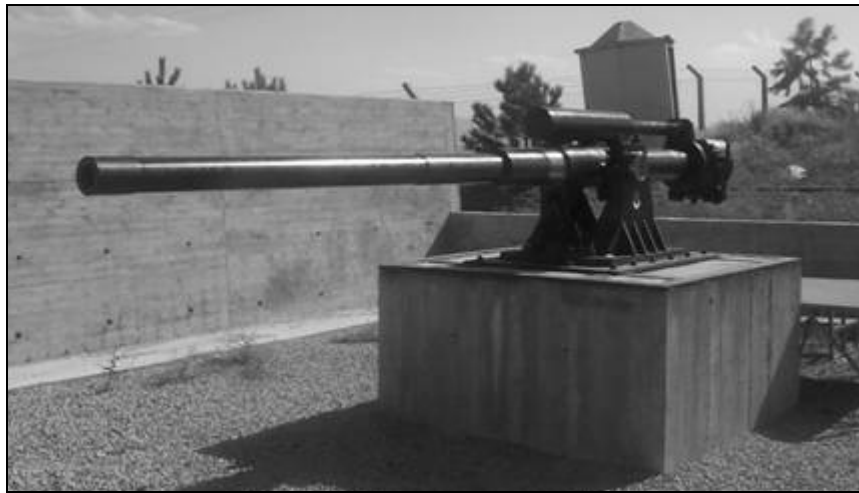
Figure 1.1 Powder gas gun used at FML
