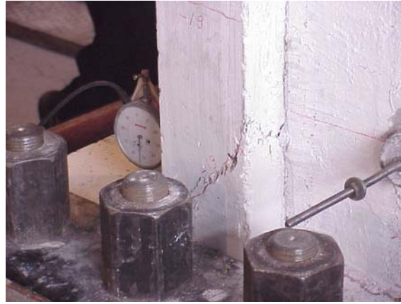
Figure 5.44 – Column Base Damage in the Nineteenth Cycle, Specimen CID4
