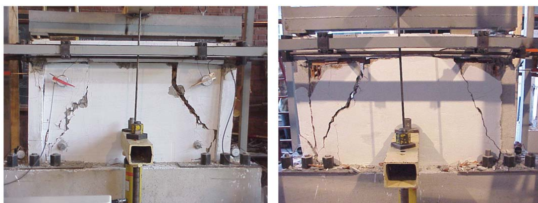
Figure 5.63 – General View of Specimen LIC4 after the Test
