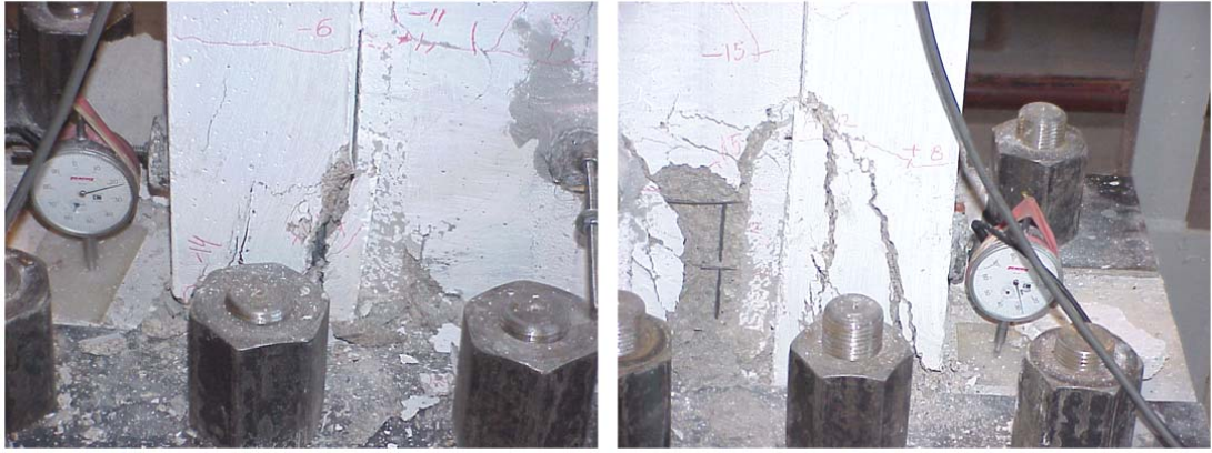
Figure 5.72 – Damage in the Lap-Splice Region of the Column, Specimen LID4
