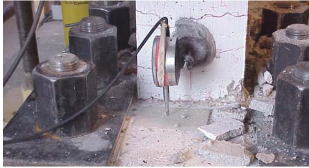
Figure 5.52 – Cracking at the Column Base and Lap-Splice Level in the Fourth Cycle, Specimen LR
