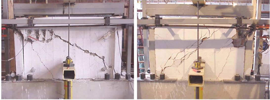
Figure 5.47 – General View of Specimen CID4 after the Test
