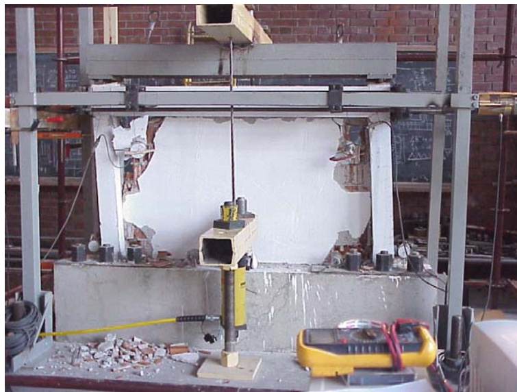
Figure 5.53 – Deformation in the Frame during the Test, Specimen LR
