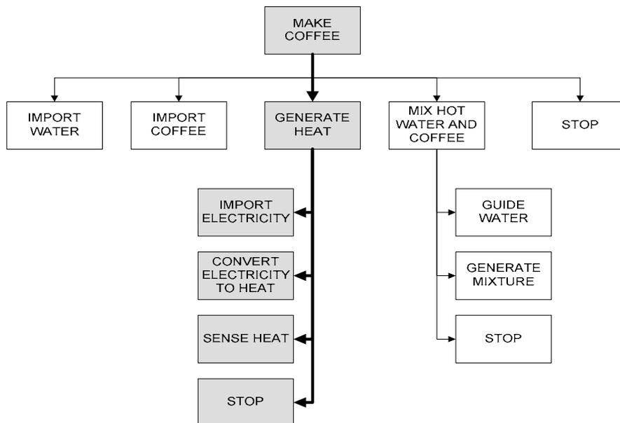
Figure 5.7 Functional Design Tree of Coffee Machine
