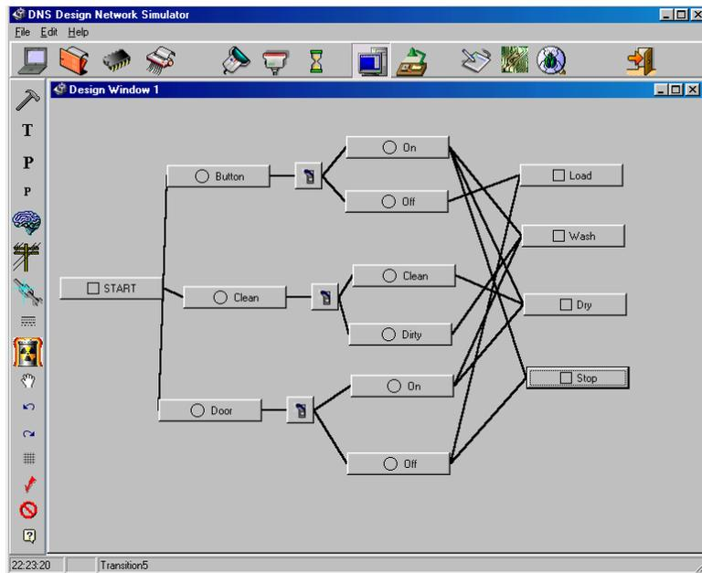
Figure 4.10 Creation of N-PNDN for the dish machine (continued)
