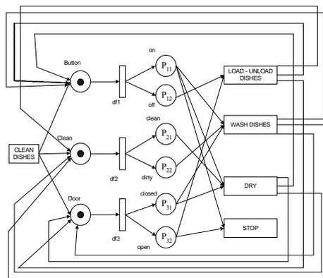
Figure 3.5 Token Flow First Step for Dish Machine (Korkmazel, 2001)
