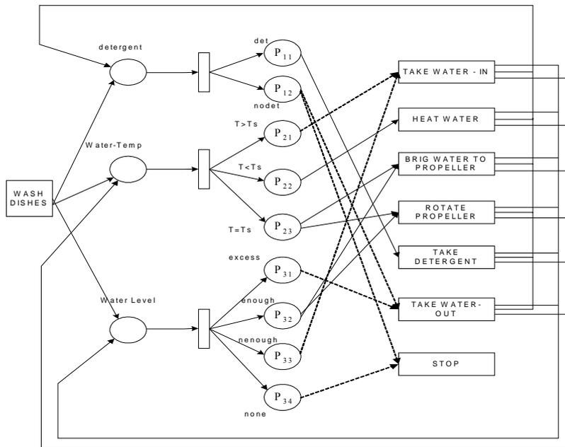
Figure 3.3 The sub-layer of the functional state Wash Dishes and its functional decomposition, (Korkmazel, 2001)
