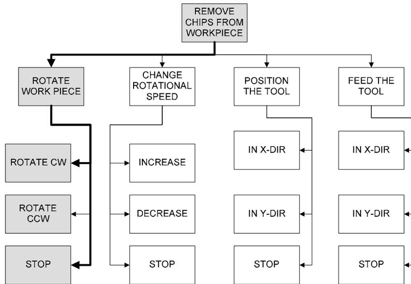
Figure 5.10 Functional Design Tree Lathe
