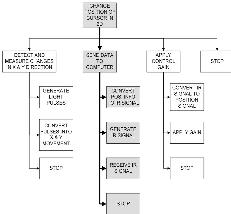
Figure 5.1 Functional Design Tree of Mouse
