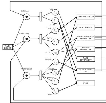
Figure 3.8 Token Flow Fourth Step for Dish Machine (Korkmazel, 2001)
