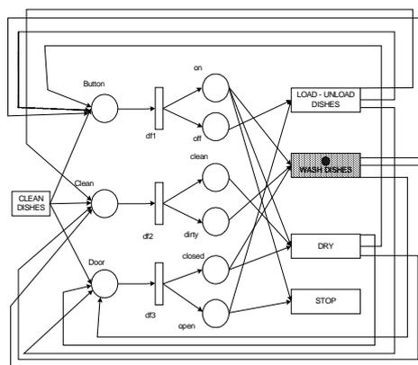
Figure 3.7 Token Flow Third Step for Dish Machine (Korkmazel, 2001)
