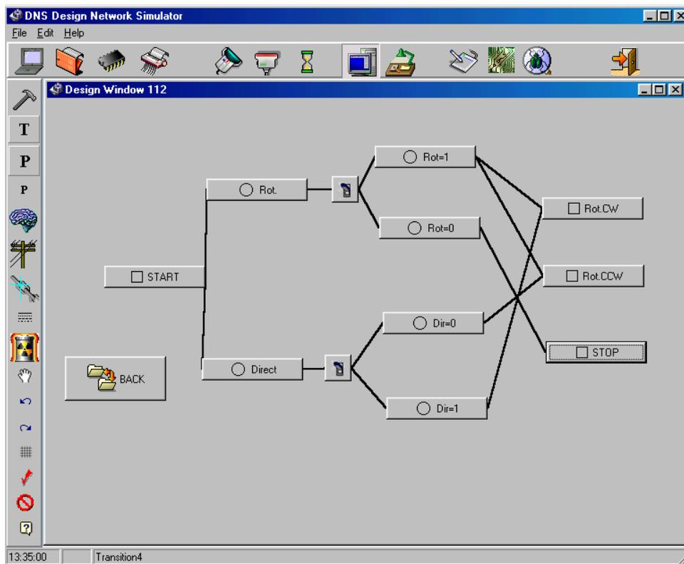
Figure 5.12 PNDN model of “Rotate Workpiece” subfunction
