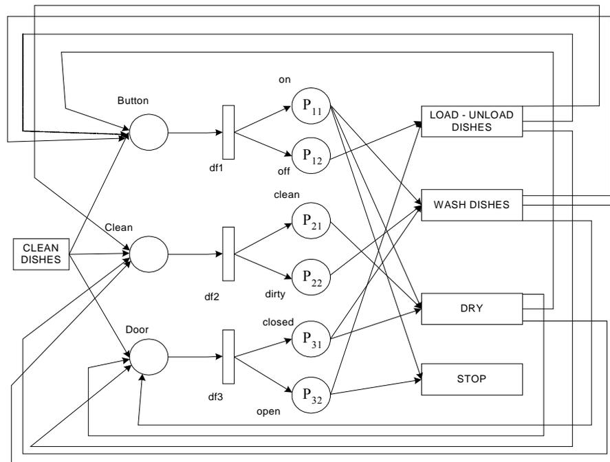
Figure 3.2 N-PNDN of the Dish Machine, the top most level of Dish Machine, (Korkmazel, 2001)
