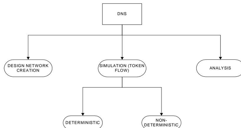
Figure 4.1 Architecture of Design Network Simulator.
