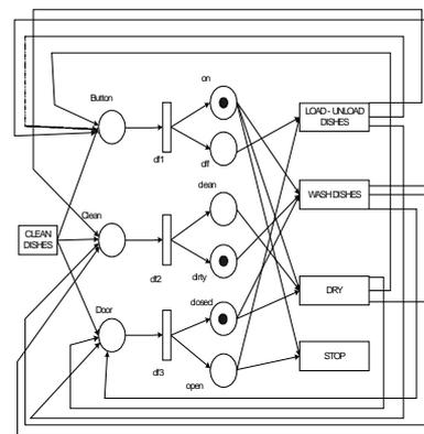
Figure 3.6 Token Flow Second Step for Dish Machine (Korkmazel, 2001)
