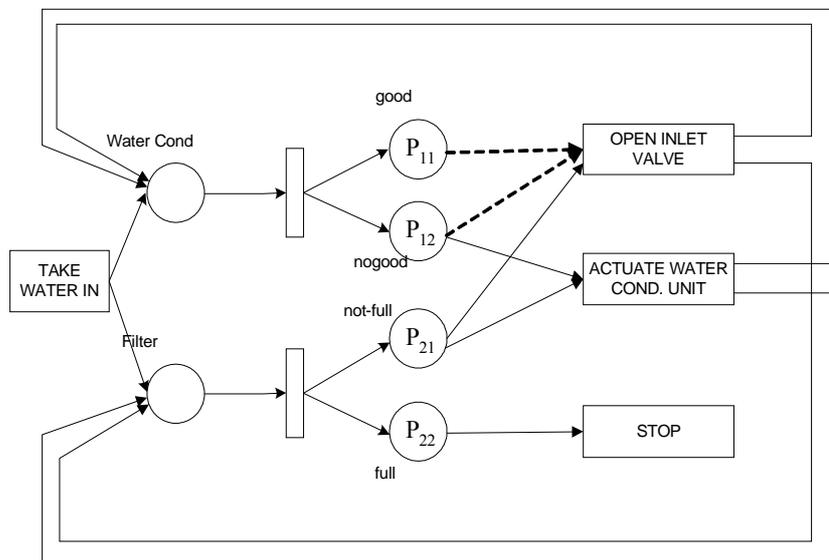
Figure 3.4 The sub-layer of the functional state Take Water - In and its functional decomposition, (Korkmazel, 2001)
