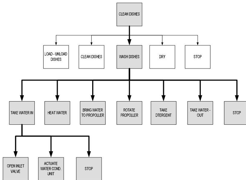
Figure 3.1 The Functional Design Tree of Dish Machine (Korkmazel, 2001)
