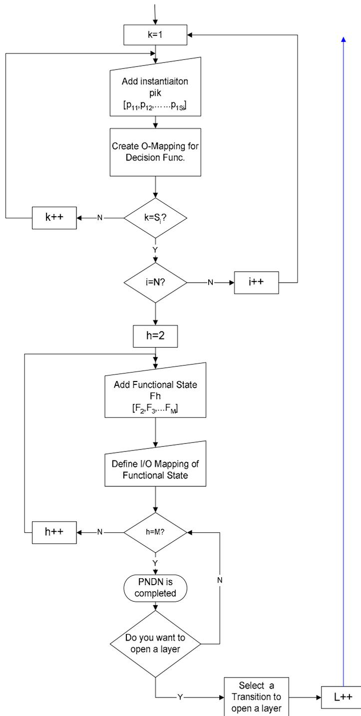
Figure 4.6 Algorithm for the Creation for N-PNDN
