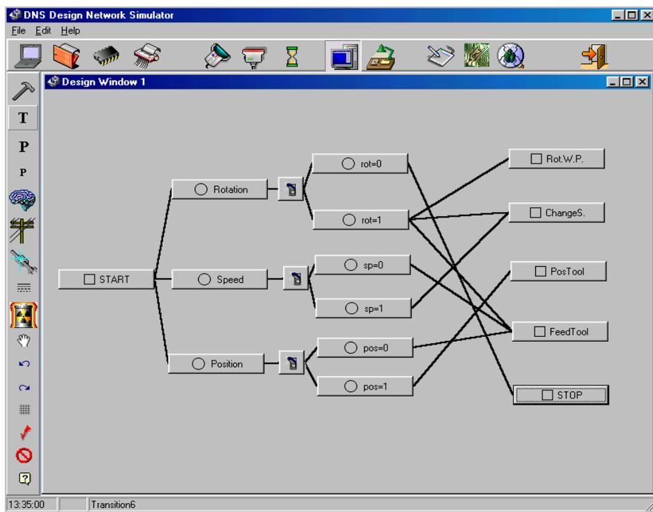
Figure 5.11 PNDN model for Lathe
