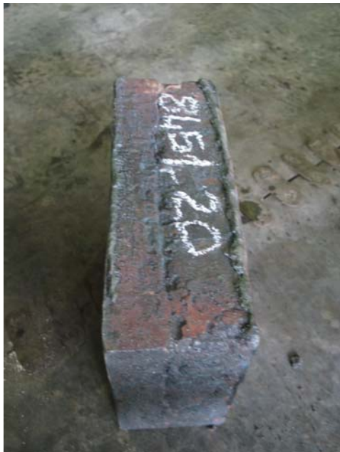
Figure 4.2 Oxygen blown bloom
