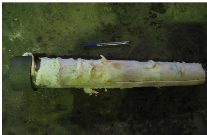
Figure 3.2. Silica type nozzle (SEN).
