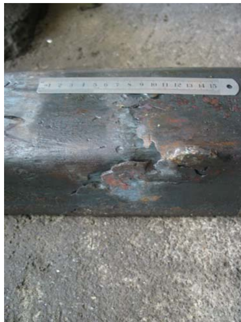
Figure 4.3 Effect of oxygen blowing after hot rolling of blooms (Billet).
