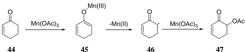
**Scheme 27.** The Suggested Mechanism for the Mn(OAc)<sub>3</sub> Oxidations of Enones
