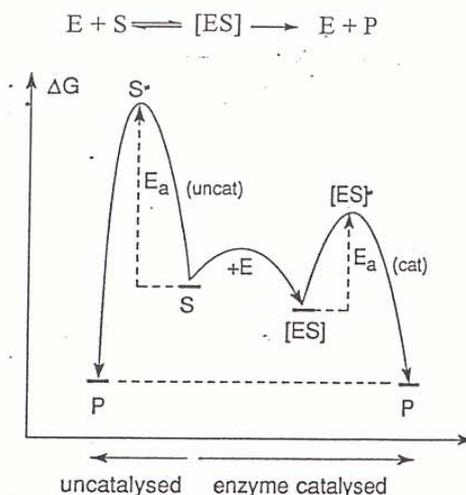
Figure 8. Energy Diagram of Catalyzed versus Uncatalyzed Reaction
