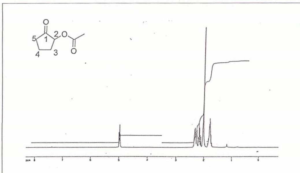
**Figure 32.**  $^1\text{H}$ -NMR Spectrum of 2-Acetoxycyclopentanone (**53a**)
