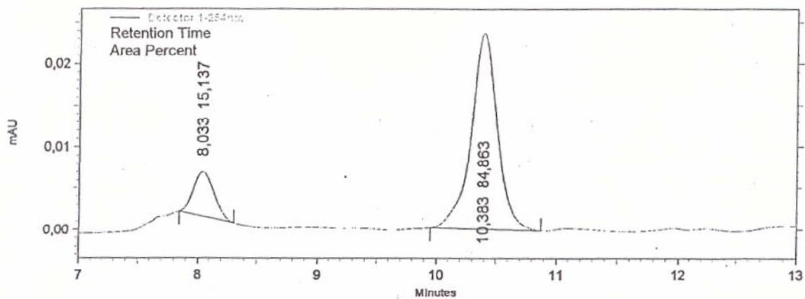
**Figure 19.** The HPLC-Chromatogram of (+)-22 from PPL Hydrolysis
