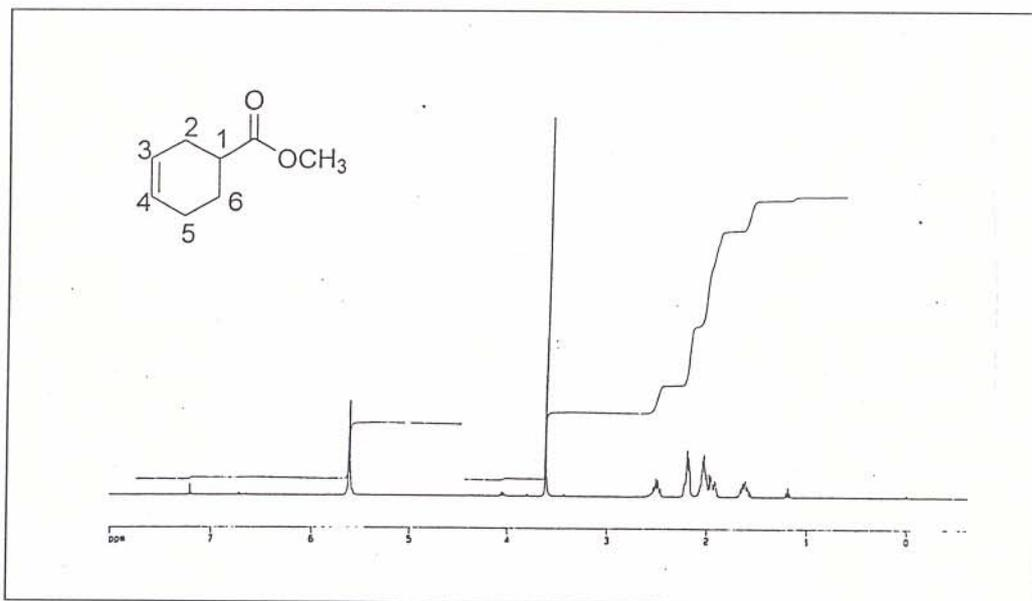
Figure 11. <sup>1</sup>H-NMR Spectrum of (±)-Methyl 3-Cyclohexene-1-carboxylate (30)
