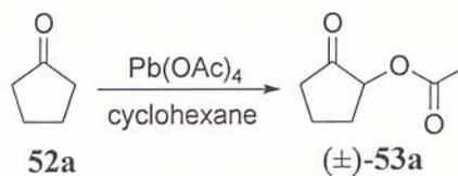
Scheme 33.  $\text{Pb}(\text{OAc})_4$  Oxidation of Cyclopentanone
