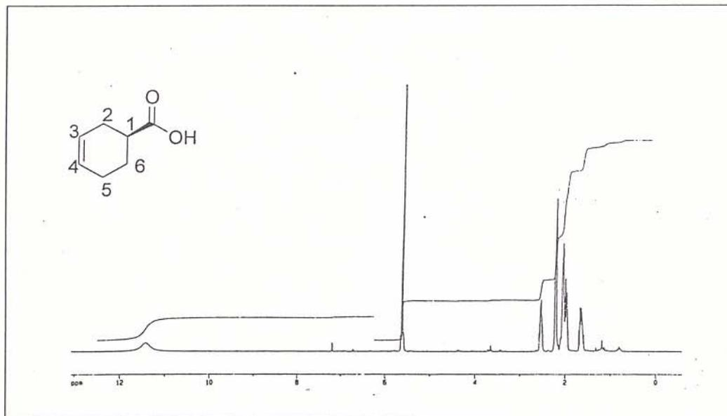
**Figure 13.** <sup>1</sup>H-NMR Spectrum of 3-Cyclohexene-1-carboxylic Acid (22)
