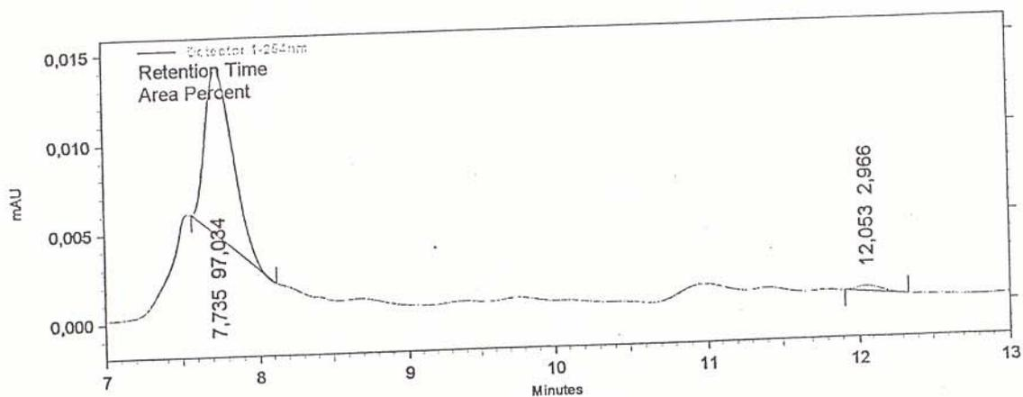
Figure 16. The HPLC-Chromatogram of (-)-22 from PLE Hydrolysis
