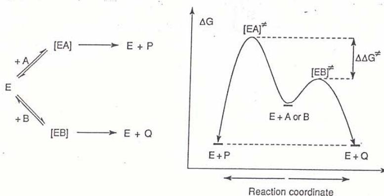
Figure 9. Energy Diagram for an Enzyme-Catalyzed Enantioselective Reaction
