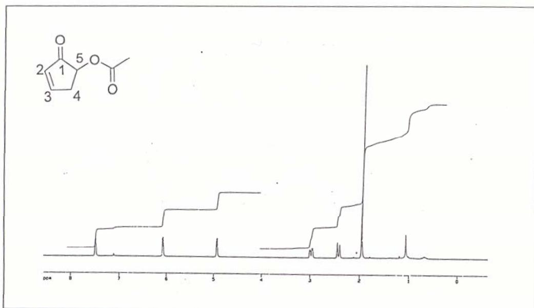
Figure 40. <sup>1</sup>H-NMR Spectrum of 5-Acetoxy-2-cyclopentenone (51a)
