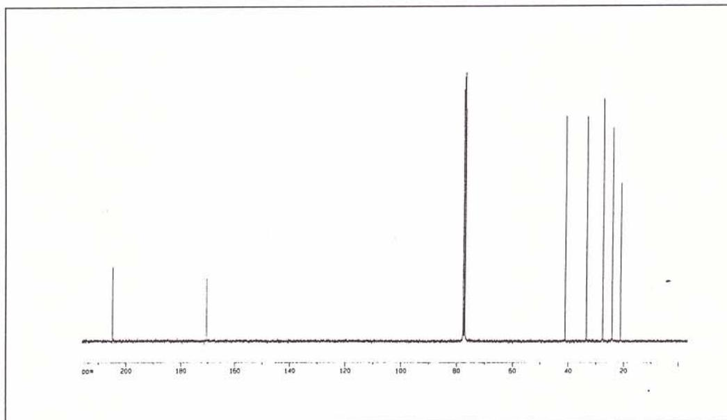
Figure 27. <sup>13</sup>C-NMR Spectrum of 2-Acetylcyclohexanone (53b)
