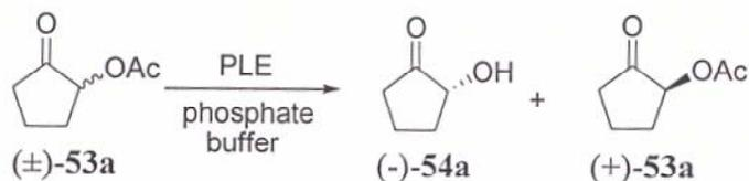
**Scheme 34.** Enzymatic Hydrolysis of ( $\pm$ )-**53a** with PLE
