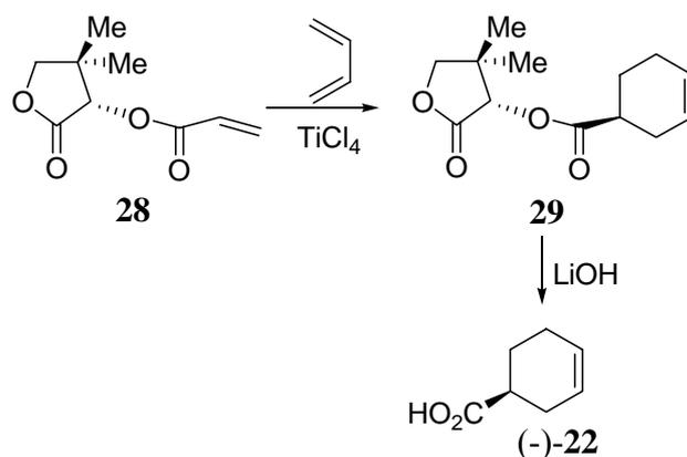
**Scheme 14.** TiCl<sub>4</sub>-Catalyzed Asymmetric Synthesis of (-)-**22**
