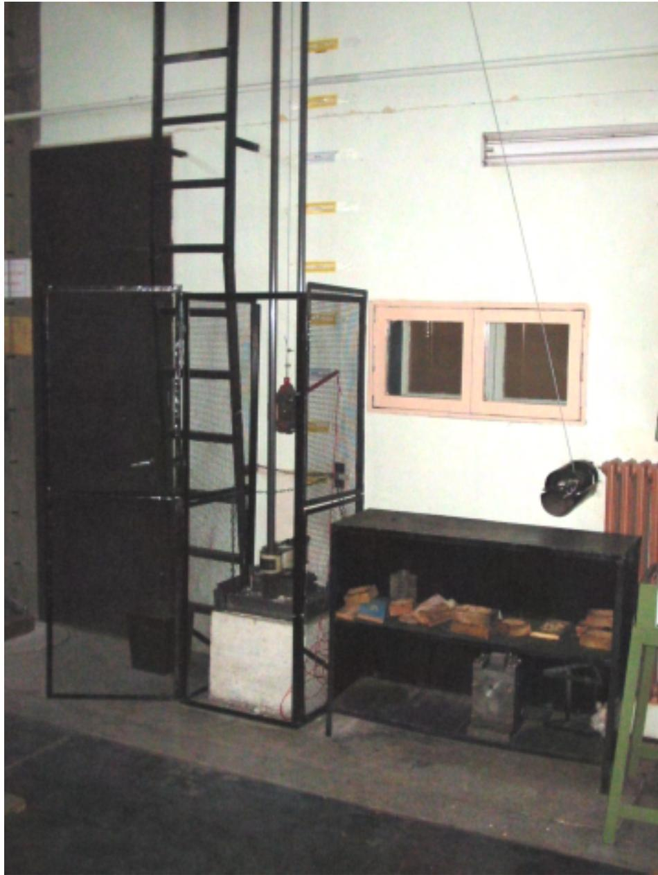
*Figure 3.1* Gravity drop weight testing machine [METU].
