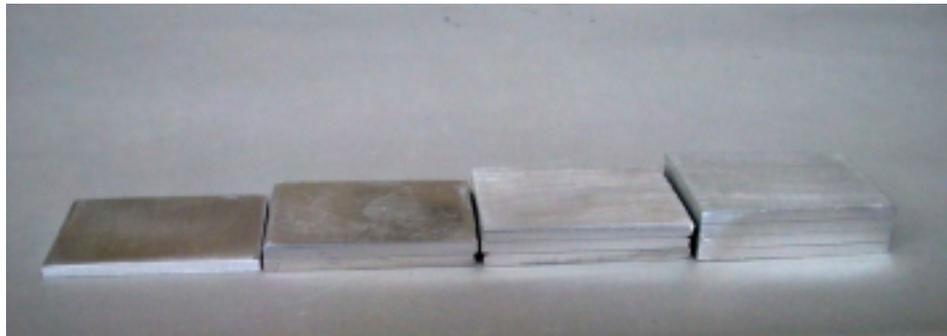
*Figure 3.7* AA 2024 plates bonded with epoxy adhesive.
