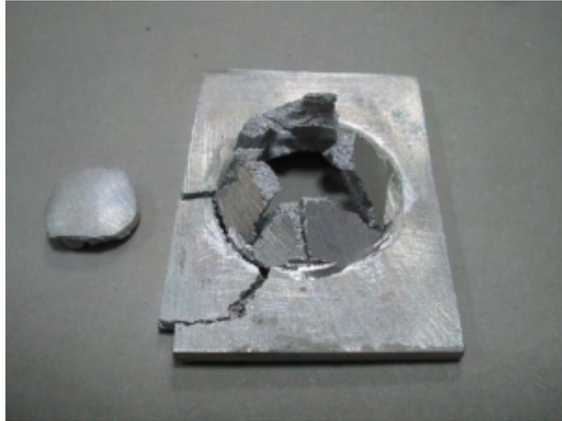
*Figure 5.6* AA 2024 target solution heat treated at 540°C impacted under drop-weight test machine
