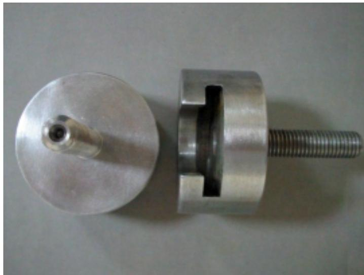
*Figure 3.15* Grips prepared for tensile testing of adhesives.
