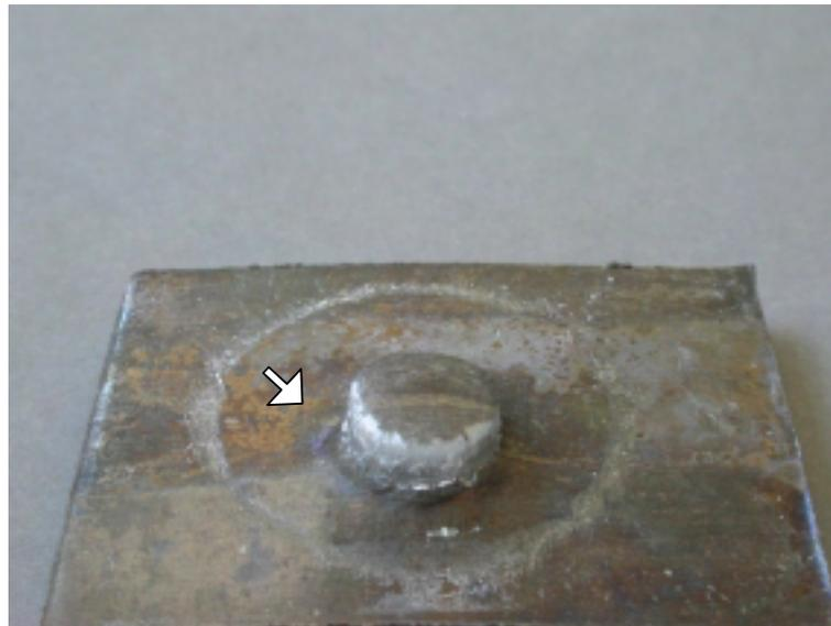
**Figure 4.27** Ballistic limit reached after an impact. The plug could not be separated.
