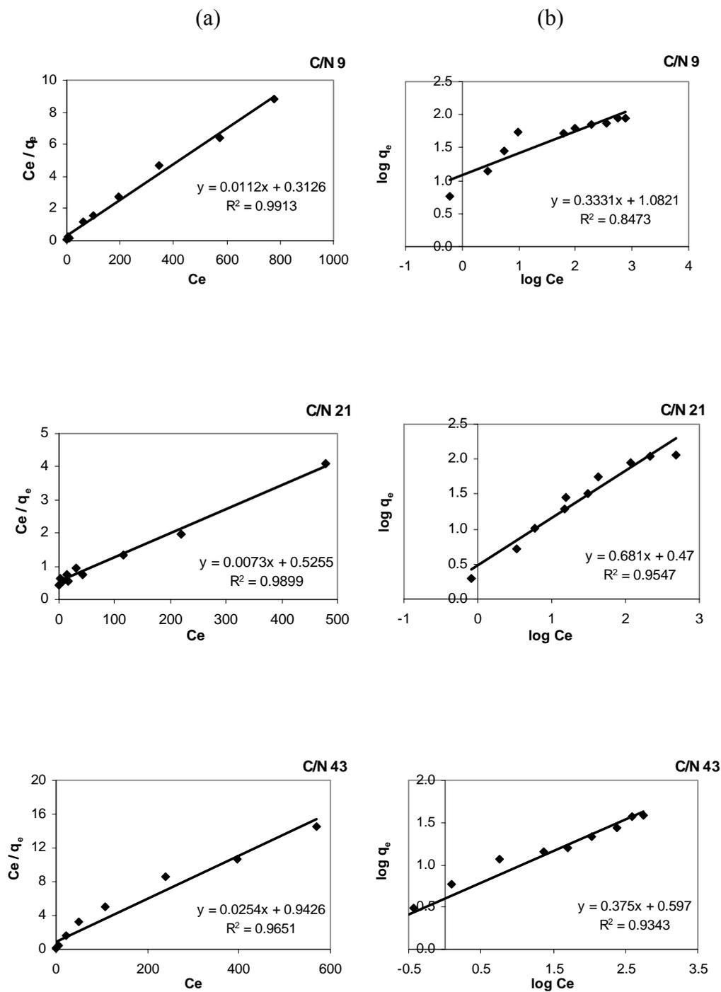
**Figure C.4.** Linearized a) Langmuir and b) Freundlich isotherms of zinc for C/N ratios 9, 21 and 43
