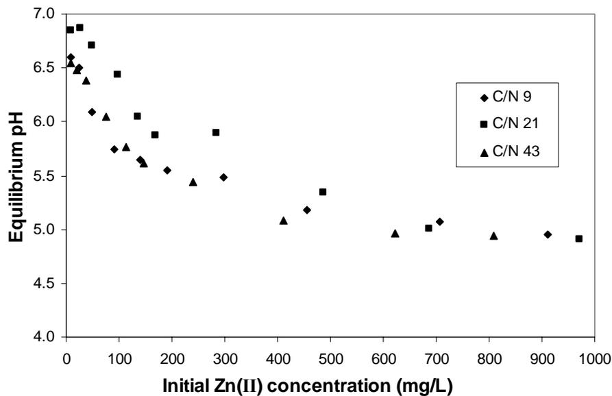
**Figure 4.26.** Effect of initial Zn(II) concentration on the equilibrium pH
