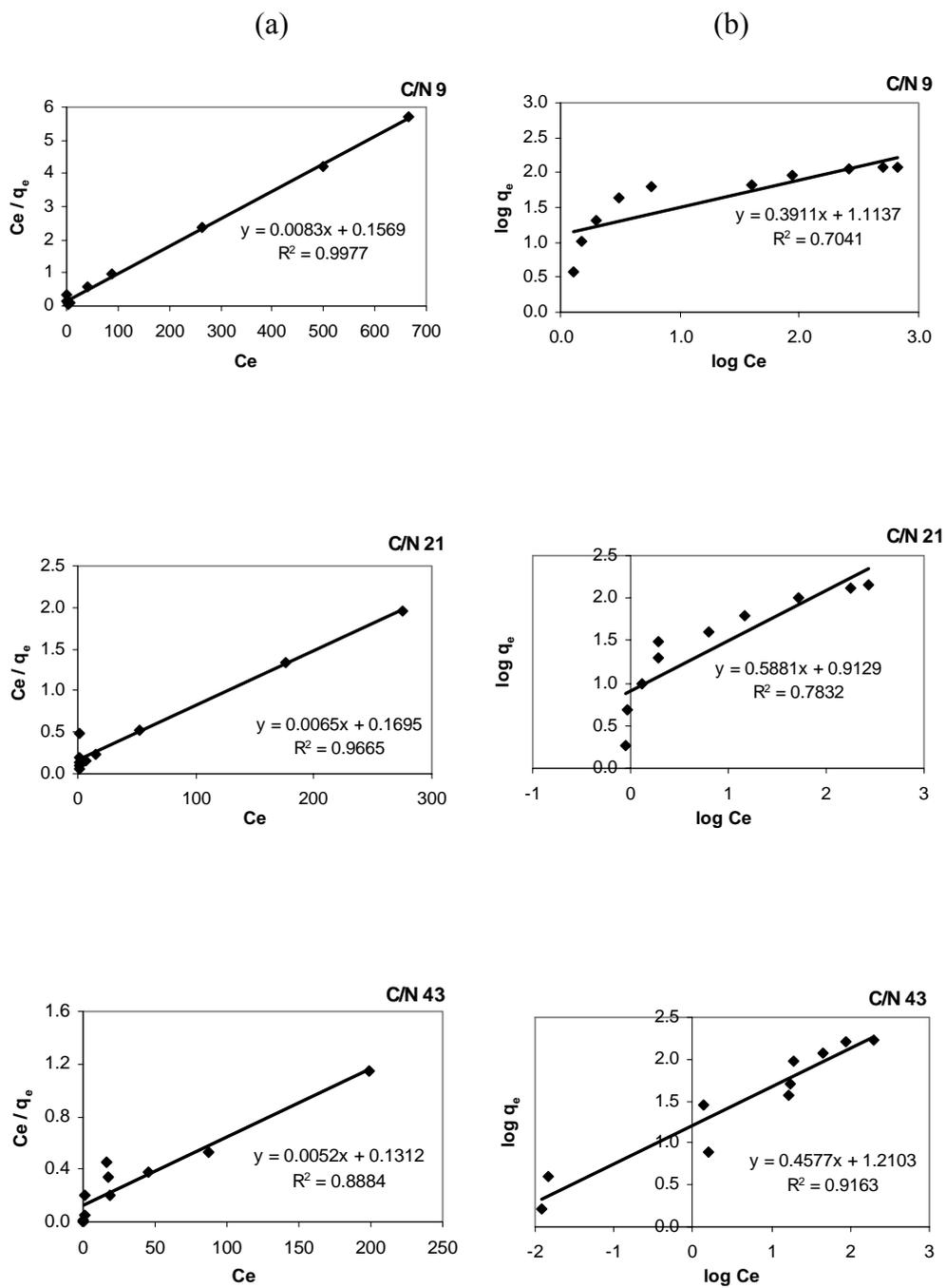
**Figure C.2.** Linearized a) Langmuir and b) Freundlich isotherms of cadmium for C/N ratios 9, 21 and 43
