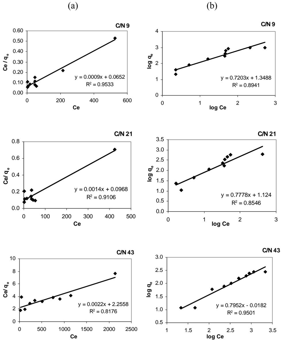
**Figure C.1.** Linearized a) Langmuir and b) Freundlich isotherms of lead for C/N ratios 9, 21 and 43
