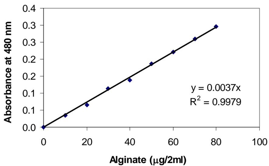
**Figure A 1.** Calibration curve for Dubois method
