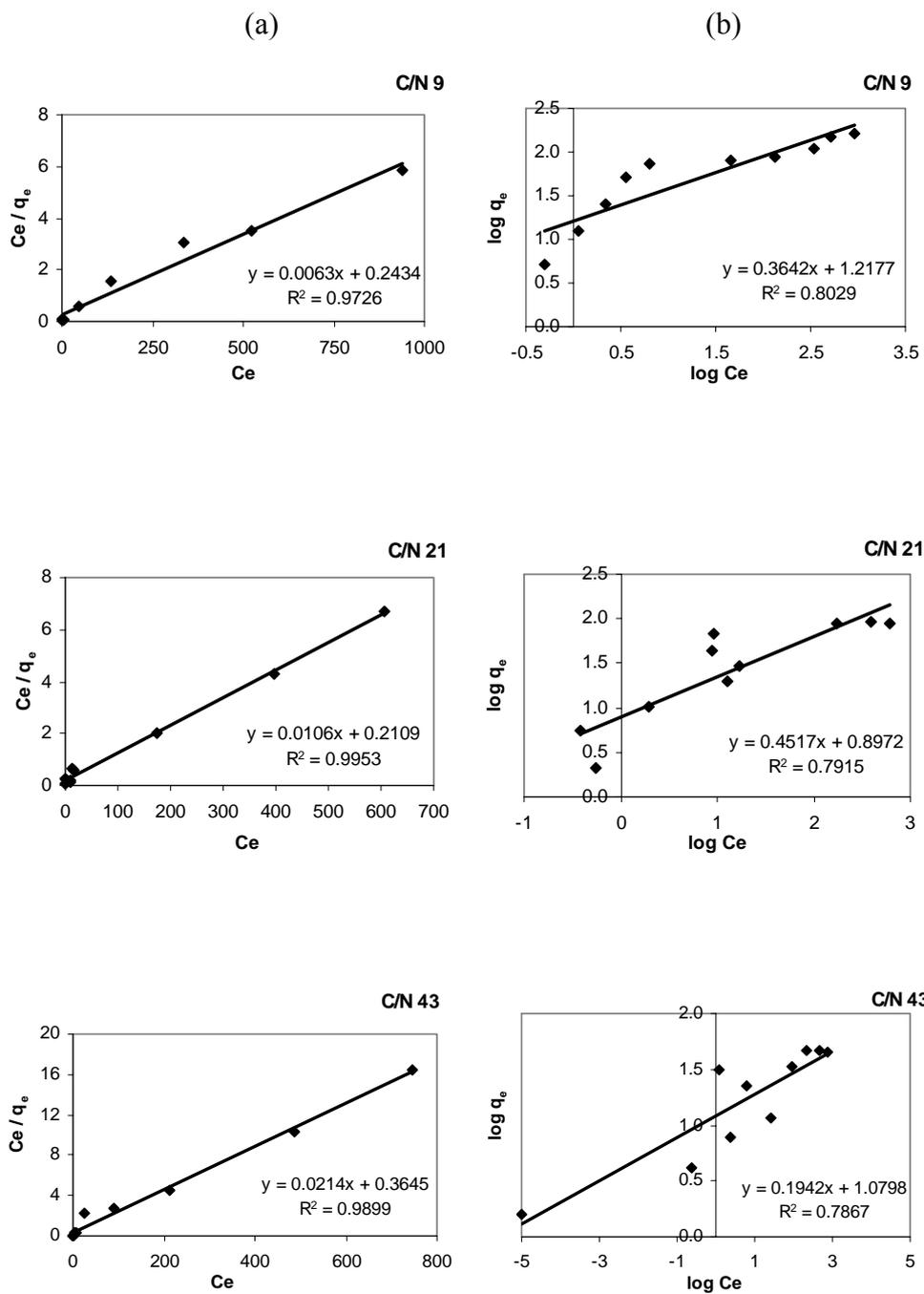
**Figure C.3.** Linearized a) Langmuir and b) Freundlich isotherms of copper for C/N ratios 9, 21 and 43
