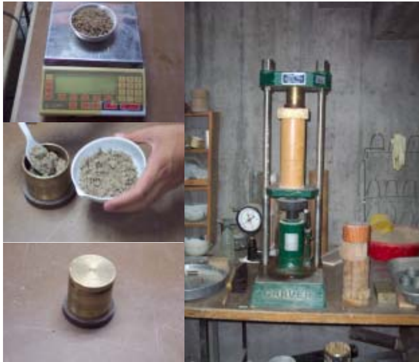
Figure 4.5 Placement of the sample into the Sampler Ring and the Compaction on the Hydraulic Jack
