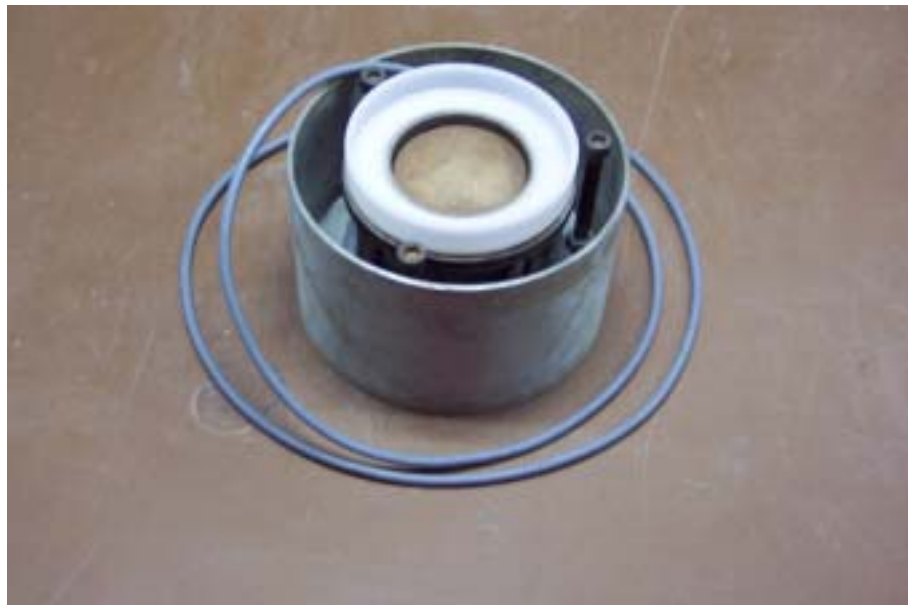
Figure 4.6 thin wall oedometer with placed sample and screwed into the inundation container.
