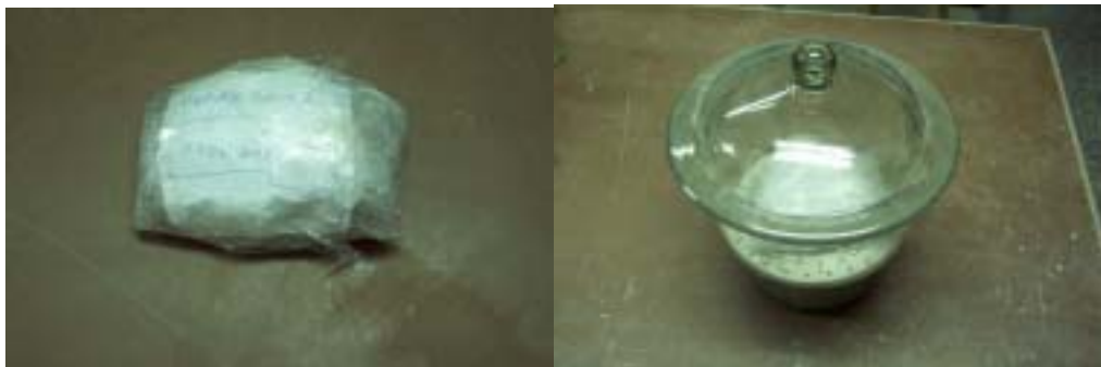
Figure 4.4 Soil Sample in Nylon Bag and in Dessicator
