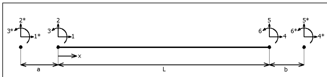
Figure 2.1 Frame element dimensions and DOF's
