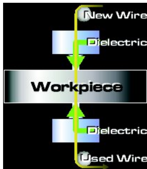
Figure 5.5 Diagram of the wire EDM process
