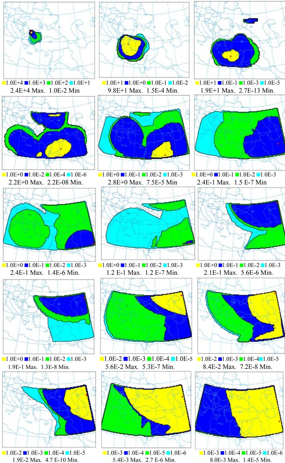
**Figure 4.13** Ground Level Activities of the Cs-137 and I-131 Isotopes for the Higher Release Rate- Concentration (Bq/m<sup>3</sup>) averaged between 0-10 m
