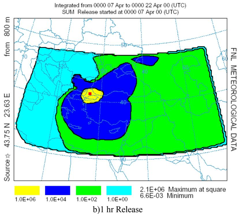
**Figure 4.10** Cumulative Deposition Patterns of the Cs-137 and I-131 Isotopes for the 1-hr and 6-hr Release Duration Cases
