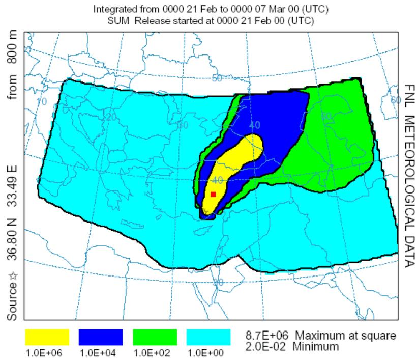
**Figure 4.6.** Cumulative Deposition Pattern of the Cs-137 and I-131 Isotopes for the
