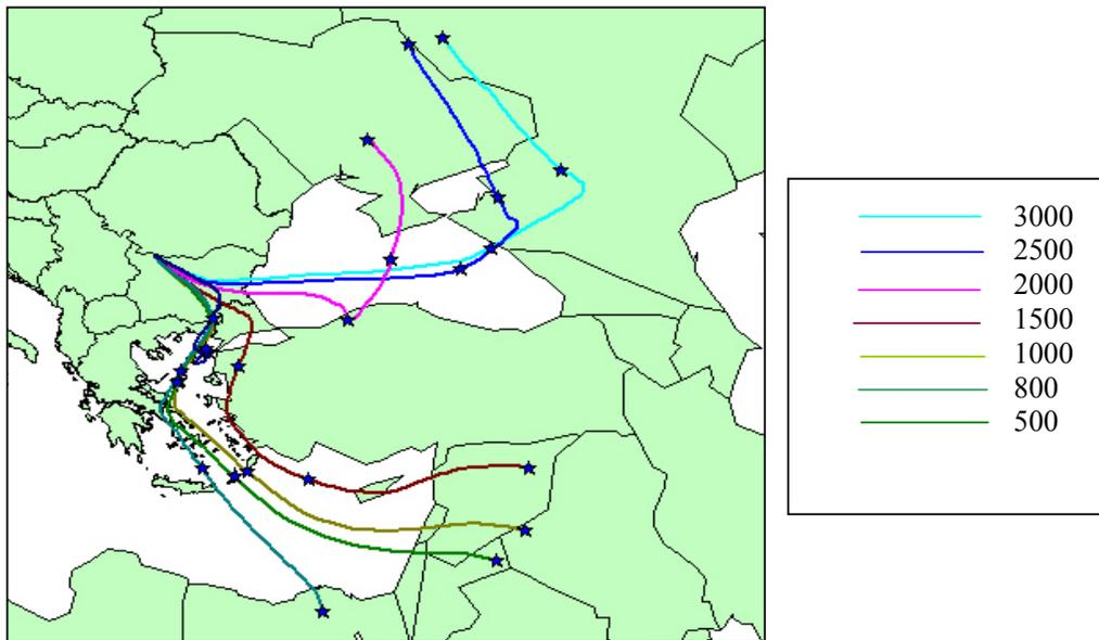
**Figure 4.3.** 314 and 72 hr-long forward trajectories starting at 500 m, 1000 m, 1500 m, 2000 m, 2500 m and 3000 m at the time of Kozloduy accident
