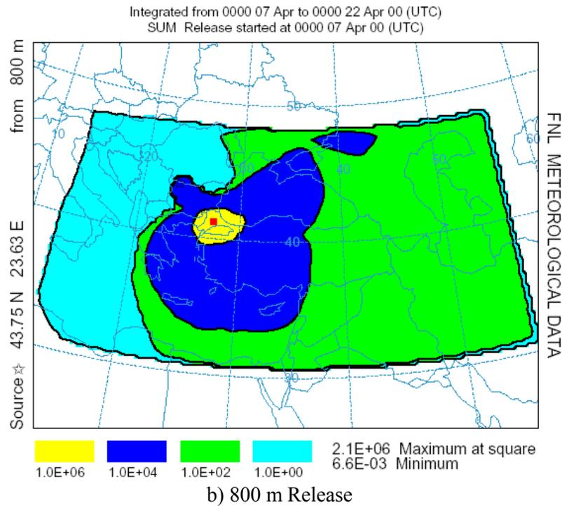
**Figure 4.8.** Cumulative Deposition Patterns of the Cs-137 and I-131 Isotopes for the 45 m and 800 m Release Heights
