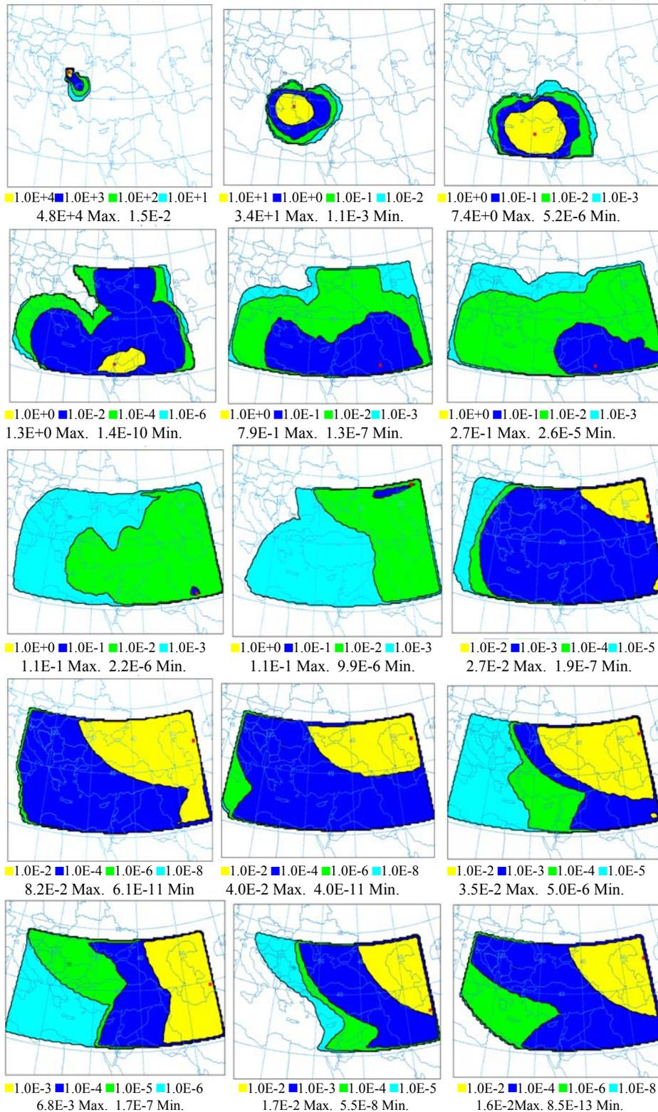
**Figure 4.9.** Ground Level Activities of the Cs-137 and I-131 Isotopes for the 45 m Release Height (7-22 April 2000) ( $\text{Bq}/\text{m}^3$ )
