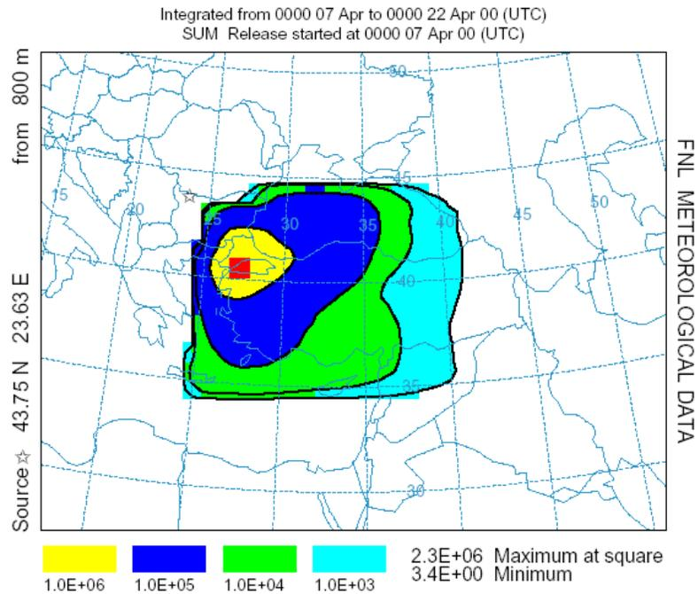
**Figure 4.14.** Cumulative Deposition Pattern for the 64 Isotopes for the Kozloduy
