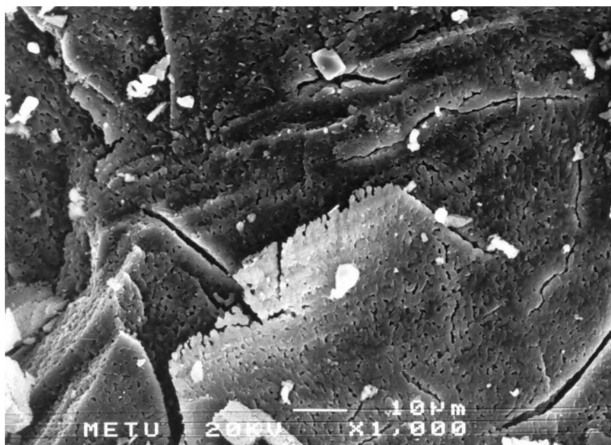
Figure 36a. SEM image of hand-picked trona samples calcined at 150 °C (bar = 10μm, magnification 1000x)
