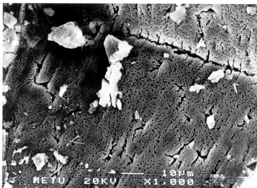
Figure 37a. SEM image of hand-picked trona samples calcined at 200 °C (bar = 10μm, magnification 1000x)
