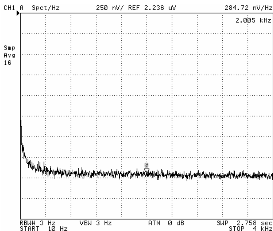
Figure 8.11: Total measured noise spectral density of the preamplifier from 10 Hz to 4 kHz using a transimpedance amplifier with 39.2 k \Omega feedback resistance.
