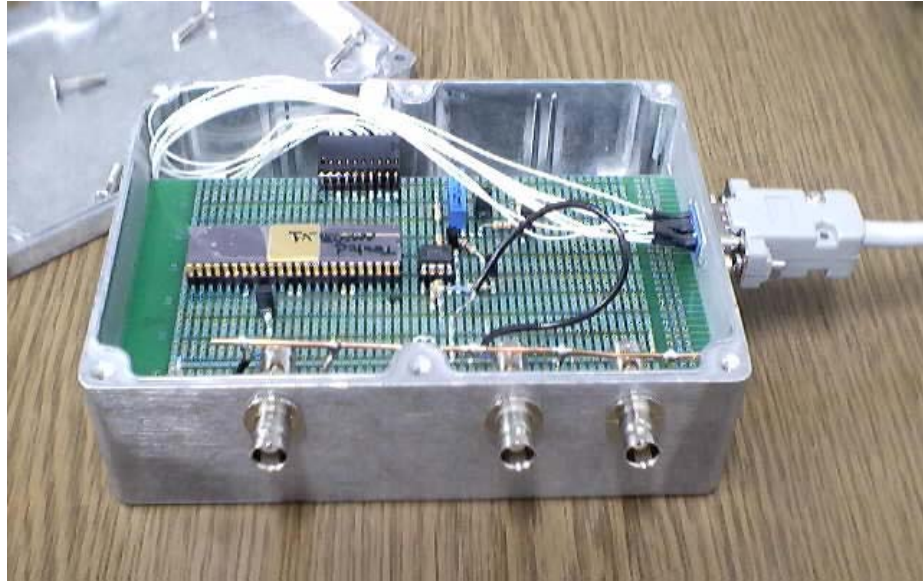
Figure 8.9: Prepared PCB and faraday cage for noise measurement. The test chip and all the required bias circuitry is on the PCB. The critical bias voltages are applied by a 1.5 V battery placed at the bottom of the PCB (not seen here). Output is taken via one of the BNC connectors, and power is applied by a 9-pin connector.
