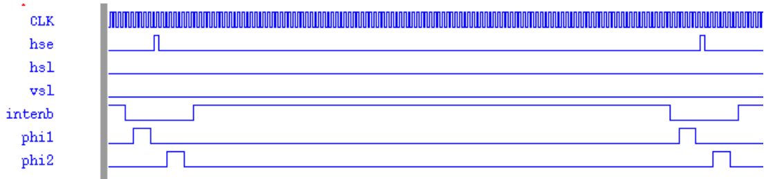
Figure 6.49: Verilog-XL simulation result showing the generation of the intenb , phi1 , and phi2 with respect to pixel select control signals such as hse , hsl , and vsl .
