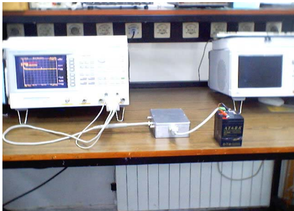
Figure 8.10: Noise measurement setup where the test circuit is placed in a faraday cage powered by an external battery.
