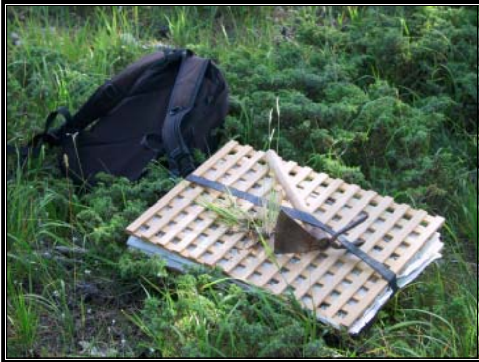
Figure 3.07. Standard plant press (in size 40.64x 25.4 cm or 16x10 inch)
