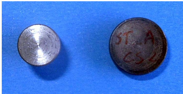
Figure 3.57 Circular shape of compressed standard compression test specimen of carbon steel
