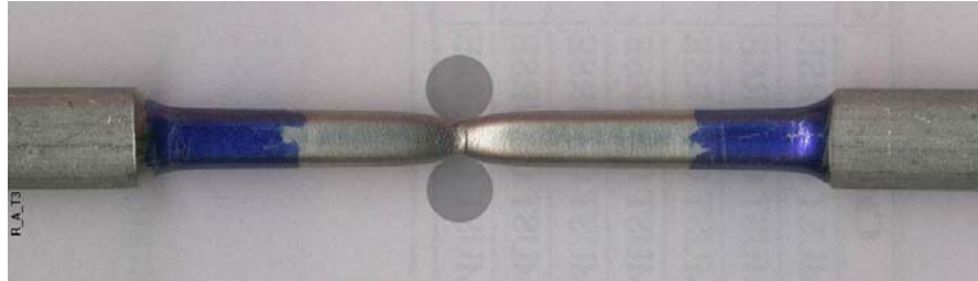
Figure 3.5 Photo of the failed tensile specimen with circles fit to the neck section.
