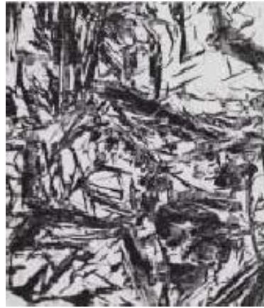
Figure 6.5 The microstructure of martensite body [7].
