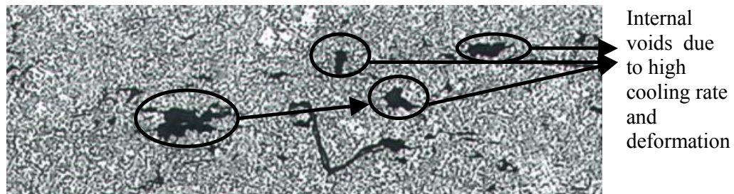
Figure 5.14 Internal defects occurred by excessive deformation (50X Microstructure film at the flange center)
