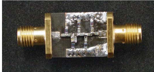
Figure 5.27: Top view of the second HP filter with elements and connectors soldered
