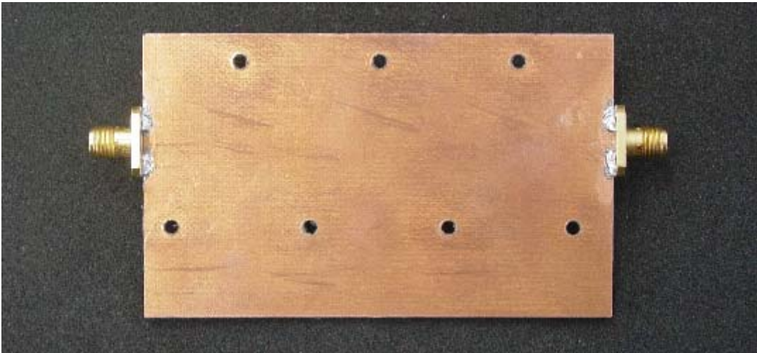
Figure 5.44: Connected view of Selected Lowpass Filter 1
