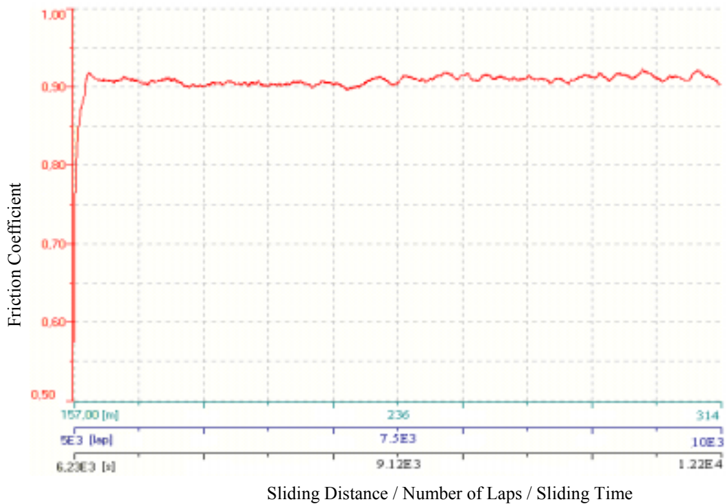
Figure 4.4 Variation of friction coefficient of the mica glass-ceramic studied as functions of number of laps, sliding distance, and sliding time. The applied load was 4N the sliding speed was 0.025 m/s and the environment was ambient. Data was obtained between;
