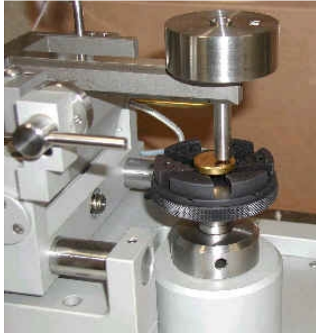
Figure 2.4 Pin on disc tribometer used in this study.
