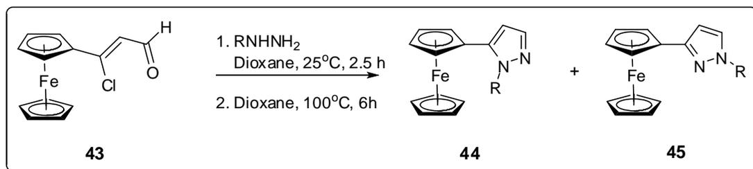
**Figure 21.** Synthesis of ferrocenyl pyrazoles by the reaction of (2-formyl-1-chlorovinyl)ferrocene (**43**) with hydrazines.
