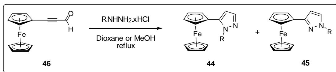
**Figure 22.** Synthesis of ferrocenyl pyrazoles by the reactions of 3-ferrocenylpropynal (**46**) with hydrazinium salts.
