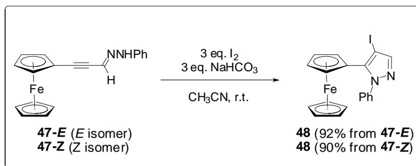
**Figure 32.** Synthesis of 5-ferrocenyl-4-iodo-1-phenyl-1*H*-pyrazole (**48**).
