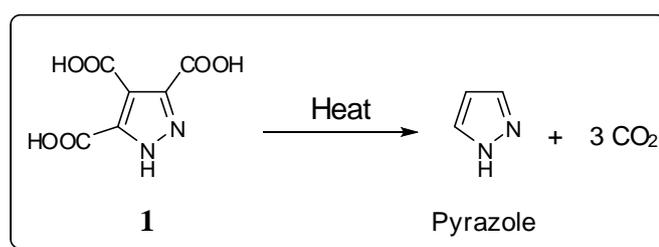
**Figure 3.** Decarboxylation of pyrazole-3,4,5-tricarboxylic acid (**1**) to pyrazole.
