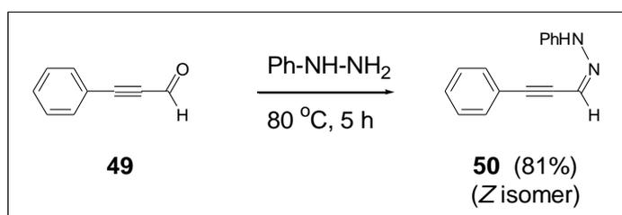
**Figure 38.** Synthesis of phenyl substituted hydrazone **50**.
