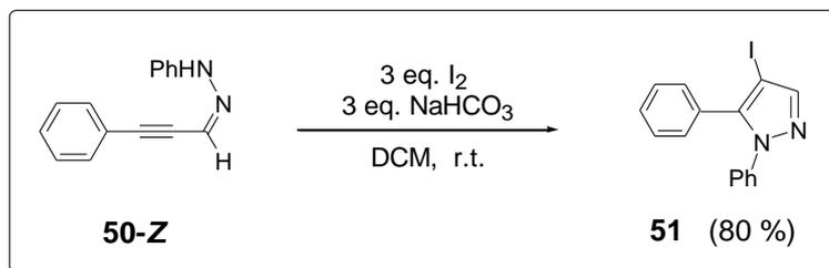
**Figure 39.** Synthesis of 4-iodo-1,5-diphenyl-1*H*-pyrazole (**51**).
