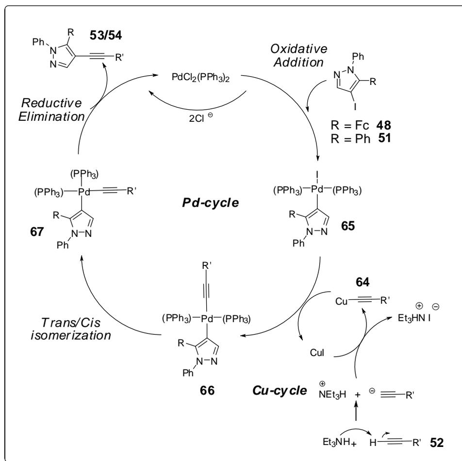
**Figure 47.** Mechanism of Sonogashira coupling reaction.
