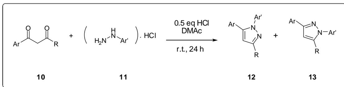
**Figure 8.** Synthesis of pyrazoles by the reaction of 1-arylbutane-1,3-diones **10** with arylhydrazine hydrochlorides **11**.
