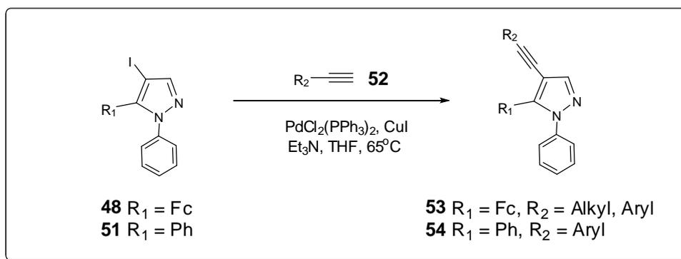
**Figure 27.** Synthesis of 4-alkynyl-5-ferrocenyl-1-phenyl-1*H*-pyrazoles (**53**) and 4-alkynyl-1,5-diphenyl-1*H*-pyrazoles (**54**).
