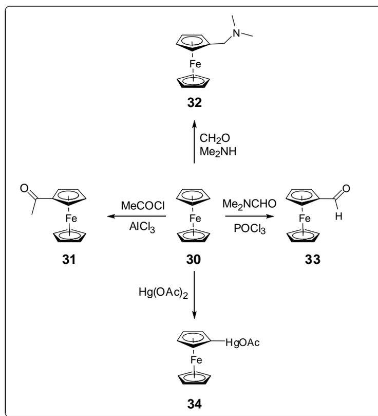
**Figure 17.** Typical substitution reactions of ferrocene (**30**).
