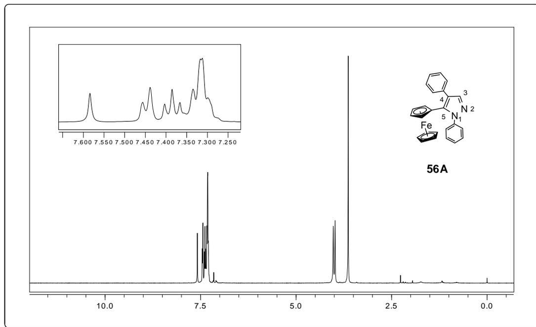
**Figure 44.** <sup>1</sup>H NMR spectrum of 5-ferrocenyl-1,4-diphenyl-1H-pyrazole (**56A**).
