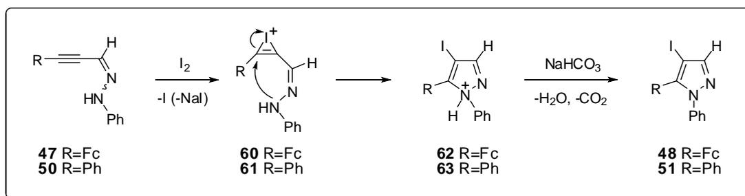
**Figure 46.** The mechanism for the formation of 4-iodo-5-ferrocenyl-1-phenyl-1*H*-pyrazole (**48**) and 4-iodo-1,5-diphenyl-1*H*-pyrazole (**51**).
