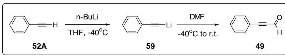
**Figure 37.** Synthesis of 3-phenylpropynal (**49**).
