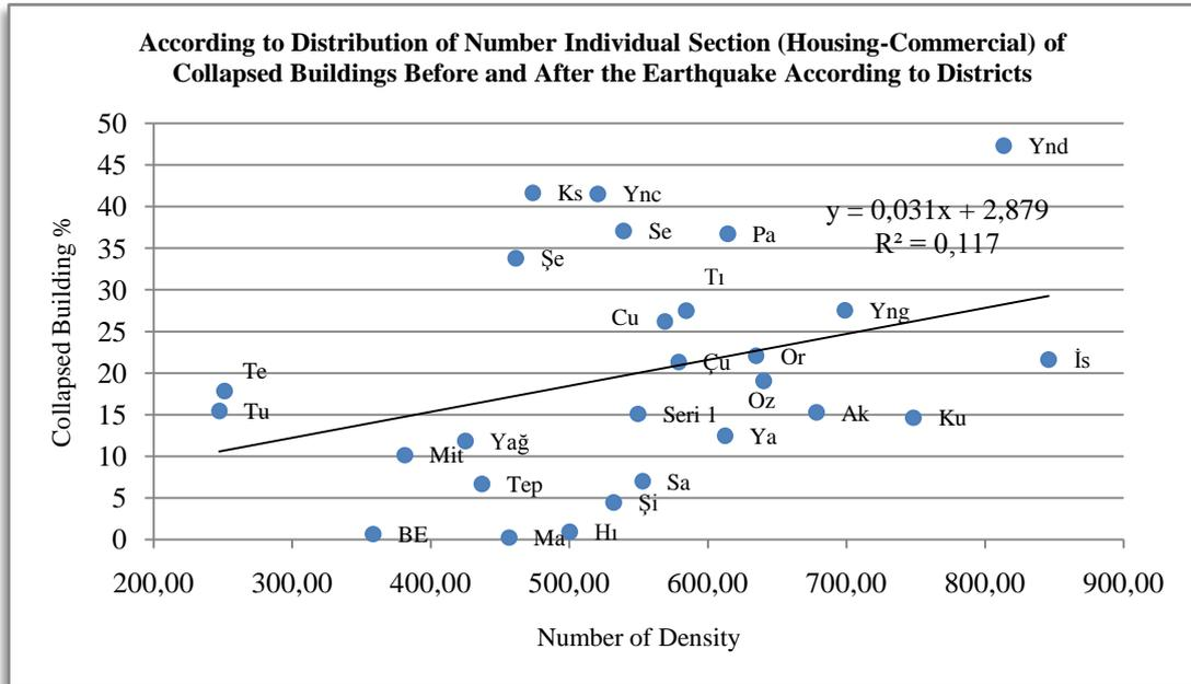
Figure 3.4 According to Distribution of Number Individual Section (Housing-Commercial) of Collapsed Buildings Before and After the Earthquake According to Districts
