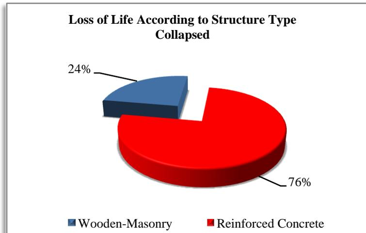
Figure 5.19 Loss of Life According to Structure Type Collapsed
