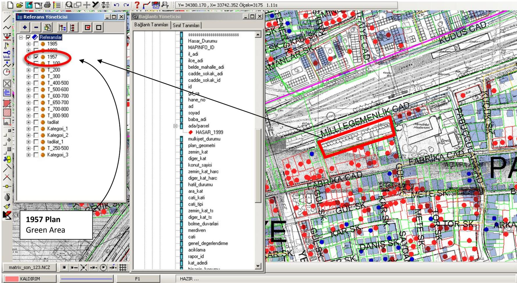
Figure A.6 An Example Of Database interrogation (GIS) for Collapsed Buildings
