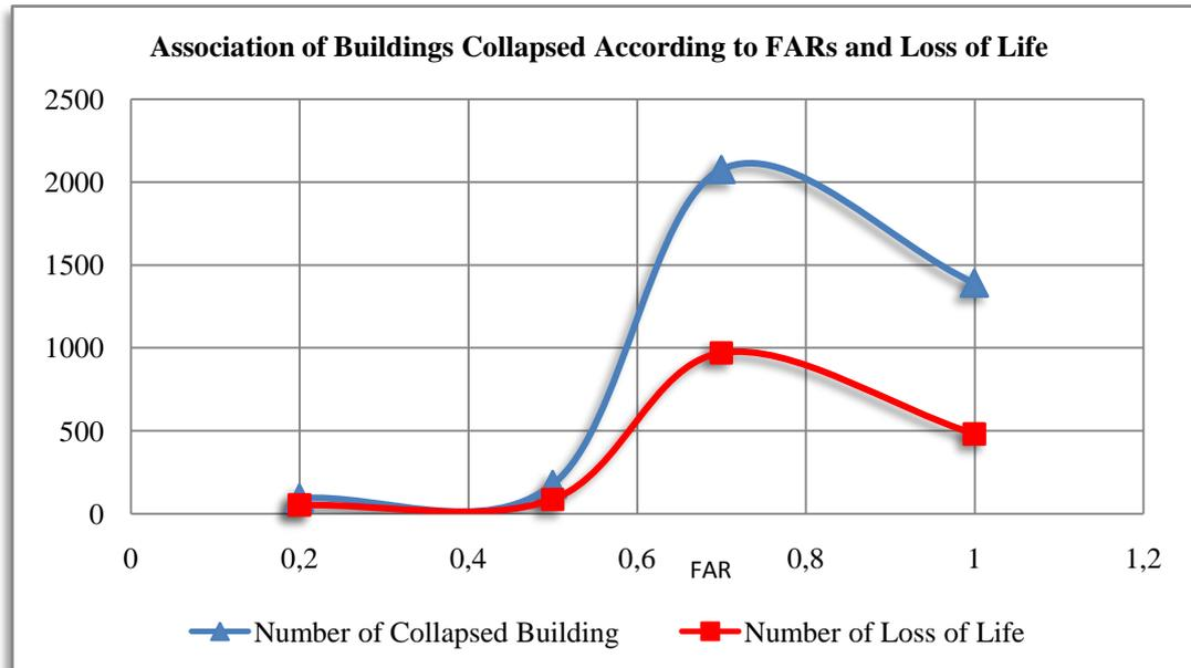
Figure 5.32 Association of Buildings Collapsed According to FARs and Loss of Life
