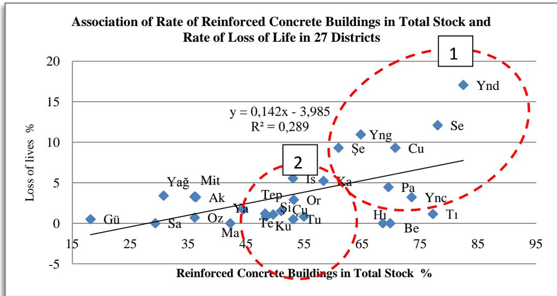
Figure 5.20 Association of Rate of Reinforced Concrete Buildings in Total Stock and Rate of Loss of Life in 27 Districts
