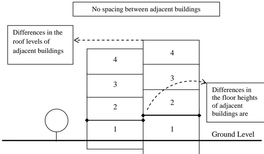
Figure 5.25 Hammering Impacts of Adjacent Buildings in the Earthquake
