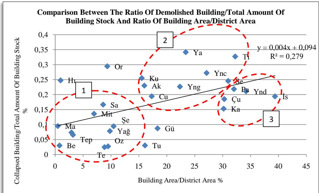
Figure 5.17 Comparison Between The Ratio Of Collapsed Building/Total Amount Of Building Stock And Ratio Of Building Area/District Area
