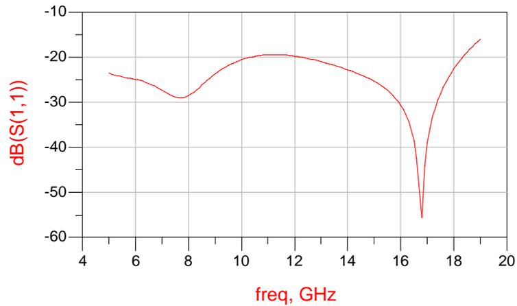
**Figure 4.111** S11 of 6-18 GHz power divider.
