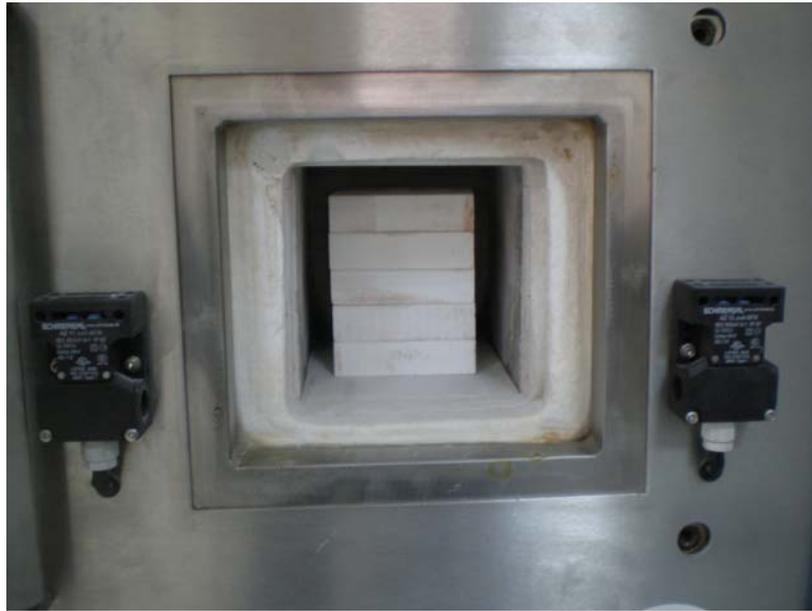
**Figure 3.4** Picture of home-built “insulation cage” placed within the heating chamber of the microwave sintering furnace.
