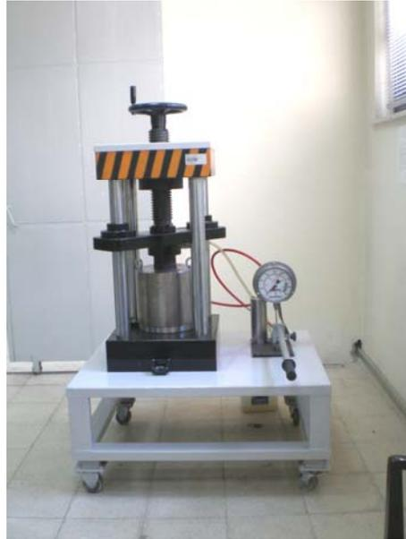
**Figure 3.5** The pictures of home-designed and custom-built Cold Isostatic Press
