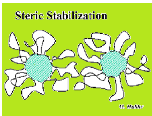
Figure 8. Schematic representation of steric stabilization of metal nanoparticles.
