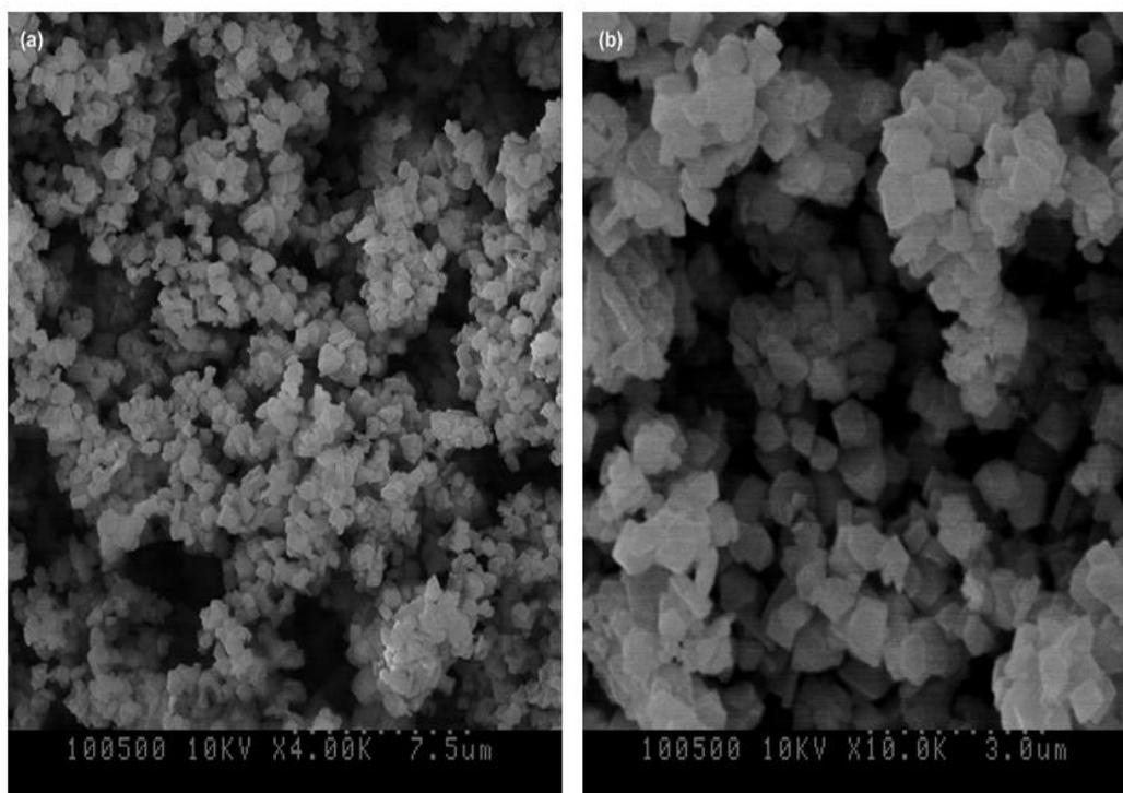
**Figure 4.2.** The scanning electron microscopy (SEM) images of zeolite confined rhodium(0) nanoclusters with a 0.5 % wt Rh loading (after dehydration process) in different magnifications. Scale bar (a) 7.5  $\mu\text{m}$ , (b) 3.0  $\mu\text{m}$
