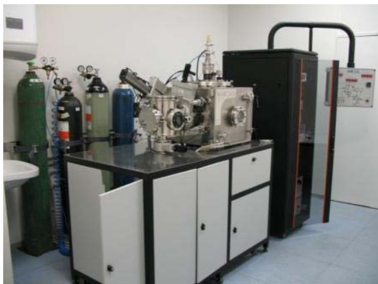
*Figure 2.2 Photograph of Nano-D100 sputtering system.*
