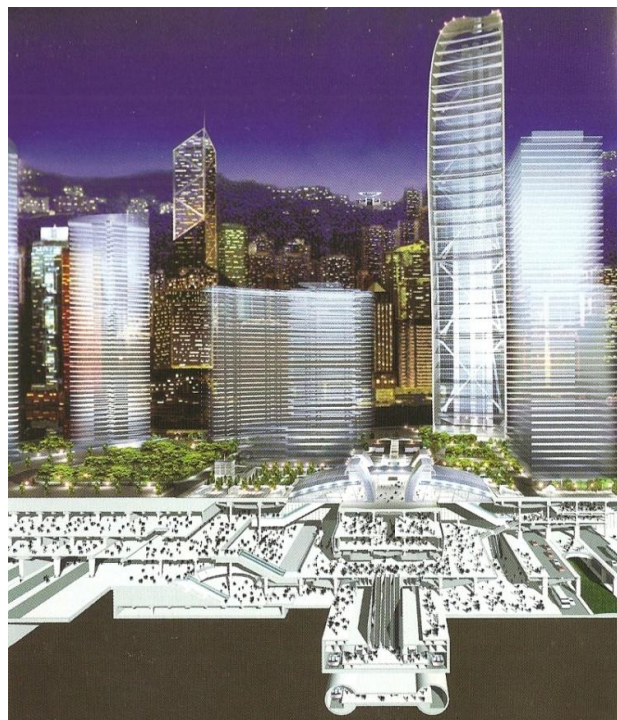
Figure 4.21 A section perspective drawing showing the sub-surface mobility layers and the urban park at the street level in the Kowloon Station. (Source: Martha Thorne. Ed. Modern trains and Splendid Stations . Chicago: Merrell-The Art Institute of Chicago, 2001. pg 68)
