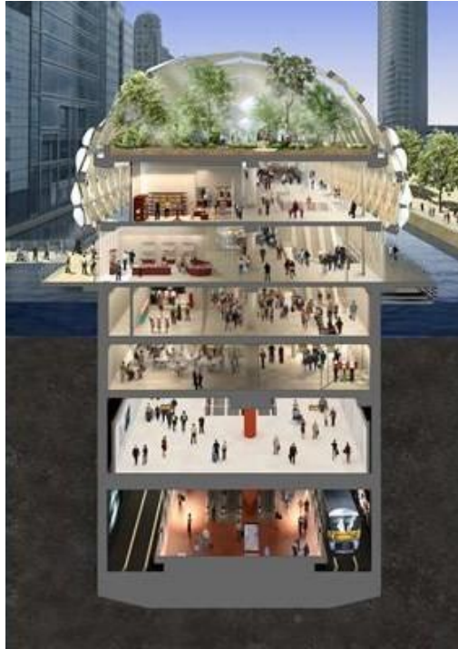
Figure 4.20 The section showing the sub-surface mobility layers and the proposed urban park above the Canary Wharf – Crossrail Line Station (Source: www.nce.co.uk . Last accessed on 09.03.2010)
