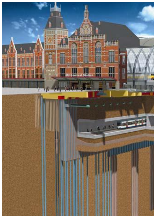
Figure 4.27 The section showing the superposition of the former and new transportation layers in IJ Hall
