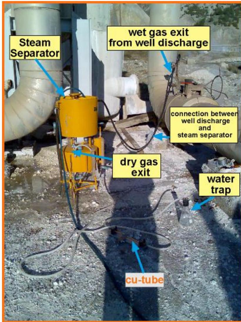
Figure 5.16 Gas sampling from wells in Kızıldere via steam separation.
