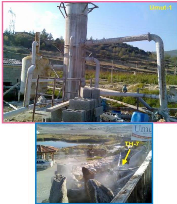
Figure 5.8 Drilling well (Umut-1) and well discharge through pipe (TH-7) in the Tekke Hamam geothermal field.
