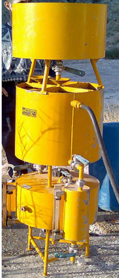
Figure 5.15 Steam Separator used in the Kizildere geothermal field.
