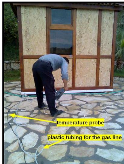
Figure 5.5 Sealing of the gas tube and the temperature probe.
