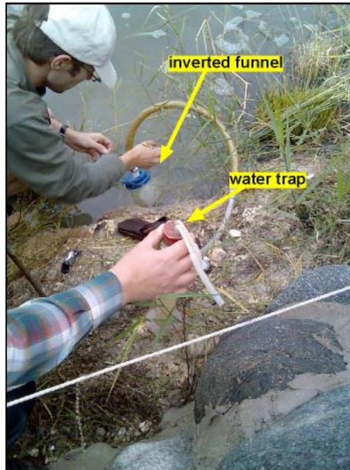
Figure 5.2 Insertion of the inverted funnel and checking the gas flow with a water trap.
