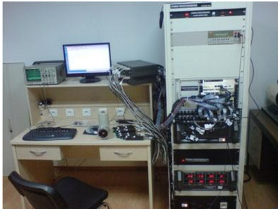
Figure 4.21 The setup for characterizing dual-band three-contact FPA
