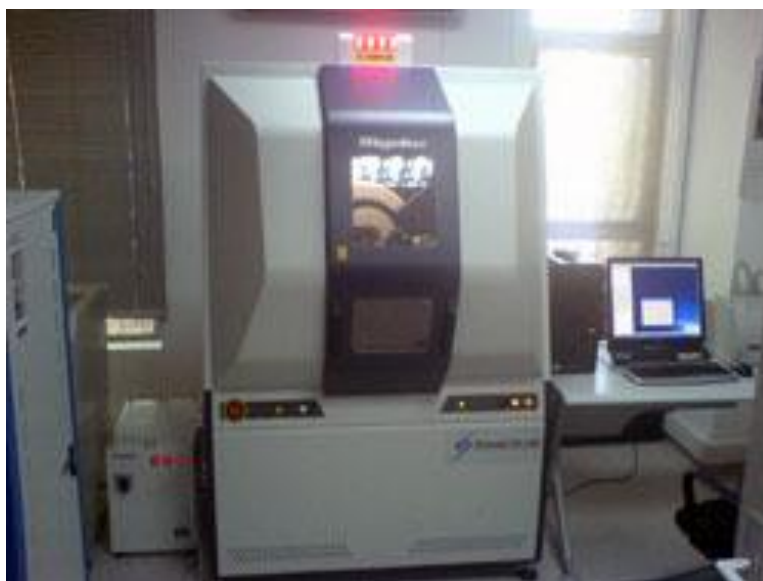
Figure 3.5 Photograph of the Rigaku HR-XRD system
