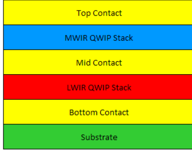
Figure 4.1 General structure of MWIR/LWIR dual band QWIP
