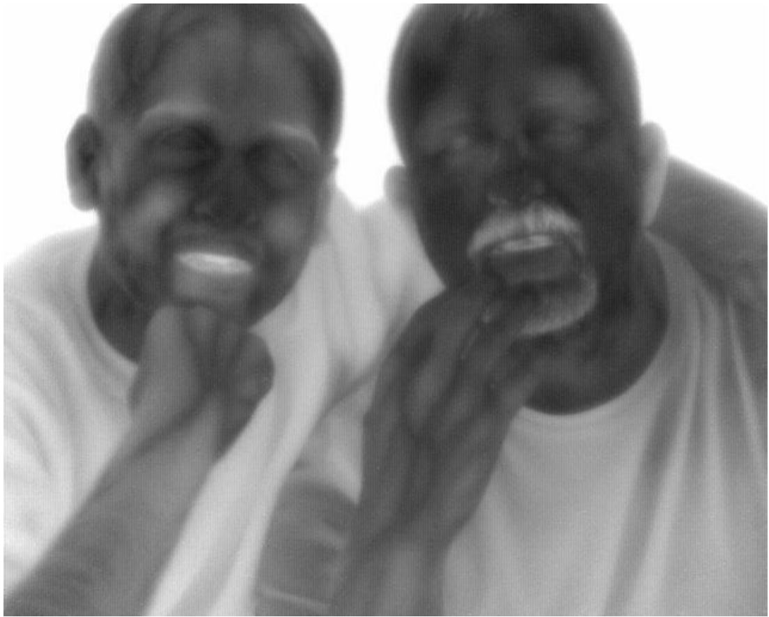
Figure 3.13 An indoor thermal image recorded with AlInAs/InGaAs QWIP FPA [67]
